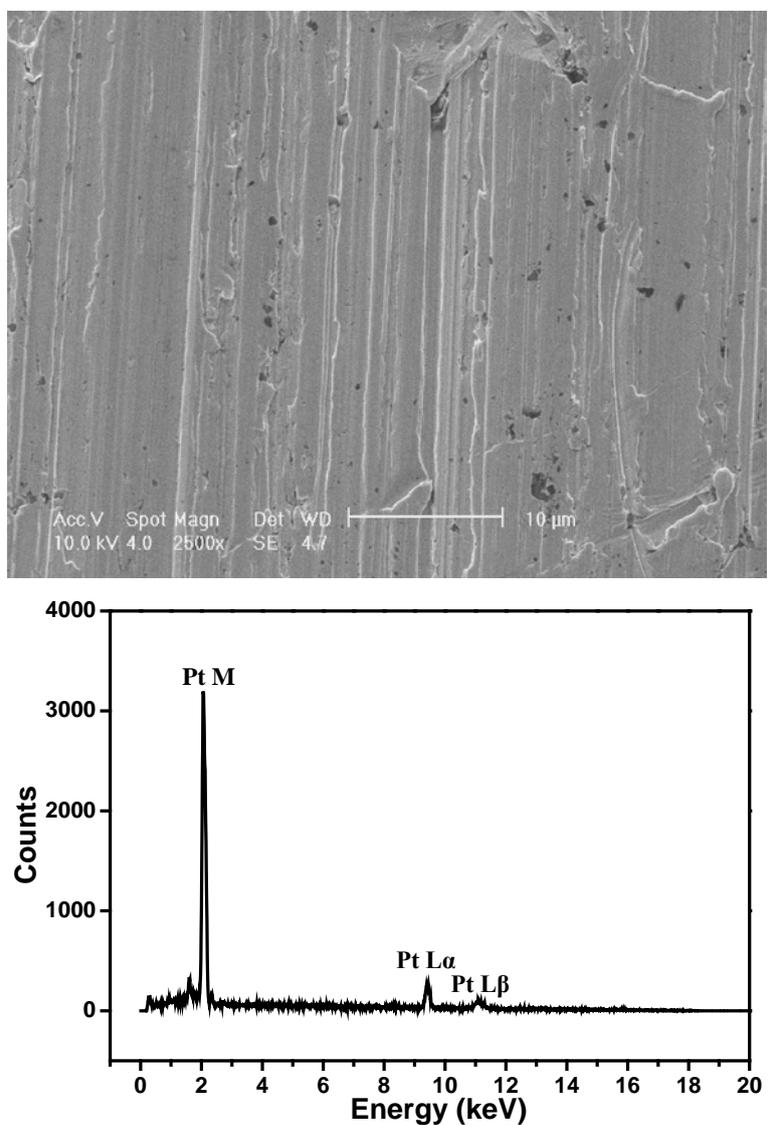
**Figure S1.** SEM image (top) and the corresponding EDS spectra (bottom) of the commercial Pt wire.
