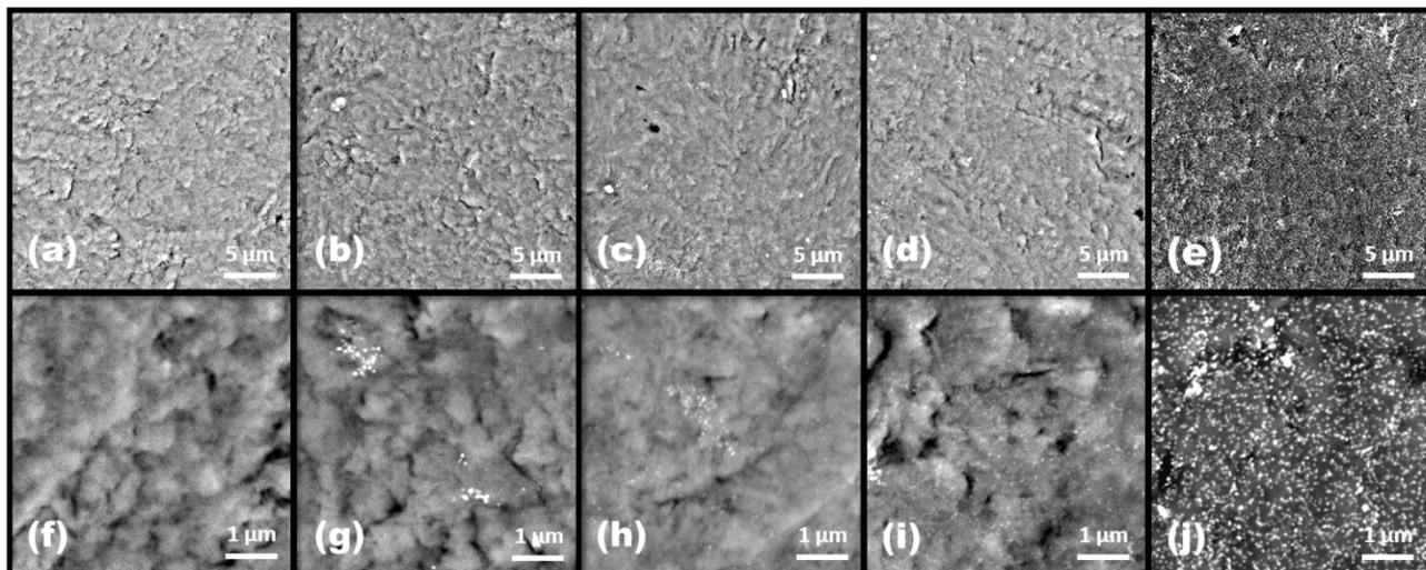
**Figure S5.** SEM images of the graphite electrode surface after different CV cycles when using a Pt wire as counter electrode. (a, f) 0 cycle, (b, g) 4000 cycles, (c, h) 8000 cycles, (d, i) 10000 cycles, (e, j) 12000 cycles, respectively.
