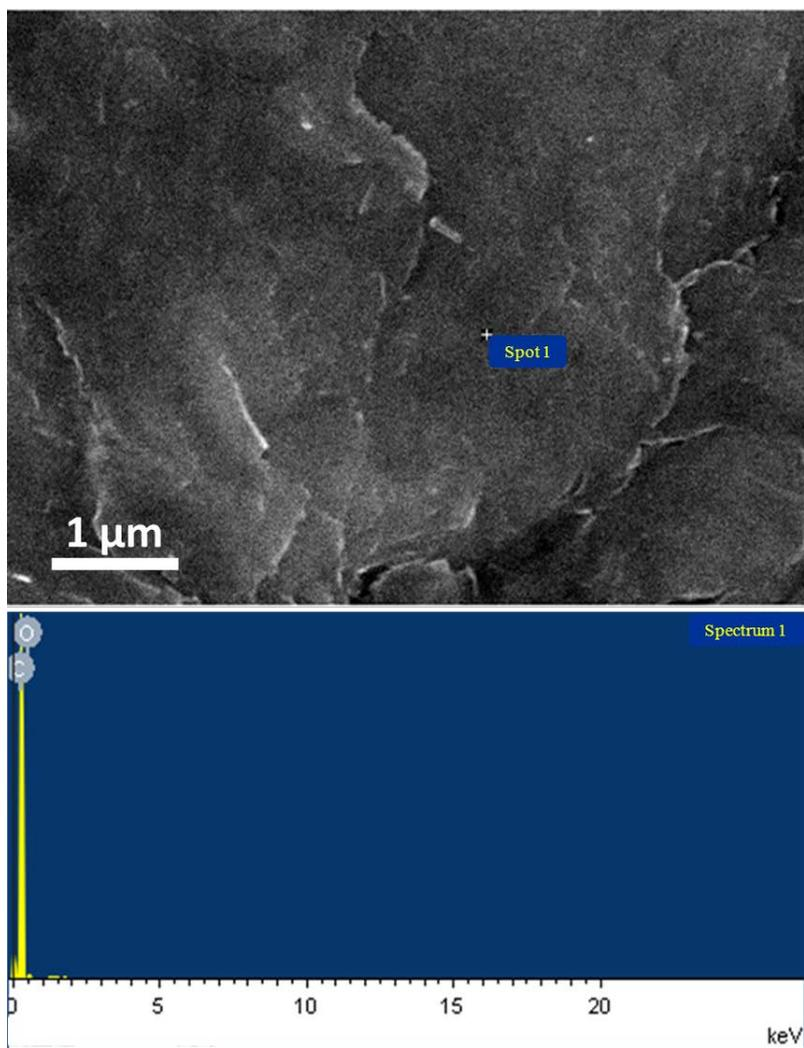
**Figure S2.** SEM image (top) and the corresponding EDS spectra (bottom) of the initial graphite electrode surface.
