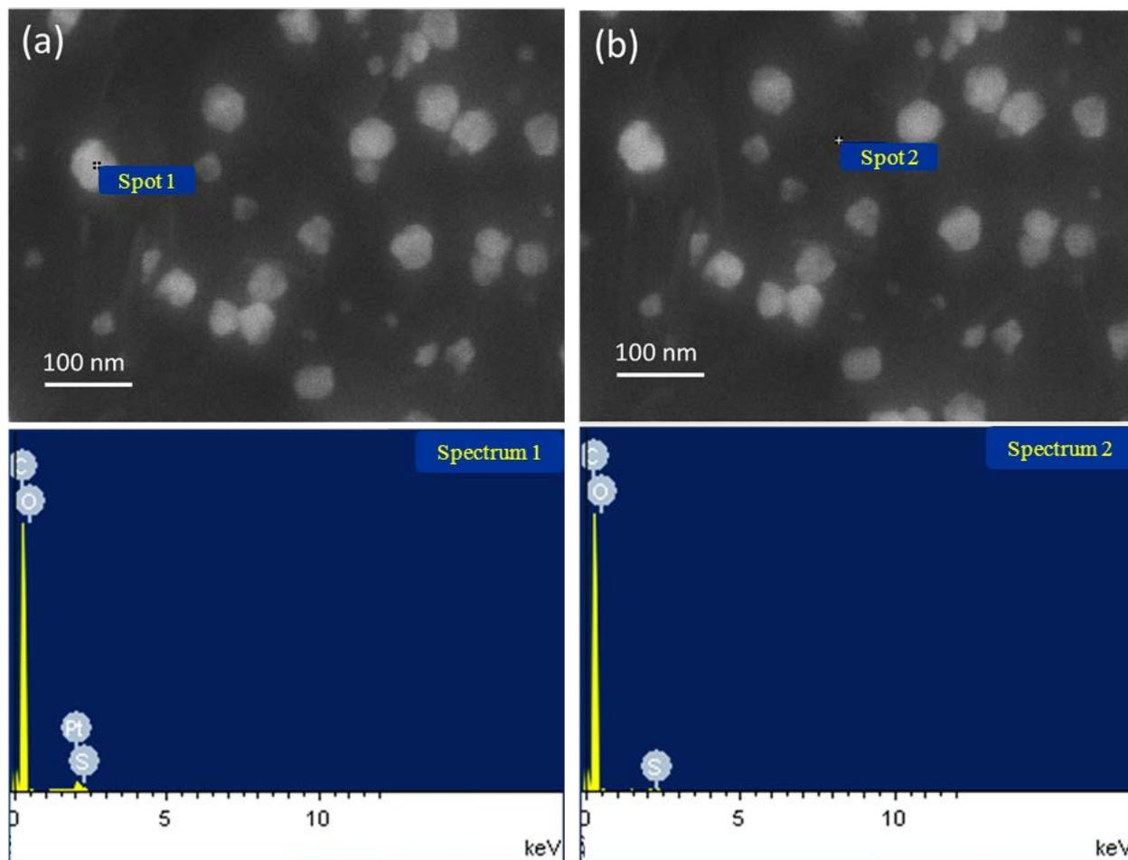
**Figure S3.** EDS spectra collected on different surface location of Pt-GE activated with Pt wire as the counter electrode, (a) on nanoparticle; (b) on the graphite layer.
