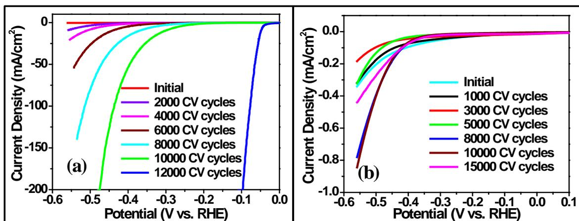
**Figure S4.** LSV curves on HER of graphite electrodes after different cycles of activation when using Pt wire (a) or graphite rod (b) as counter electrode, respectively.
