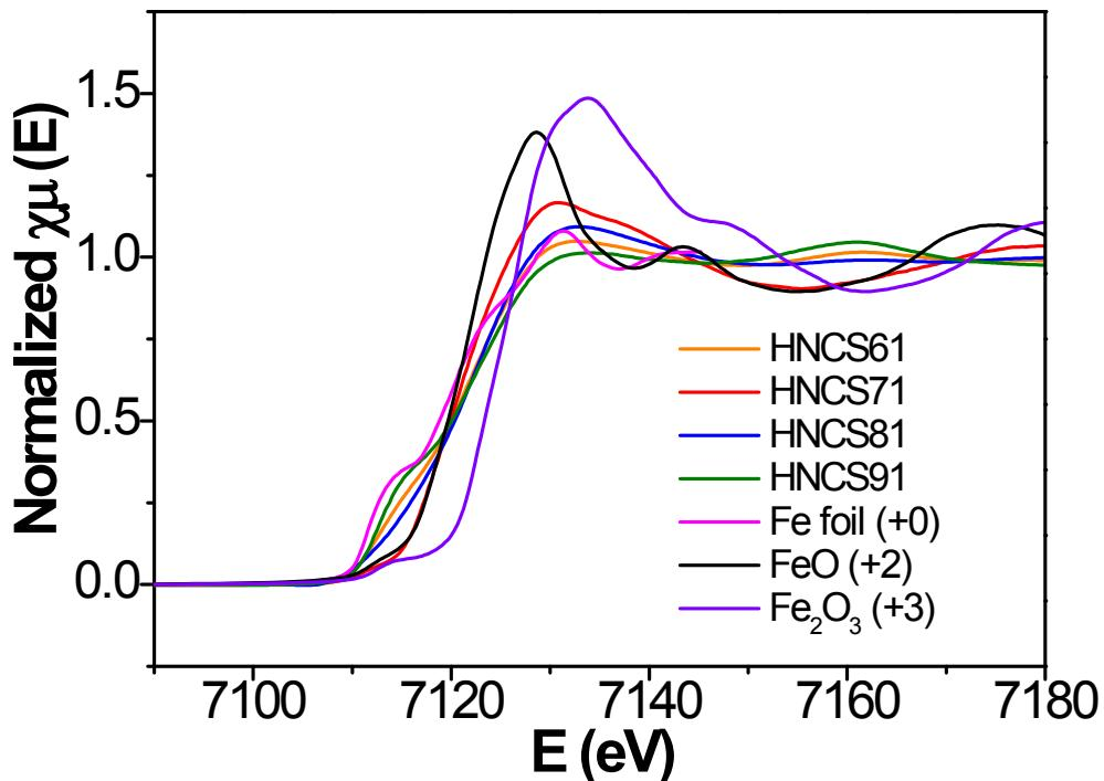
**Figure S6.** Fe K-edge XANES spectra of HNCS electrocatalyst with standard Fe foil, FeO and Fe<sub>2</sub>O<sub>3</sub>
