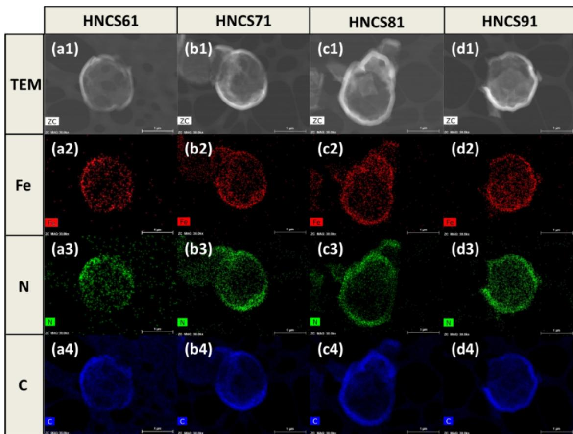
**Figure S2.** Arrays showing the bright field STEM image, individual of element the Fe-K edge, N-K edge and C-K edge image of catalyst Vs. HNCS61, HNCS71, HNCS81, and HNCS91.
