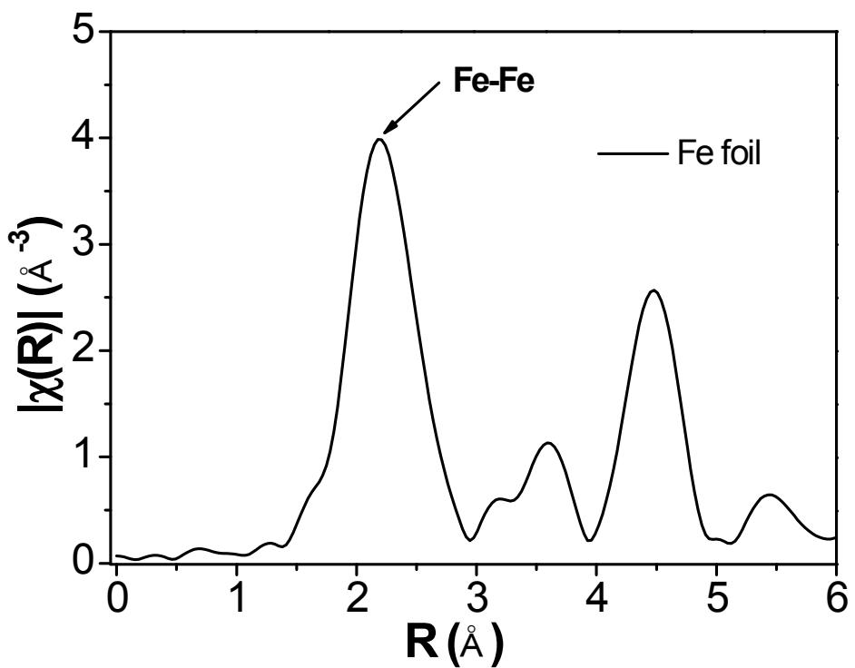
**Figure S7.** Fe K-edge of k<sup>2</sup>-weighted Fourier transforms EXAFS spectra of standard Fe foil.
