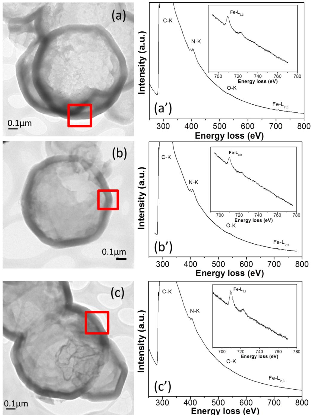
**Figure S1.** STEM image and EELS spectrum (red square indicated in STEM images) of (a, a') HNCS61, (b, b') HNCS81, (c, c') HNCS91, respectively.
