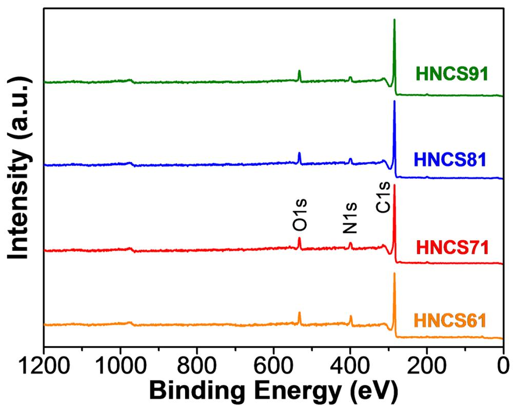
**Figure S3.** XPS survey spectra of HNCS catalyst.
