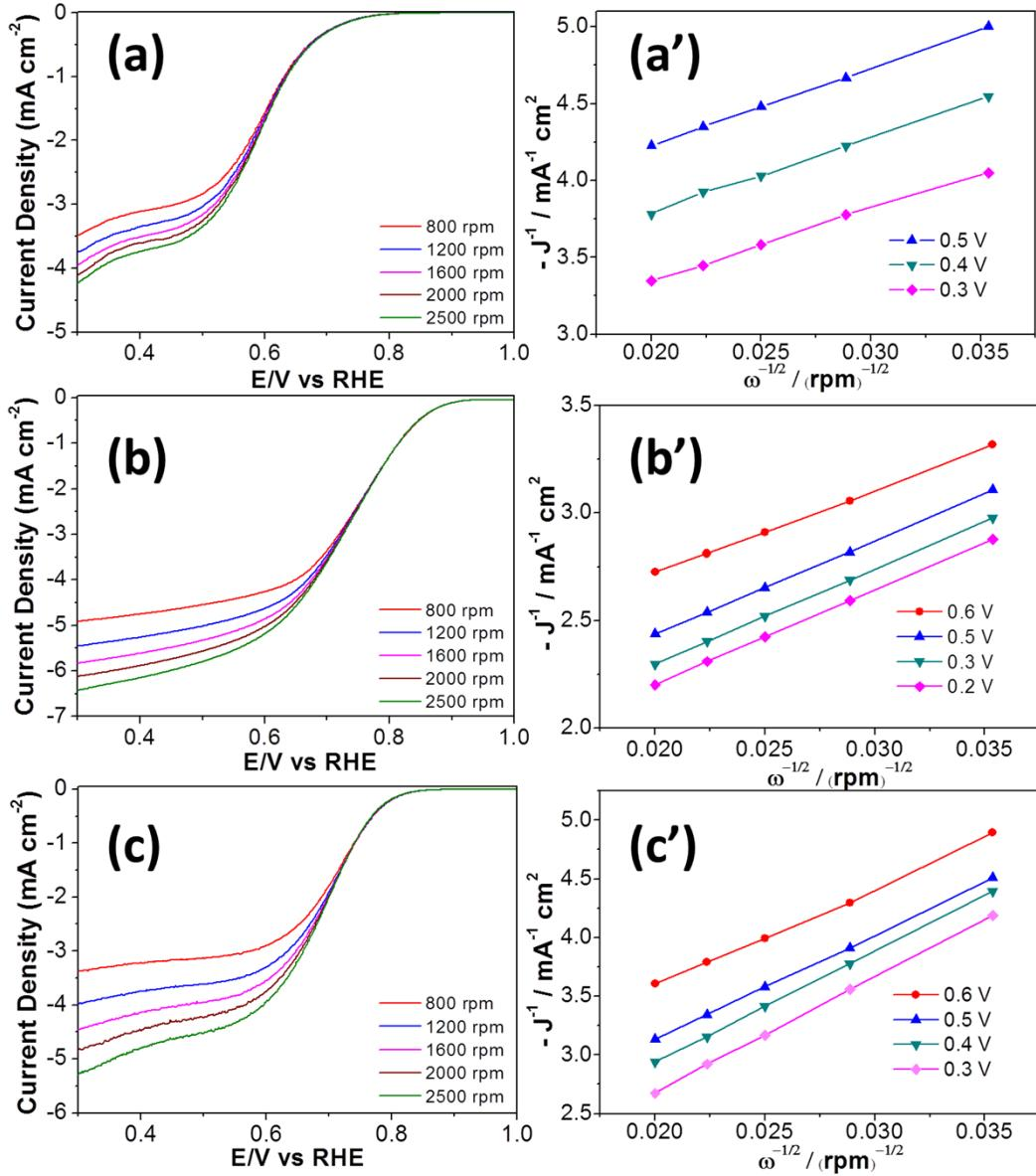
**Figure S5.** ORR polarization curve and K-L plot of (a, a') HNCS61, (b, b') HNCS81, (c, c') HNCS91, respectively. In  $\text{O}_2^-$  saturated 0.1M KOH.
