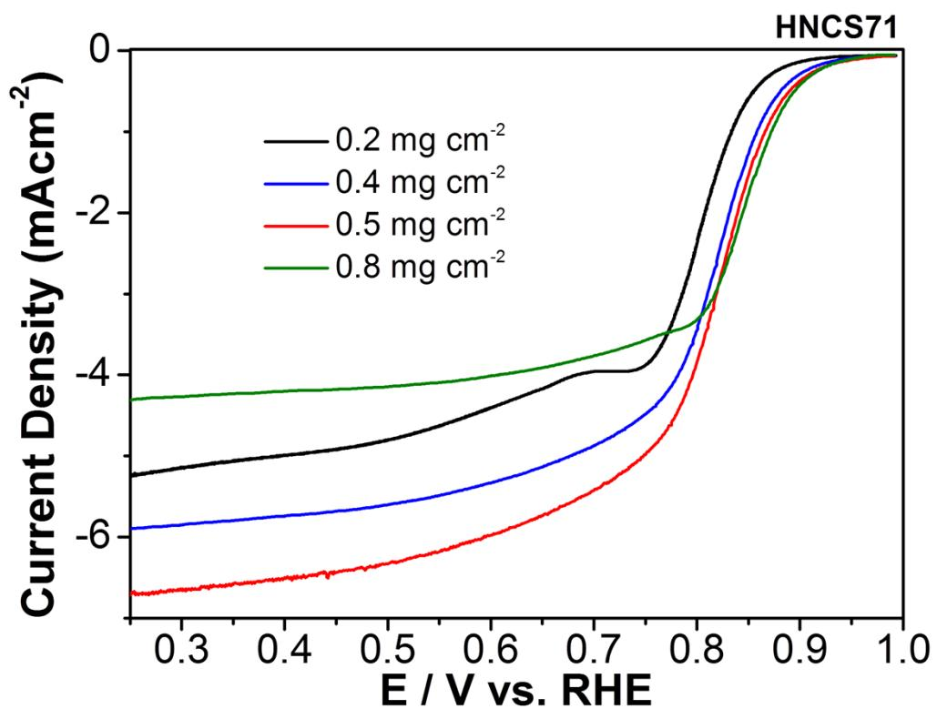
**Figure S4.** ORR polarization curve of HNCS71 with different loading in  $\text{In O}_2^-$ - saturated 0.1M KOH, 1600 rpm.
