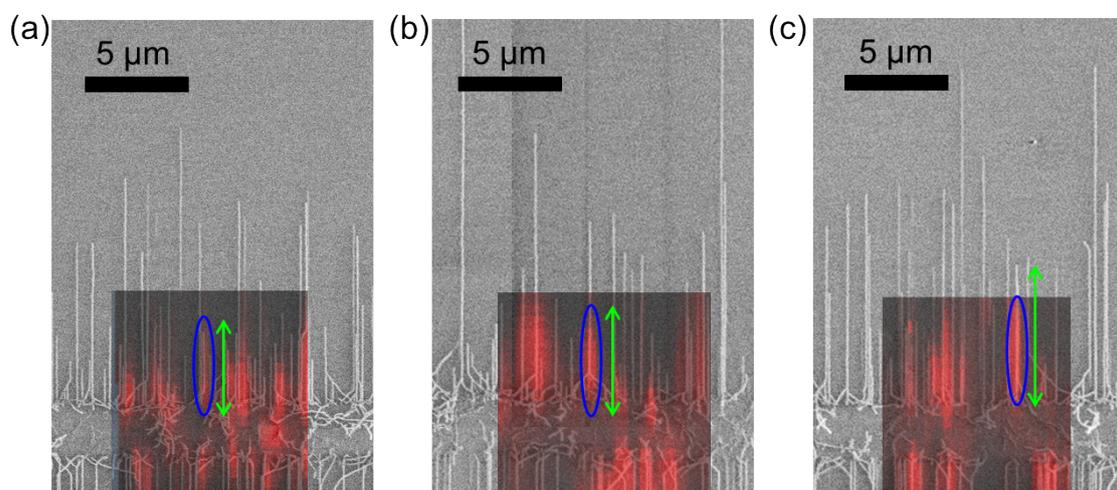
**Fig. S1** Overlapped Raman mapping and SEM images to determine lengths of chirality-assigned SWCNTs. The red contrast of the Raman mapping images represents the G-band intensity of SWCNTs obtained with 488 nm excitation. The blue circles show the areas where RBM spectra of the focused frequency range are detected. The green arrows show the determined SWCNT lengths. (a,b) SWCNT lengths are determined only by Raman mapping images when SWCNT lengths are within Raman mapping
