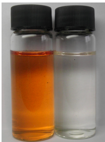
Fig. S4 The appearance of the solutions of acidic 1,10-phenanthroline with the precursor (left) and the 2D-FC (right) dissolved.
