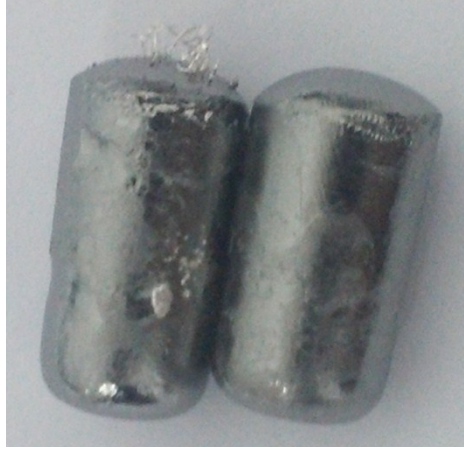
Fig. S7 Ingot samples after high temperature annealing. \text{CuAg}_{1.01}\text{Se} , \text{Cu}_{1.01}\text{AgSe} , and \text{CuAgSe}_{0.99} display the same phenomenon as the left sample with the metallic Ag on the surface. The samples in the Section of 3.1.1-3.1.4 are the right one without obvious metallic Ag observed.
