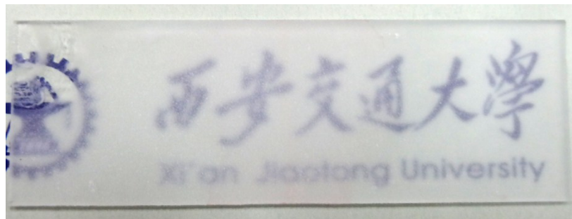
Figure S 7. A camera image of an SAPU coating (as shown in video 3) with its right half side has been immersed in hydrochloric acid solution for 12 h. The red separation line on the SAPU coating during immersion has been erased for a better visual effect.
