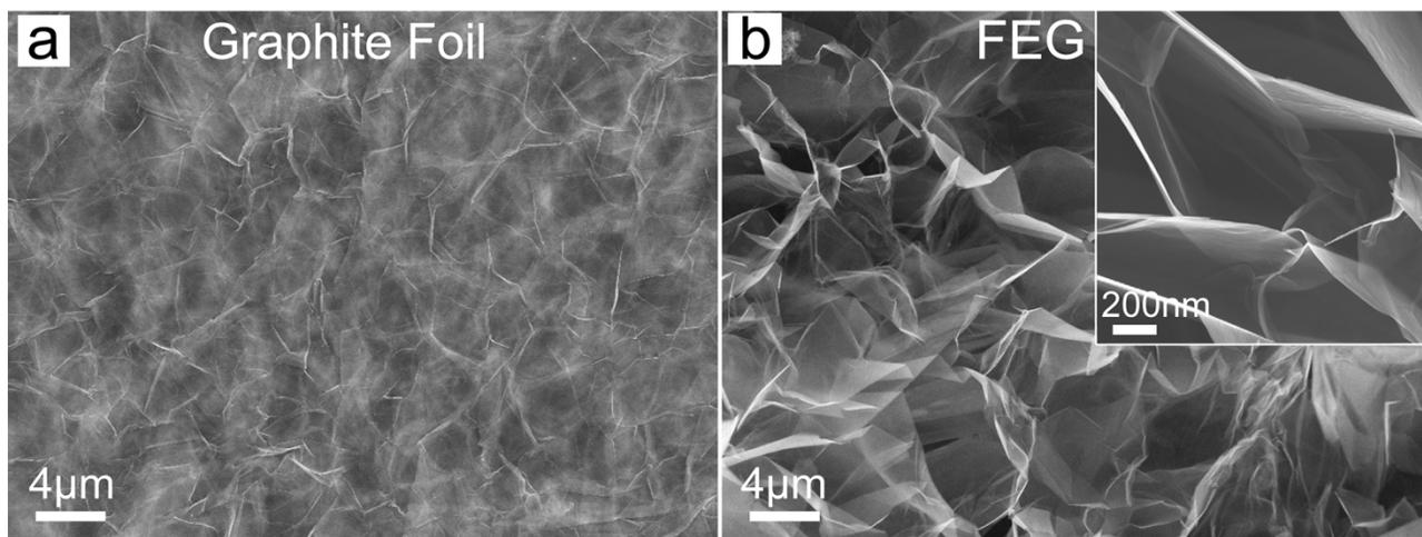
**Figure S1** SEM image of (a) untreated graphite foil and (b) FEG. Inset shows the magnified image of FEG.
