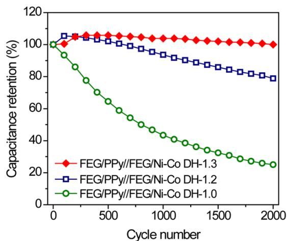
**Figure S5** Cycling stability of the model ASCs with different  $R = Q_-/Q_+$  ( $R=1, 1.2,$  and  $1.3$ ) after 2000 cycles.
