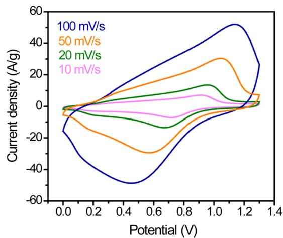
**Figure S7** CV curves of FEG/PPy//FEG/Ni-Co DH-1.3 at different scan rates.
