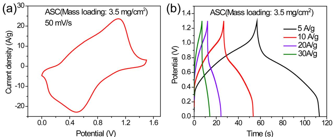
**Figure S8** CV and constant current charge/discharge curves of ASC with higher active materials mass loading of 3.5 mg/cm<sup>2</sup>.
