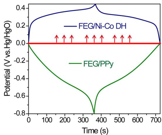
**Figure S6** Schematic diagram of positively shifting upper potential limit of PPy for charge balance with cathode
