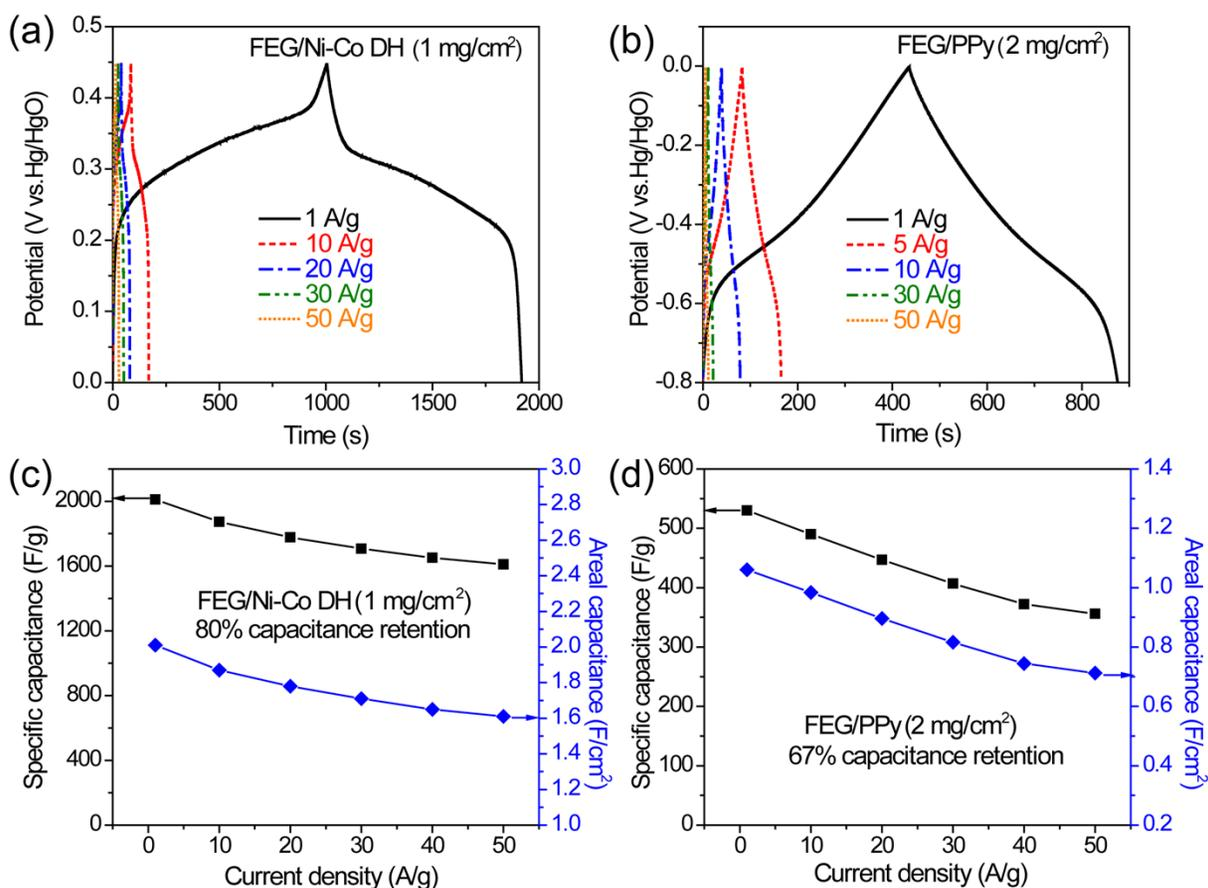
**Figure S4** Constant current charge-discharge profiles of FEG/Ni-Co DH (mass loading: 1 mg/cm<sup>2</sup>) and FEG/PPy (mass loading: 2 mg/cm<sup>2</sup>) measured at different current densities (a, b). Gravimetric/areal specific capacitance of FEG/Ni-Co DH (mass loading: 1 mg/cm<sup>2</sup>) and FEG/PPy (mass loading: 2 mg/cm<sup>2</sup>) measured at different current densities (c, d).
