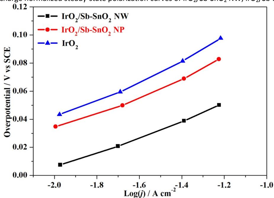
Fig S6 Tafel curves of IrO<sub>2</sub>/Sb-SnO<sub>2</sub> NW, IrO<sub>2</sub>/Sb-SnO<sub>2</sub> NP and IrO<sub>2</sub>
