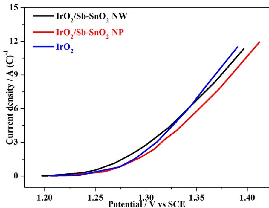
Fig S5 The total charge normalized steady-state polarization curves of IrO<sub>2</sub>/Sb-SnO<sub>2</sub> NW, IrO<sub>2</sub>/Sb-SnO<sub>2</sub> NP and IrO<sub>2</sub>
