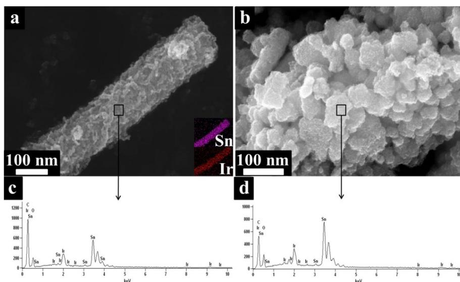
Fig S2 SEM images (a) (inset is SEM and the corresponding elemental mapping from EDX mapping image) and EDX images (c) of IrO<sub>2</sub>/Sb-SnO<sub>2</sub> NW, SEM images (b) and EDX images (d) of IrO<sub>2</sub>/Sb-SnO<sub>2</sub> NP
