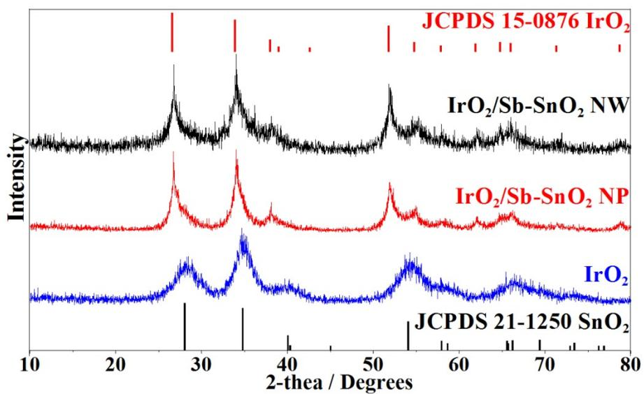
Fig S3 XRD patterns of IrO<sub>2</sub>/Sb-SnO<sub>2</sub> NW, IrO<sub>2</sub>/Sb-SnO<sub>2</sub> NP and IrO<sub>2</sub>
