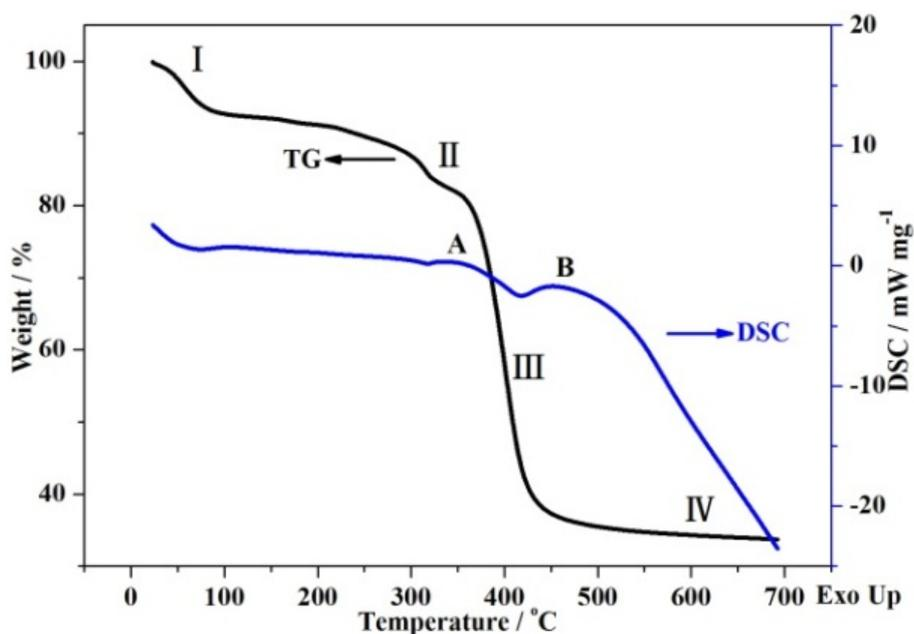
Fig S1 TG-DSC curves of the as-spun Sb-SnO<sub>2</sub> NW precursors
