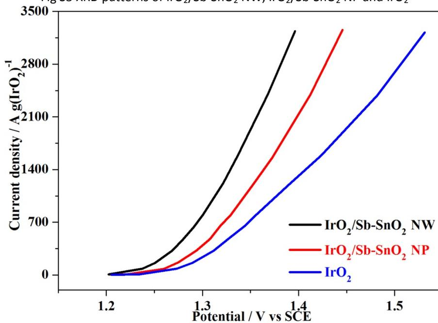
Fig S4 Mass normalized steady-state polarization curves of IrO<sub>2</sub>/Sb-SnO<sub>2</sub> NW, IrO<sub>2</sub>/Sb-SnO<sub>2</sub> NP and IrO<sub>2</sub>
