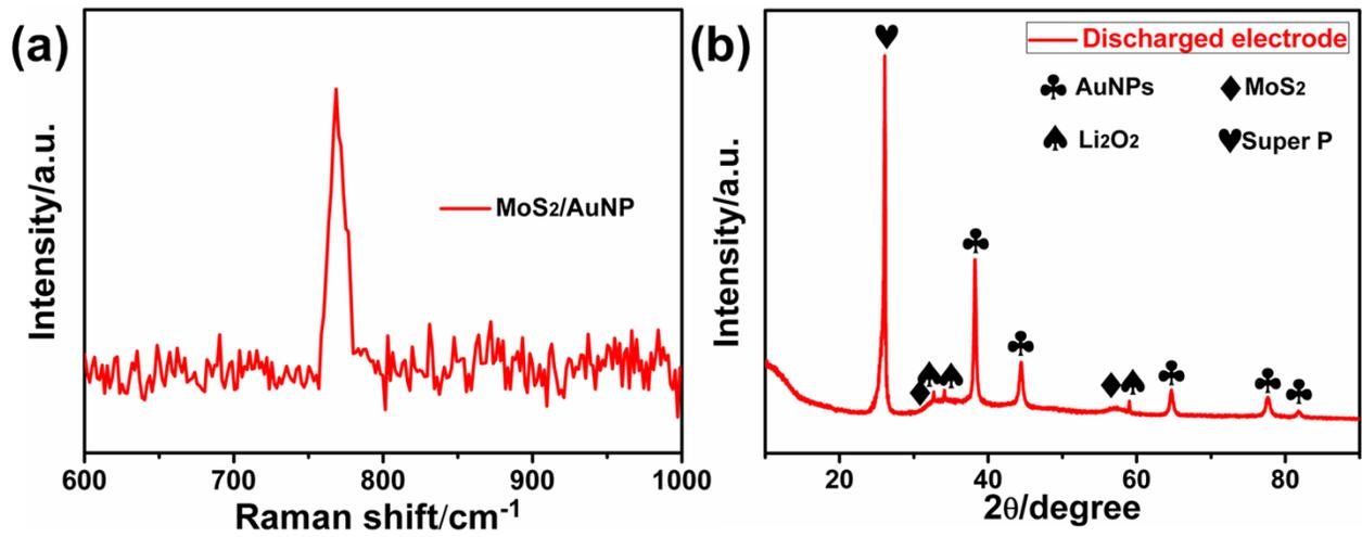
Fig. S5 (a) Raman spectrum and (b) XRD pattern of the discharge product on the electrode modified with MoS<sub>2</sub>/AuNP nanohybrids.
