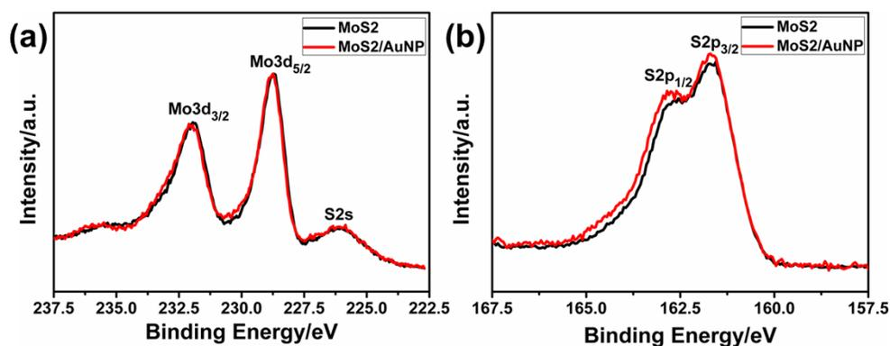
**Fig. S1** XPS spectra for (a) Mo and (b) S binding energies of MoS<sub>2</sub> nanoflowers and MoS<sub>2</sub>/AuNP nanohybrids.
