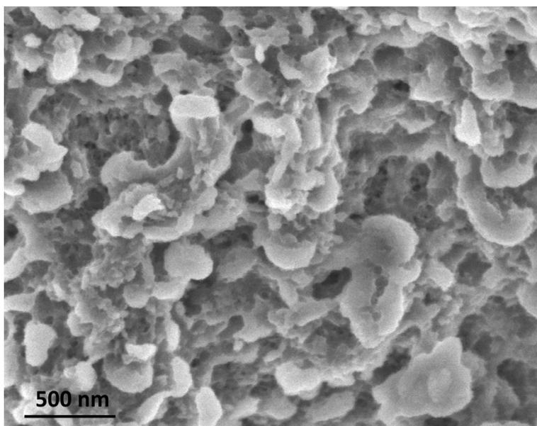
**Fig. S4** SEM image of the electrode modified with MoS<sub>2</sub>/AuNP nano hybrids after discharging.
