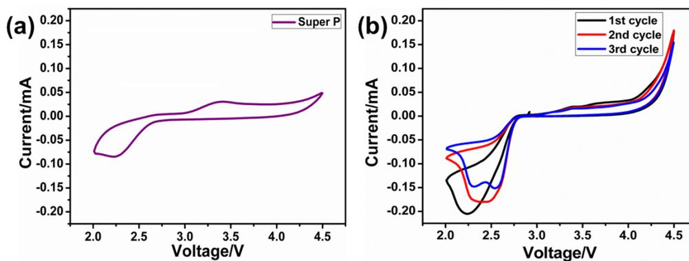
**Fig. S3** CVs of (a) Super P and (b) MoS<sub>2</sub>/AuNP nano hybrids with the first to three cycles at 0.1 mV·s<sup>-1</sup> scan rate and voltage of 2.0 V to 4.5 V.
