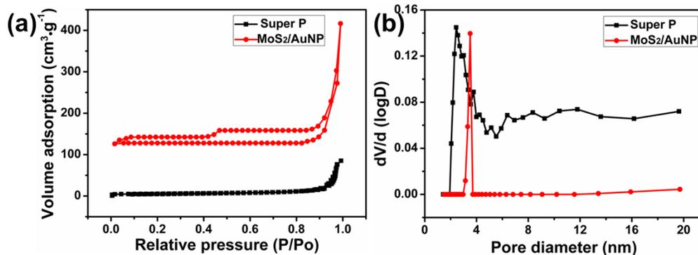
**Fig. S2** (a) Nitrogen-adsorption-desorption isotherms, (b) pore-size distributions of Super P and MoS<sub>2</sub>/AuNP nano hybrids.
