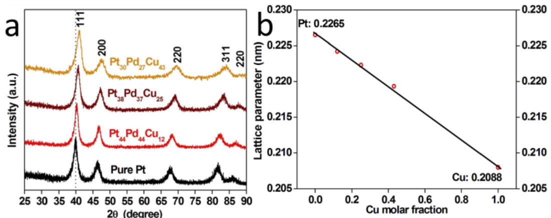
**Figure S1** (a) Wide-angle XRD patterns of the pure Pt and ternary nanoporous PtPdCu spheres with different molar ratios of Cu and (b) the relationship of the (111) diffraction angles vs. Cu molar fractions in ternary nanoporous PtPdCu.
