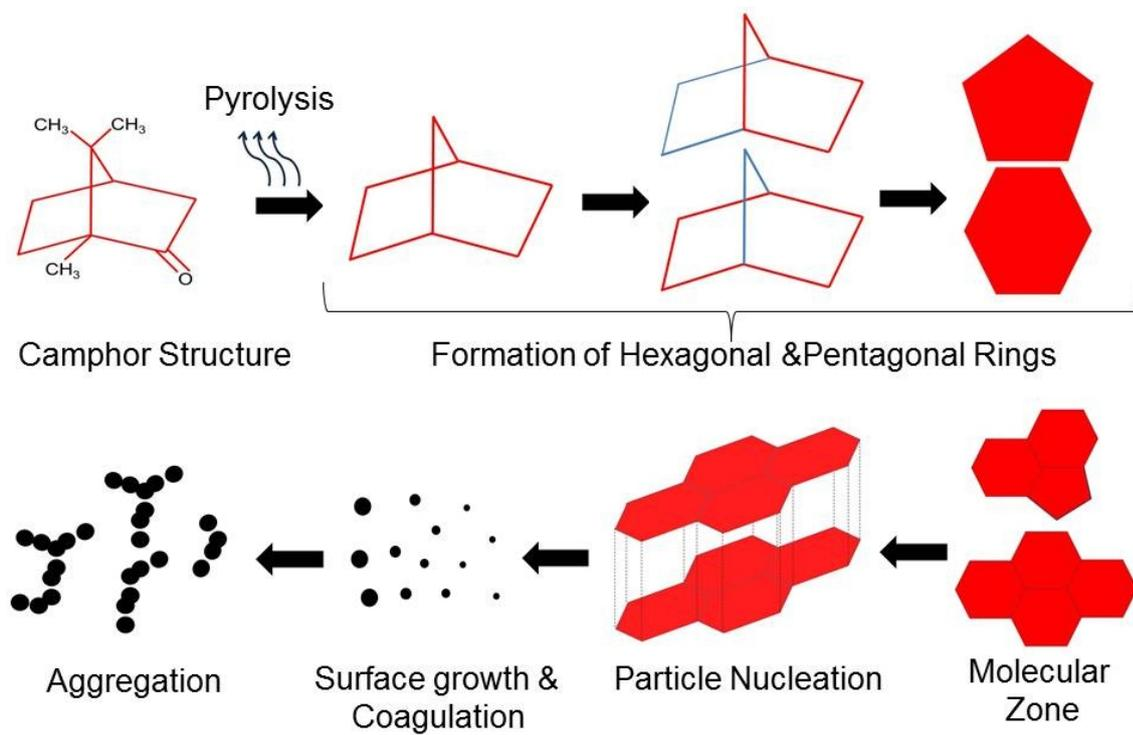
Figure S2. Schematic illustration showing the formation mechanism of graphitic carbon nanobeads obtained from camphor.
