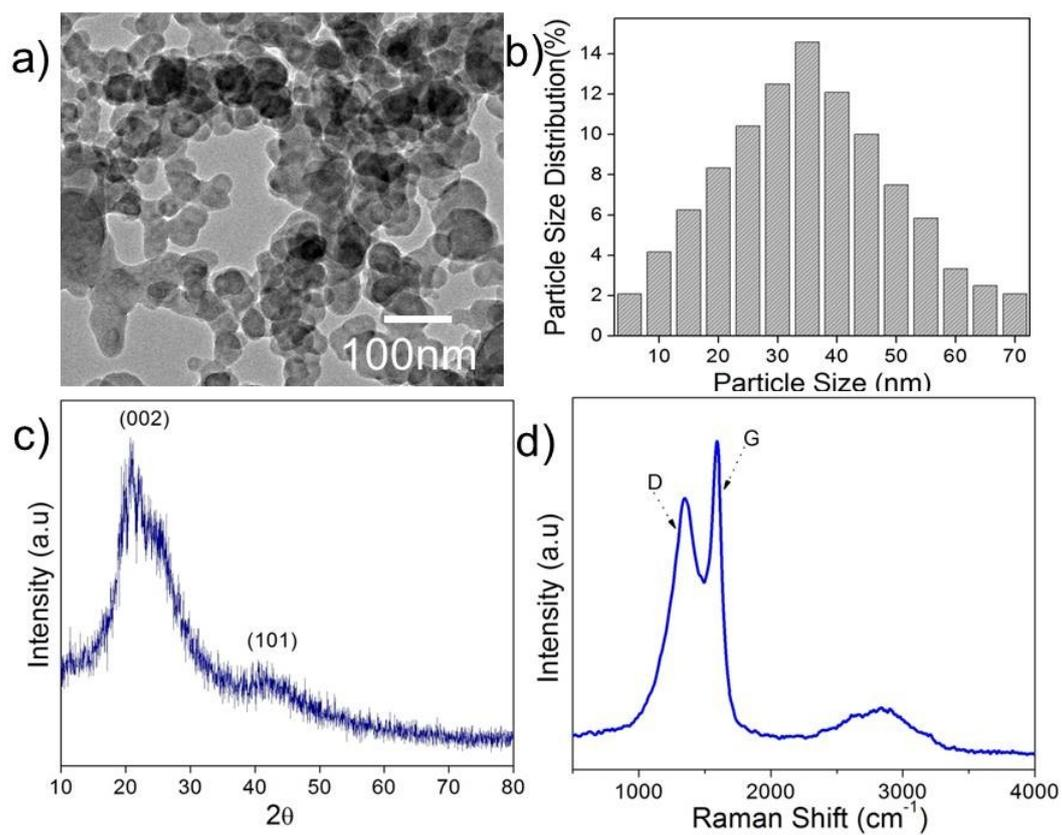
Figure S1. (a) TEM images, (b) diameter size distribution, (c) XRD and (d) Raman spectra of the carbon nanobeads used as the precursors for synthesizing carbon sponges.
