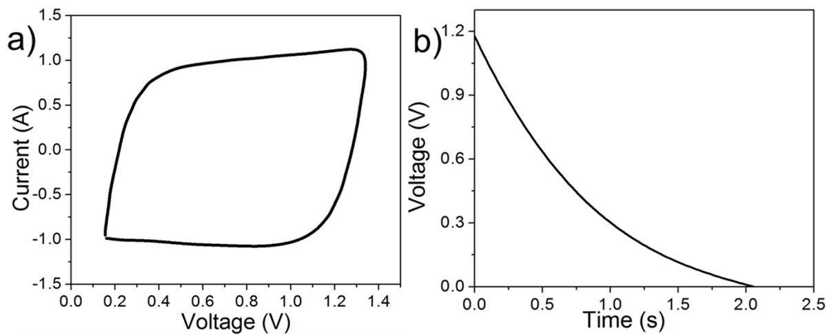
Figure S7. (a) Typical cyclic voltammetry curve at a scan rate of  $100 \text{ mVs}^{-1}$  and (b) galvanostatic discharge curve at a current density of  $1.5 \text{ mA}$  for the commercial AEC.
