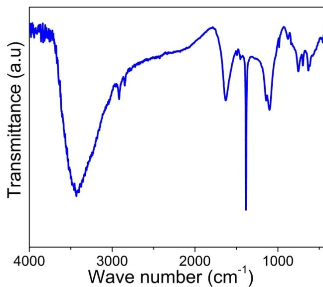
Figure S5. Typical FT-IR spectrum of the S-3 carbon sponge. The spectrum showed O-H stretching (3200-3400 cm<sup>-1</sup>), C=O and C-O stretching (1629 cm<sup>-1</sup>) and aromatic C=C stretching (1400-1600 cm<sup>-1</sup>). The bands corresponding to anti-symmetric and symmetric stretching vibrations of =CH<sub>2</sub> were seen at 2925 and 2853 cm<sup>-1</sup>, respectively.
