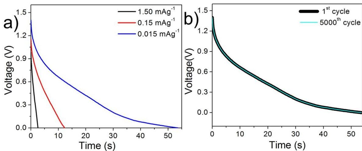
Figure S6. (a) Constant current discharge curves of S-3 sample at different current densities. (b) Constant current discharge curves of S-3 at the 1<sup>st</sup> cycle and the 5000<sup>th</sup> cycle at a current density of 0.015 mA g<sup>-1</sup>.
