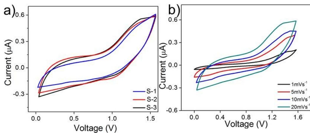
Figure S4. CV curves of (a) sponges at different surfactant concentrations at a scan rate of 20  $\text{mV/s}$ , and (b) S-3 at different scan rates from 1 to 20  $\text{mVs}^{-1}$ .
