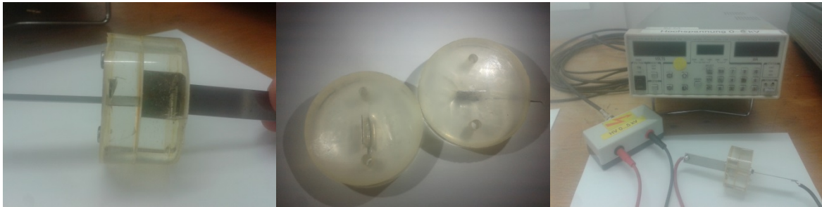
Figure 13S. Electrodes used for breakdown strength measurements (left and right). Two conductive plates with a thickness of 1 mm were embedded in an epoxy matrix. The embedded electrodes were polished to a smooth surface. The thickness of the sample is measured prior the breakdown measurement. The two electrodes are used as shown on the left. The overall set-up of the system is depicted on the right.
