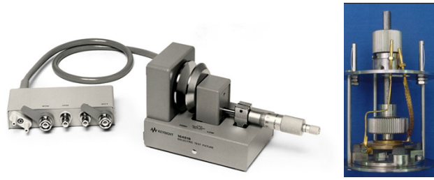
Figure 14S. The setul used for measuring the dielectric properties.
