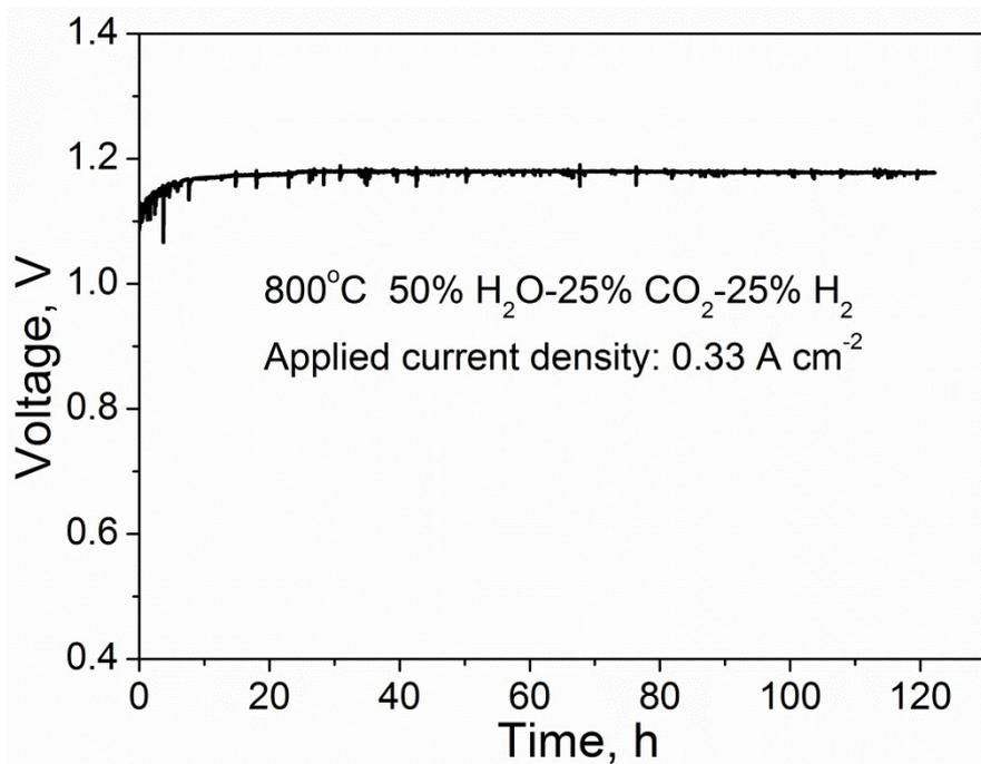
Fig. S8. A 0.33 A cm<sup>-2</sup> constant current co-electrolysis testing of Ni-SDC-YSZ/YSZ/LSM-SDC-YSZ cell fabricated by Freeze-drying Tape-casting and infiltration method in 50 vol.% H<sub>2</sub>O-25 vol.% CO<sub>2</sub>-25 vol.% H<sub>2</sub> at 800°C.
