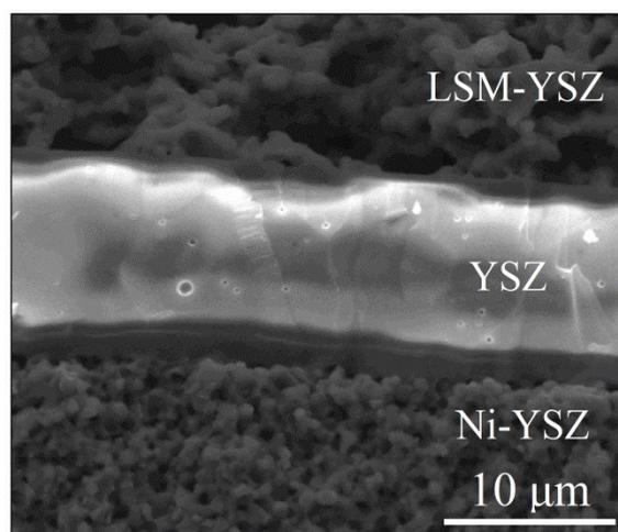
Fig. S1. Cross sectional SEM micrographs of LSM-YSZ/YSZ/Ni-YSZ single cell fabricated by traditional dry-pressing and screening-printing method.
