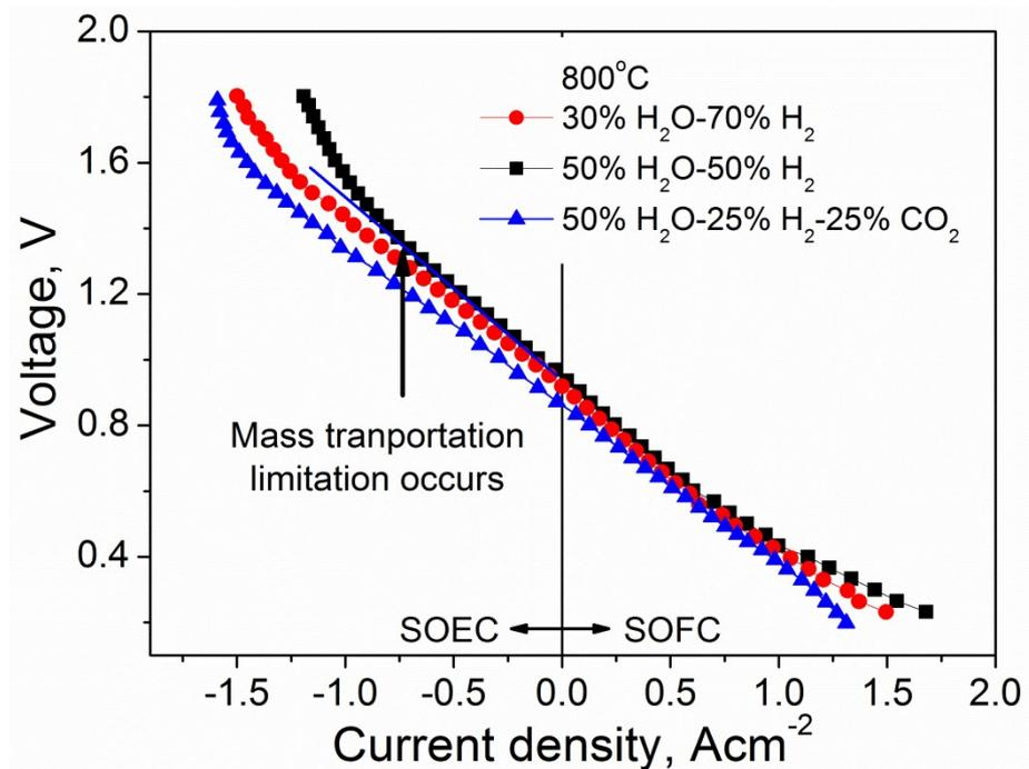
Fig. S4. DC potential-current density curves of Ni-SDC-YSZ/YSZ/LSM-SDC-YSZ single cells fabricated by dry-pressing and infiltration method operated in 50 vol.% H<sub>2</sub>O-50 vol.% H<sub>2</sub> at 800°C.
