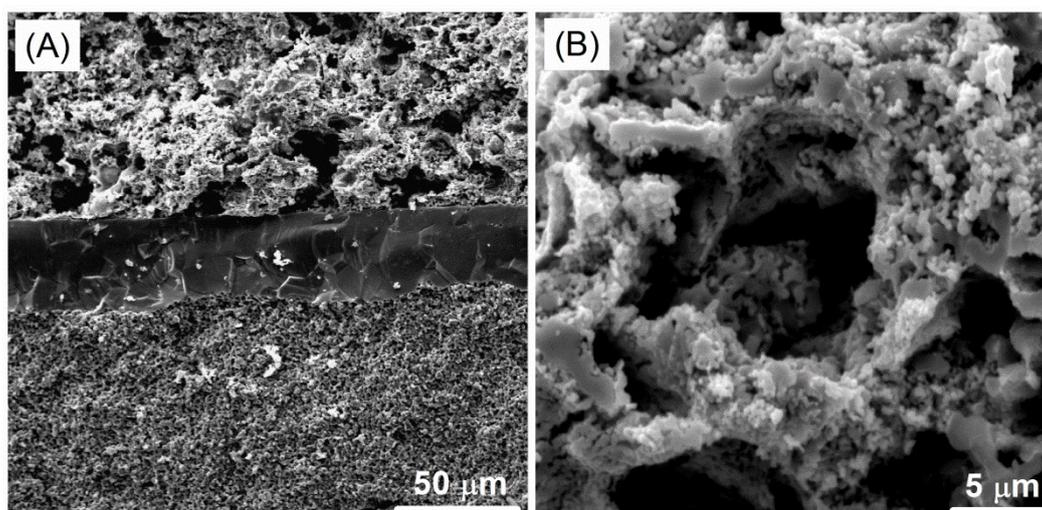
Fig. S3. (A) Cross-sectional SEM image of Ni-SDC-YSZ/YSZ/LSM-SDC-YSZ SOEC after electrolysis test, and (B) SEM images of LSM-SDC infiltrated LSM-SDC-YSZ oxygen electrode after electrolysis test.
