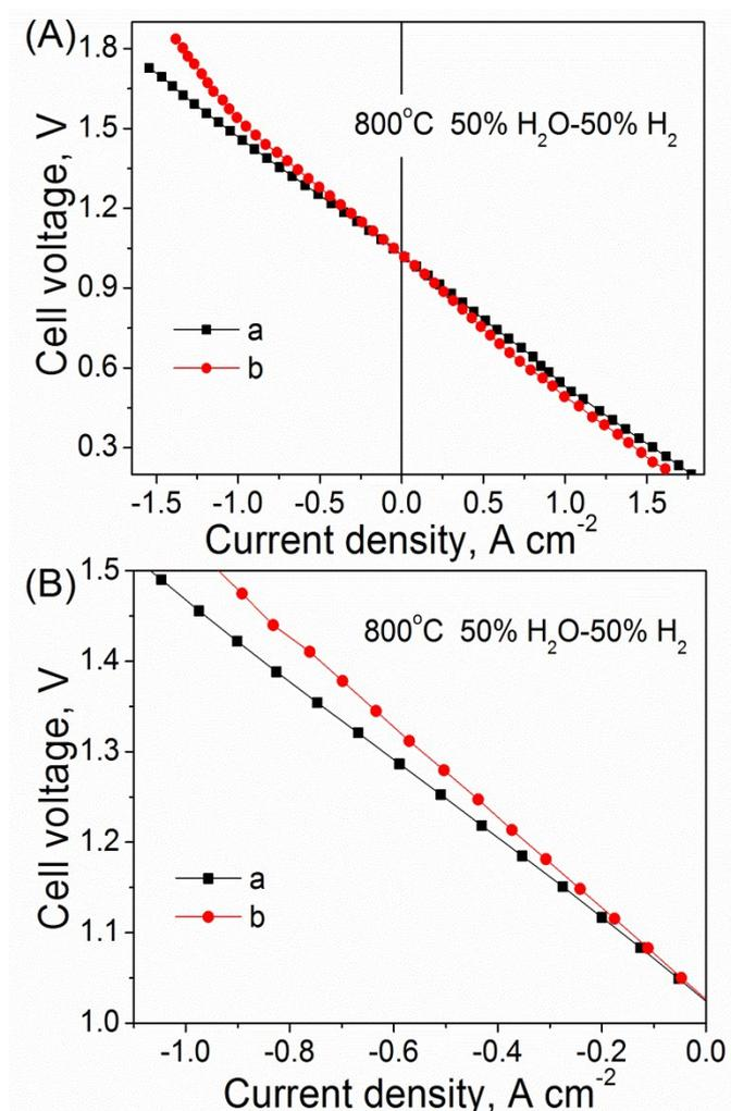
Fig. S7. DC potential-current density curves of Ni-SDC-YSZ/YSZ/LSM-SDC-YSZ single cells in fuel cell mode and co-electrolysis mode (A) or in co-electrolysis mode (from open circuit voltage (OCV) to 1.5 V) (B), fabricated by freeze-drying tape-casting and infiltration method (a) or traditional dry-pressing and infiltration method (b) in 50 vol.% H<sub>2</sub>O-50 vol.% H<sub>2</sub> at 800°C, respectively.
