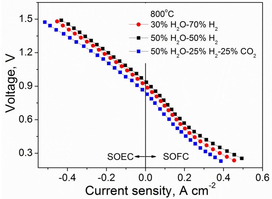
Fig. S2. DC potential-current density curves of LSM-YSZ/YSZ/Ni-YSZ cell operated in 50 vol.% H<sub>2</sub>O-50 vol.% H<sub>2</sub> at 800°C.
