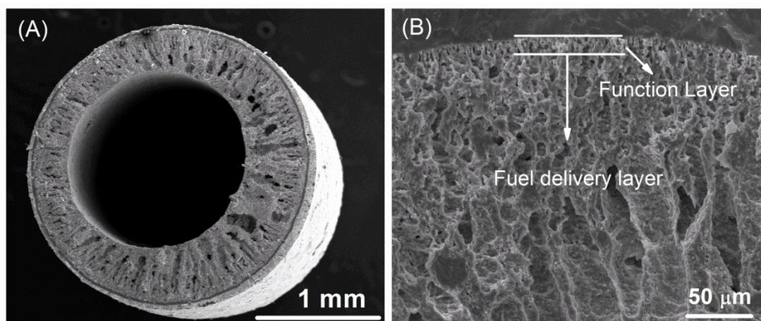
Fig. S5. (A) Overall view of the hydrogen electrode-supported Micro-tubular SOEC, (B) cross-sectional fracture surface micrograph of the hydrogen electrode-supported MT-SOC, indicating the microstructure of the hydrogen electrode fuel delivery layer and function layer.
