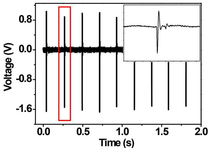
**Figure S1.** Output voltage of PVDF film with opposite polarization direction. The PVDF with opposite polarization is subjected to the periodic mechanical compressive force. The polarity of the output voltage is reversed.
