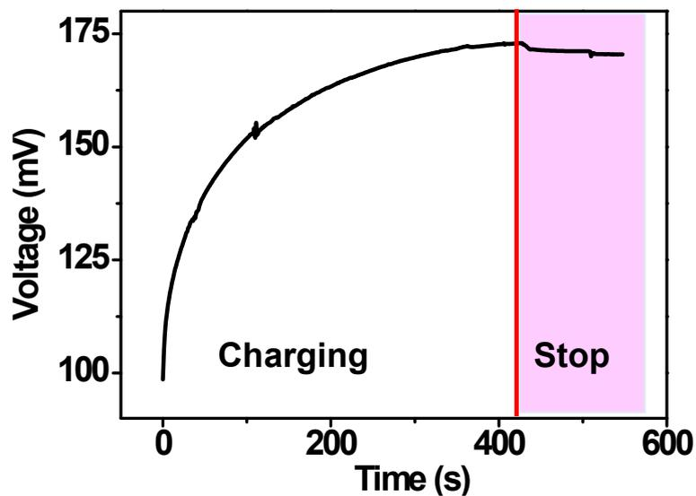
**Figure S3.** The piezo-supercapacitor without discharging at the initial stage is under compressive stress. The voltage of the device increased from 98 mV to 172 mV within 440 s and can sustain for a long time.
