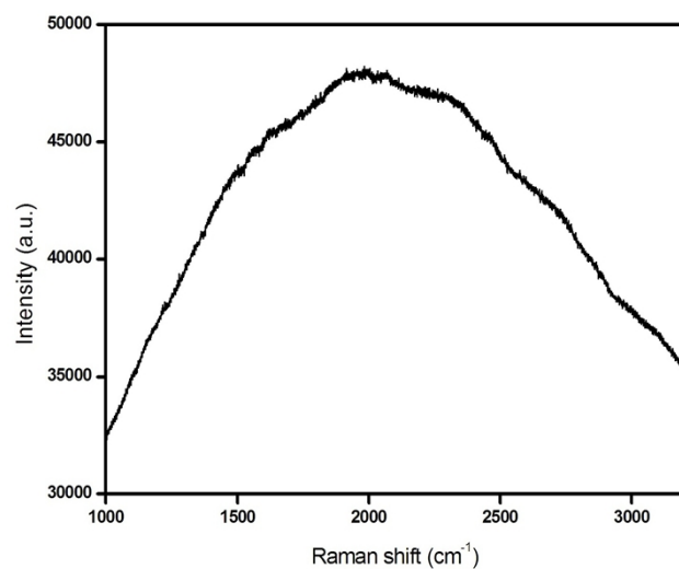
Fig. S3 Raman Spectrum of carbon nanodots. The absence of D and G band indicates the amorphous nature of the carbon nanodots.
