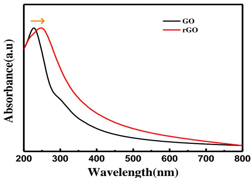
**Figure S1.** The UV-Visible spectrum of GO and rGO.
