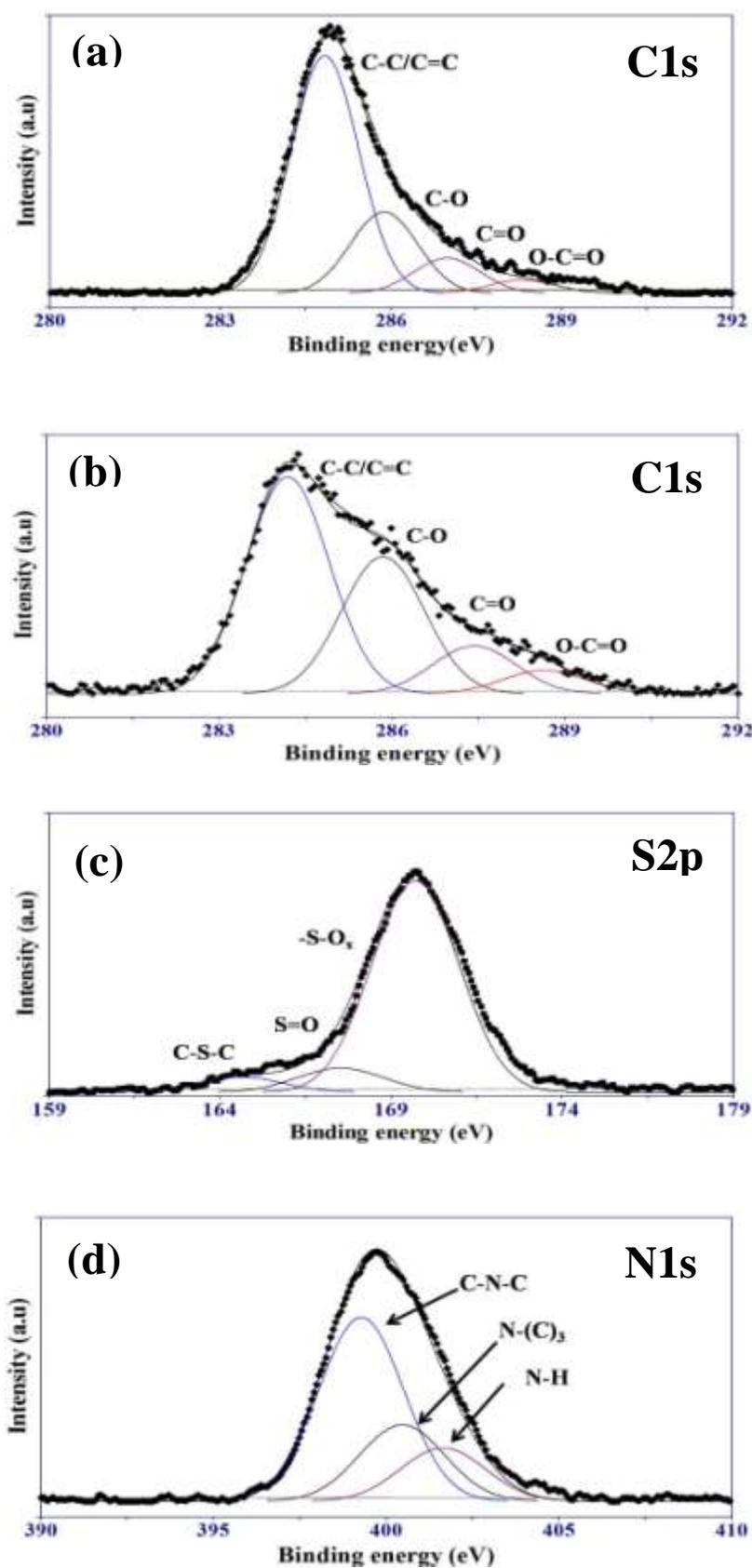
**Figure S7.** The Hi-resolution XPS spectra of (a) C1s of rGO and (b-d) C1s, S2p and N1s spectrum of rGO/CQDs-HP respectively.
