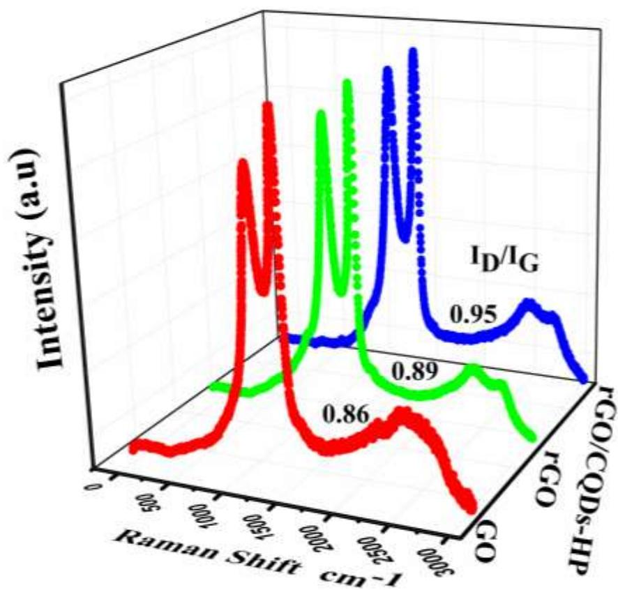
**Figure S8.** The Raman spectrum of GO, rGO and rGO/CQDs-HP.
