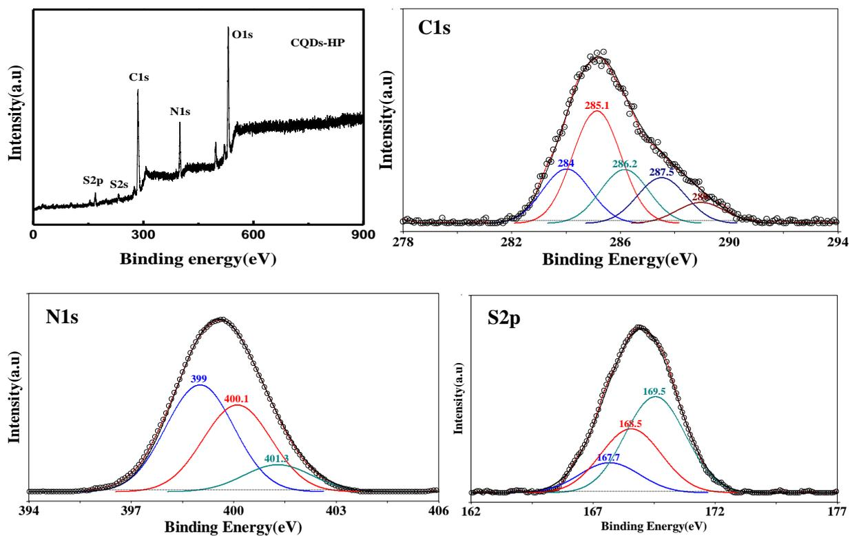
**Figure S5.** Full survey and the Hi-resolution XPS spectra of C1s, N1s and S2p of CQDs-HP.
