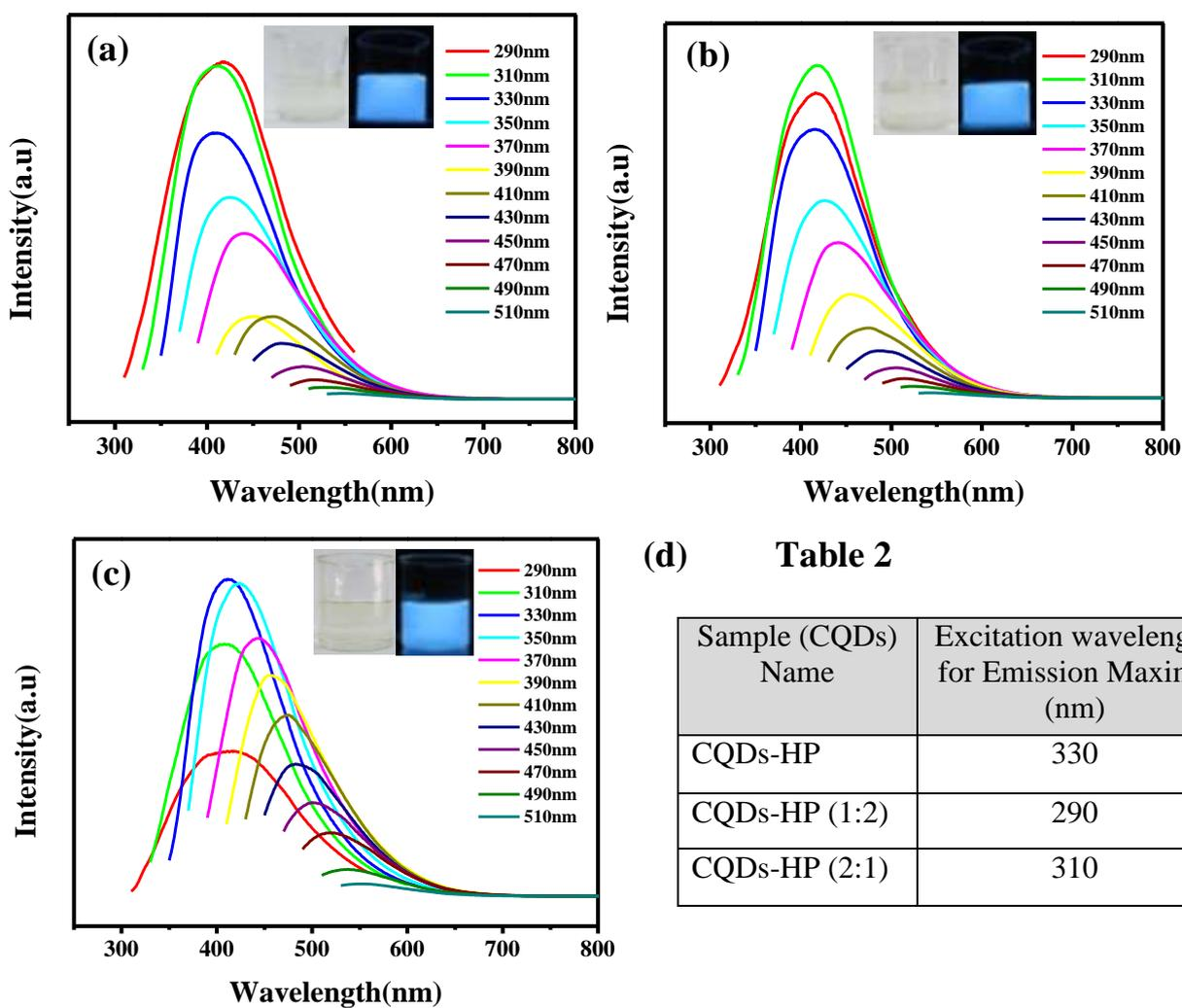
**Figure S4.** Photoluminescence emission spectrum for (a) CQDs-HP (1:2), (b) CQDs-HP (2:1) and (c) CQDs-HP. (d) Table 2 summarizes the excitation wavelength for corresponding emission maxima.
