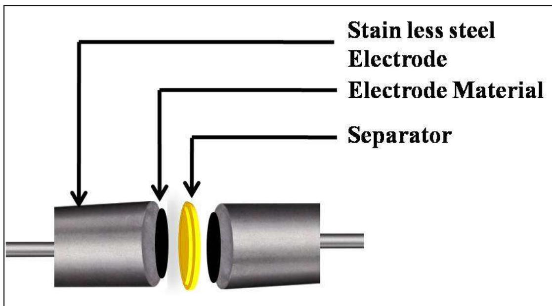
**Figure S9.** Scheme showing the arrangement of the symmetrical electrode. The sample was placed on the well polished stainless steel electrodes and the arrangement was carried out by placing a cellulose nitrate membrane as separator.
