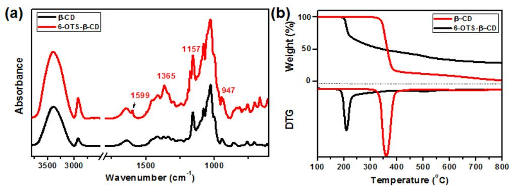
**Fig. S1** (a) FT-IR spectra and (b) TGA analyses (N<sub>2</sub>, 20°C·min<sup>-1</sup>) of 6-OTS-β-CD and β-CD
