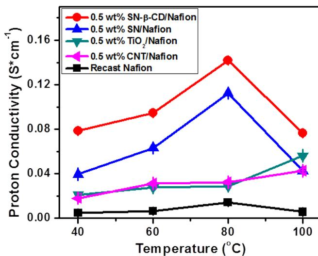
**Fig.S6** Temperature-dependent (40 RH%) proton conductivity of recast Nafion, 0.5 wt% SN-β-CD/Nafion, 0.5 wt% SN/Nafion, 0.5 wt% TiO<sub>2</sub>/Nafion and 0.5 wt% CNT/Nafion composite PEMs.
