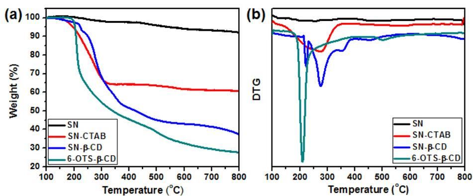
**Fig. S2** TGA (a) and DTG (b) curves of SN, SN-CTAB, SN-β-CD and 6-OTS-β-CD.
