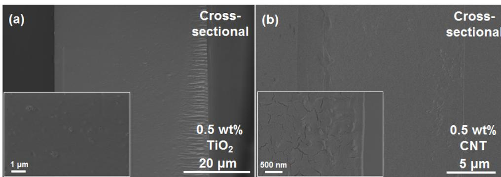
**Fig.S5** SEM images of (a) 0.5 %wt TiO<sub>2</sub>/Nafion and (b) 0.5 %wt CNT/Nafion.
