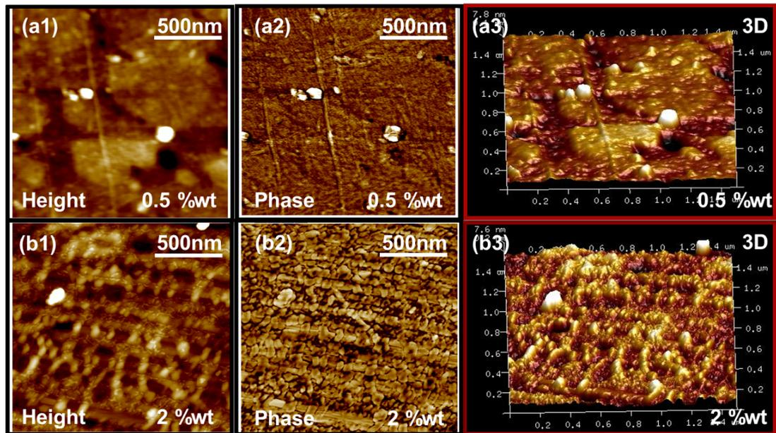
**Fig. S3** 2D-height and phase AFM images of (a1-a2) 0.5 wt% SN- $\beta$ -CD/Nafion and (b1-b2) 2 wt% SN- $\beta$ -CD/Nafion. Corresponding 3D-AFM images of (a3) 0.5 wt% SN- $\beta$ -CD/Nafion and (b3) 2 wt% SN- $\beta$ -CD/Nafion.
