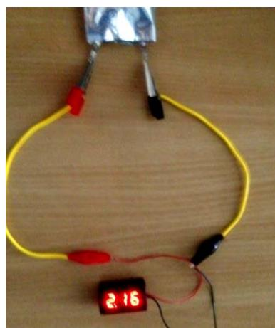
**Figure S12.** Digital photo of two ASCs connected in series that can power a commercial digital meter brightly after charging for 5 min.
