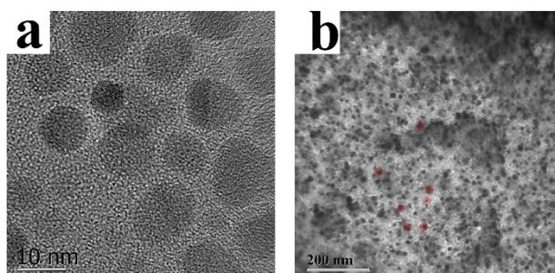
Fig. S7 TEM images of magnetic nanoparticles (a); TEM images of part of microspheres after assembly (b) and magnetic nanoparticles after assembly are signed by red circles.
