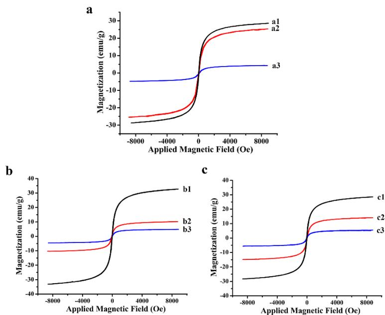
Fig.S8 Magnetic hysteresis loop of CS(2.0)-5 calcined for second time (a1), CS(2.0)-5 (a2) and MS(2.0)-5 (a3) in (a). Magnetic hysteresis loop of CS(1.5)-5 (b1), CS(1.5)-2 (b2) and CS(1.5)-1 (b3) in (b). Magnetic hysteresis loop of CS(1.8)-5 (c1), CS(1.8)-2 (c2) and CS(1.8)-1 (c3) in (c).
