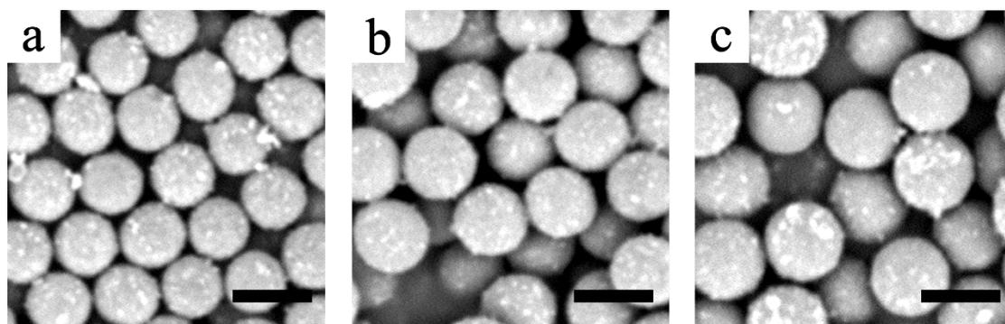
Fig.S3 SEM images of MF(1.5)@SiO<sub>2</sub>, MF(1.8)@SiO<sub>2</sub>, MF(2.0)@SiO<sub>2</sub>
