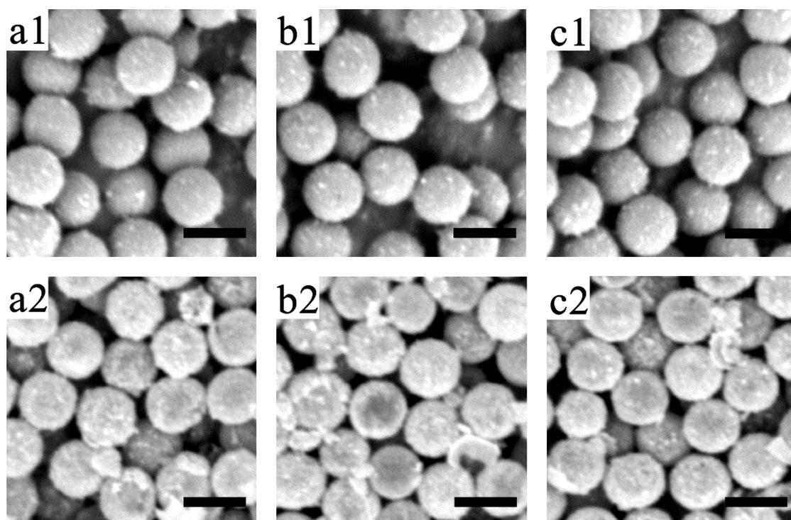
Fig.S5 SEM images of MS(1.8)-1 (a1) , MS(1.8)-2 (b1) and MS(1.8)-5 (c1) and CS(1.8)-1 (a2), CS(1.8)-2 (b2) and CS(1.8)-5 (c2). Scale bar in each image = 2  $\mu$ m.
