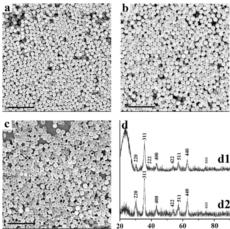
Fig. S6 SEM images of CS(1.5)-5 in (a), CS(1.8)-5 in (b) and CS(2.0)-5 in (c). The XRD patterns of MS(2.0)-5 (line d1) and CS(2.0)-5 (line d2) in (d). Scale bar in (a), (b) and (c) is 10  $\mu\text{m}$ .
