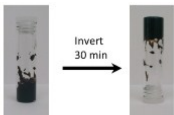
ESI 3. Picture of SWCNTs reduced at 10:1 C:Na in DMAc with a CNT system loading of 6.5 \text{ mg mL}^{-1}
