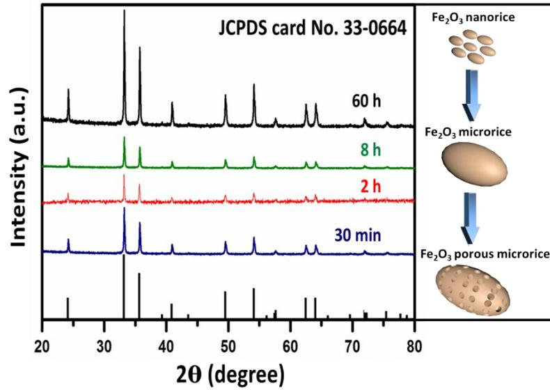
Figure S2 XRD analysis of all the products with a reaction time of 30min, 2h, 8h and 60h. The schematic illustration of the formation process of  $\text{Fe}_2\text{O}_3$  porous microrices
