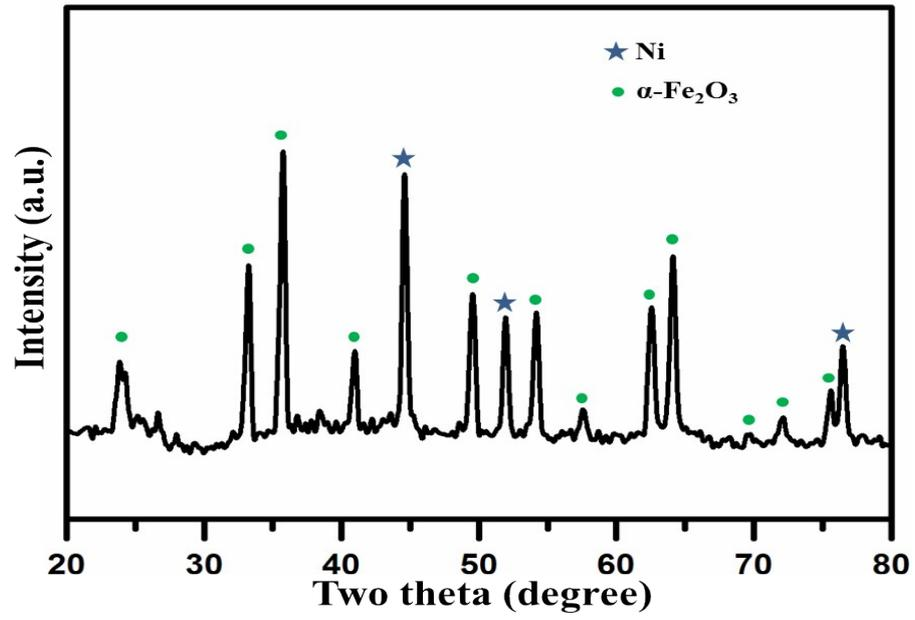
Figure S4 The XRD pattern of the Fe<sub>2</sub>O<sub>3</sub>-60@C electrode after 50 cycles. The Ni signal is attributed to the Ni foam which is used as the current collector of the battery.
