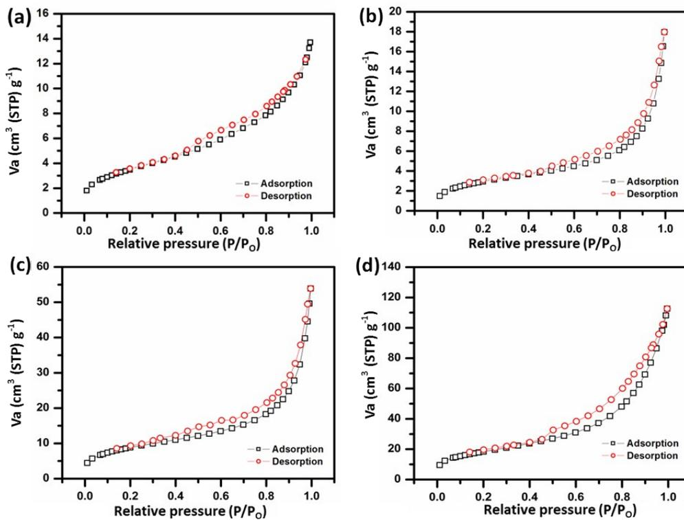
Figure S3 Nitrogen adsorption–desorption isotherms of the  $\text{Fe}_2\text{O}_3$  porous microrices
