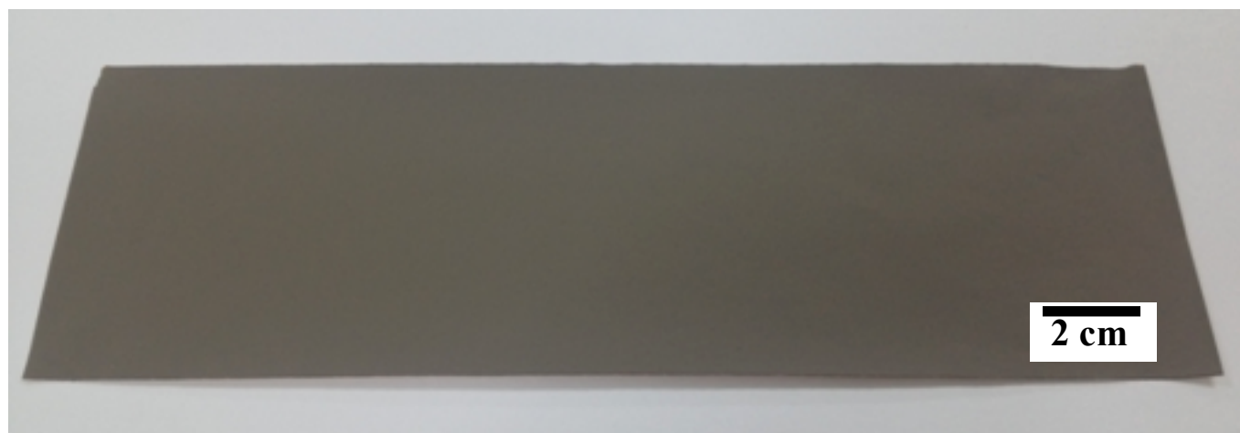
Figure S4. A digital photograph of a uniformly coated electrode film (7cm×22cm) consisting of Si micro-plates, Super P carbon blacks and alginate binder.
