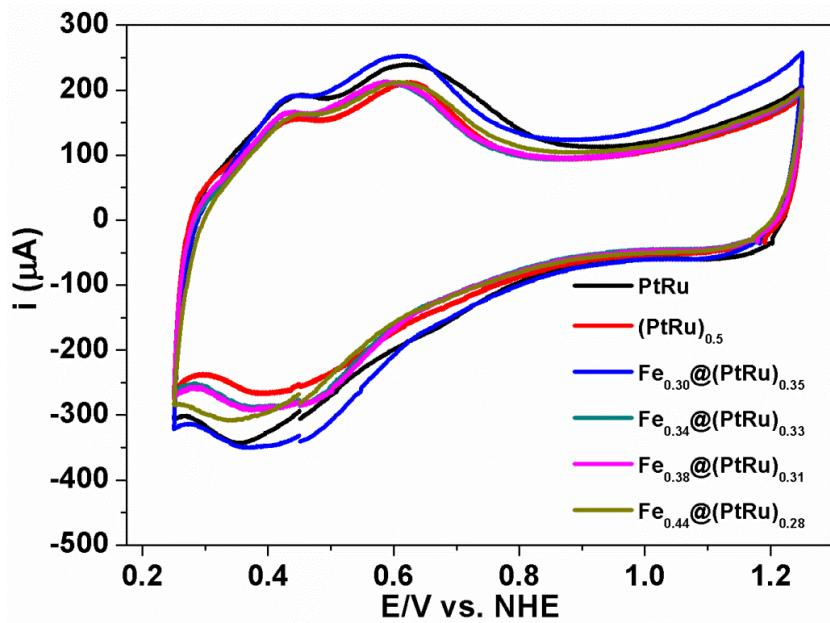
Fig. S5 CV curves of Cu-stripping measurements on  $\text{Fe}_x @ (\text{PtRu})_{(1-x)/2}$  ( $x = 0, 0.30, 0.34, 0.38, 0.44$ ) and PtRu samples measured in  $0.1 \text{ HClO}_4$  aqueous solution containing  $1 \text{ M CuSO}_4$ .
