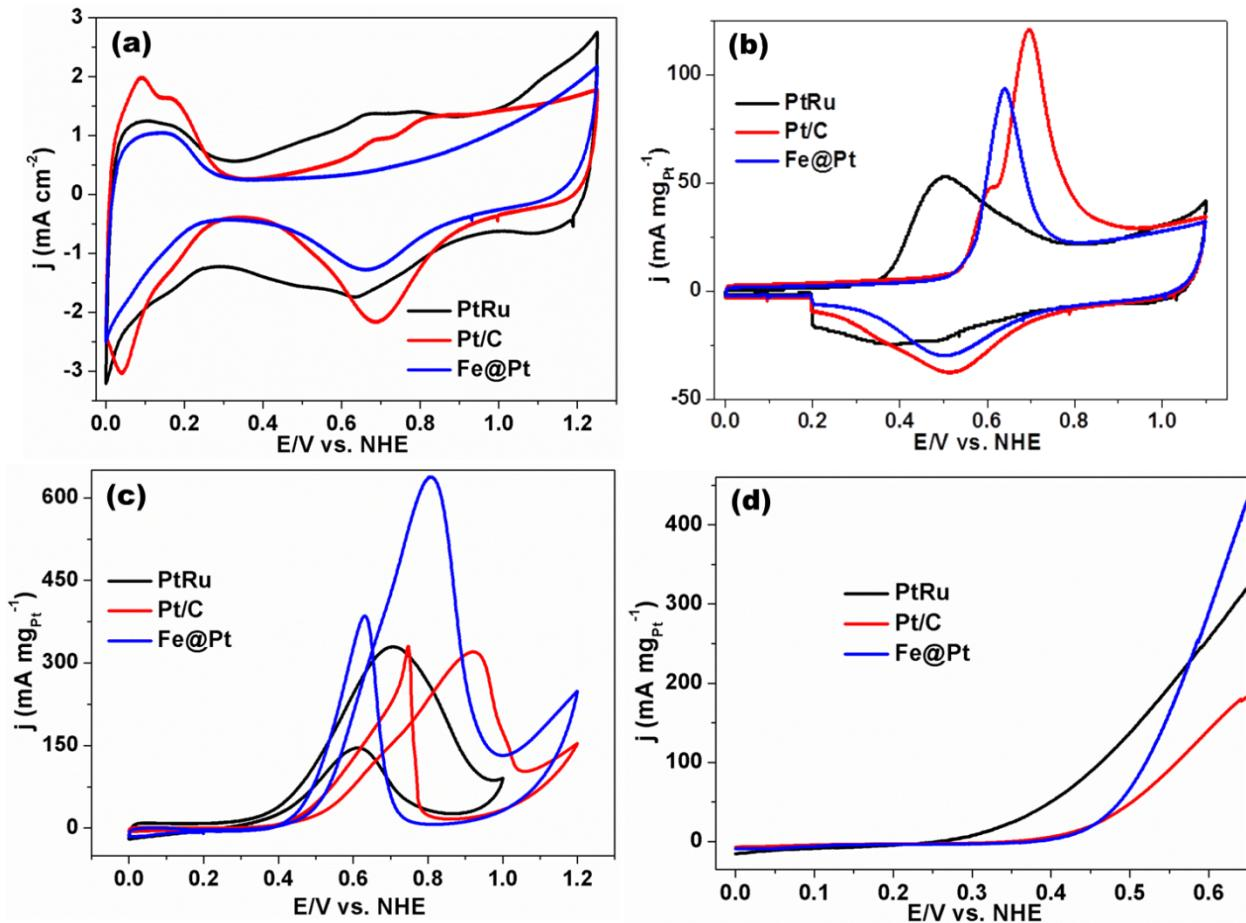
Fig. S3 Comparison of electrochemical data of PtRu, Pt/C, and Fe@Pt: (a) CV, (b) CO-stripping curve, (c) CV of MOR, and (d) LSVs of MOR.
