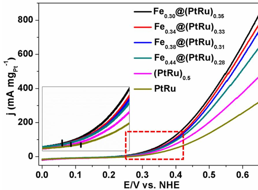
Fig. S6 LSVs of  $\text{Fe}_x @ (\text{PtRu})_{(1-x)/2}$  ( $x = 0.0, 0.30, 0.34, 0.38, 0.44$ ) and PtRu samples measured in an electrolyte of 0.1  $\text{HClO}_4$  containing 1 M  $\text{CH}_3\text{OH}$ . Inset shows onset potentials of MOR on all catalysts.
