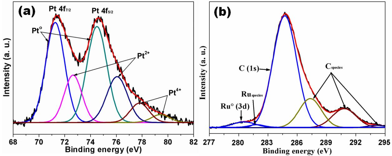
Fig. S2 XPS spectra on (a) Pt 4f region and (b) Ru 3d region of PtRu sample.
