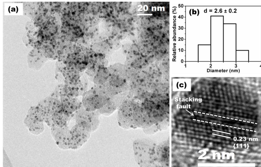
Fig. S1 (a) TEM image, (b) particle size distribution plot (by counting 200 NPs), and (c) HRTEM image of  $(\text{PtRu})_{0.5}$ .
