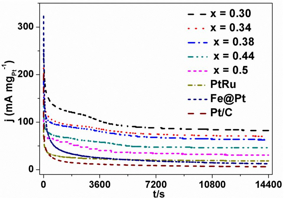
Fig. S4 Chronoamperometric curves of  $x = 0.0, 0.30, 0.34, 0.38$ , and  $0.44$  samples, PtRu, Fe@Pt, and Pt/C at applied potential of  $0.65$  V.
