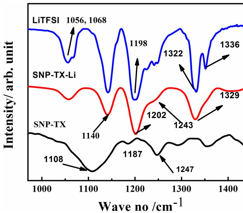
Fig. S4: FTIR spectra of SNP-TX, SNP-TX- Li and LiTFSI.
