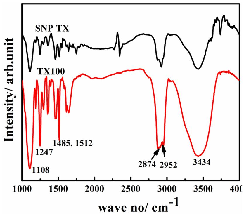
Fig. S3: FTIR spectra of SNP-TX and TX-100.
