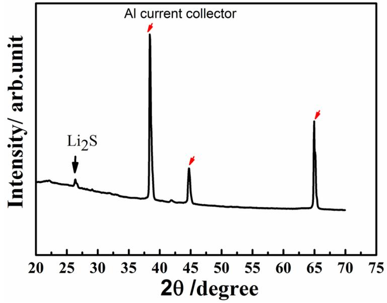
Fig. S10: Ex-situ XRD of S-MIEC after 10<sup>th</sup> cycle.
