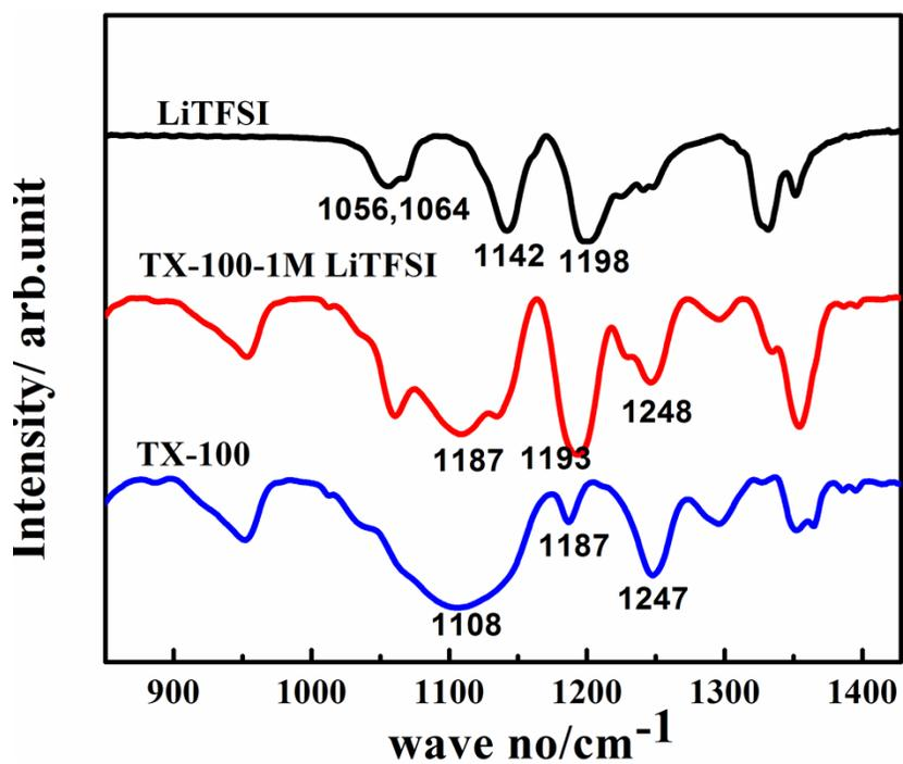
Fig. S5: IR spectrum of TX-100-LiTFSI (1 M).
