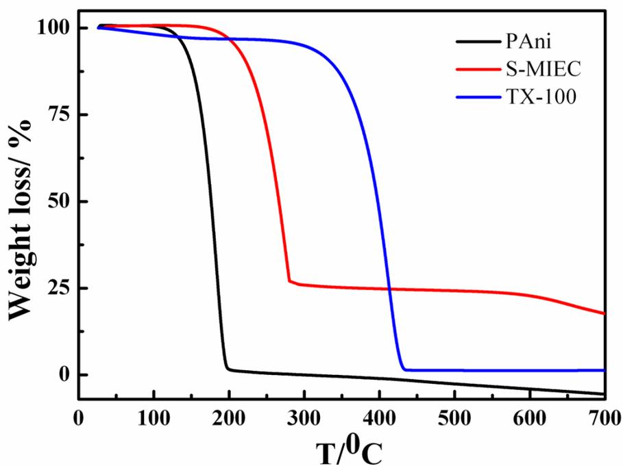
Fig. S1: Thermo gravimetric (TGA) analysis of S-MIEC.
