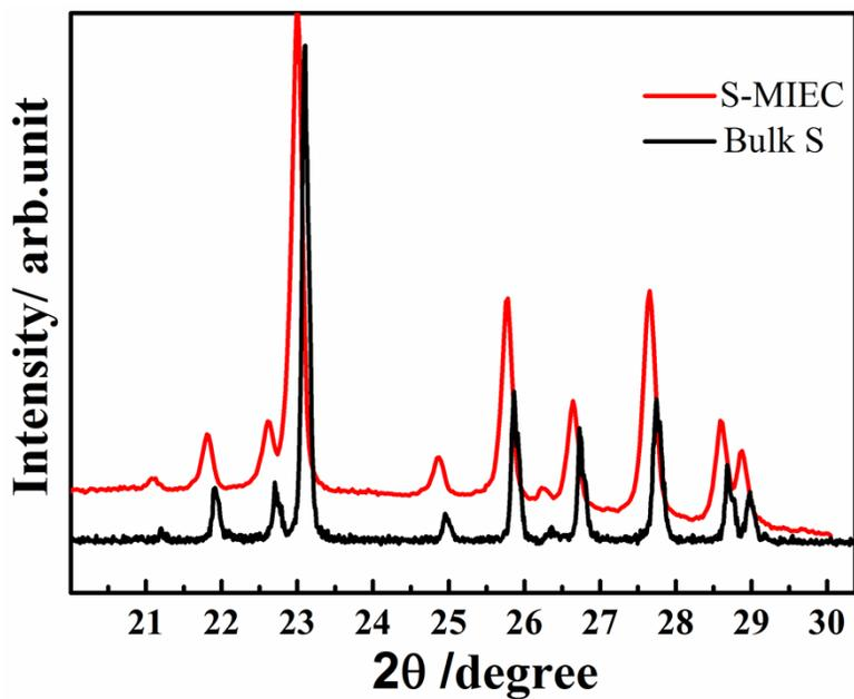
Fig. S2 (b): PXRD patterns of S-MIEC and bulk Sulfur.
