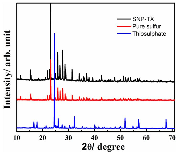
Fig. S2 (a): PXRD patterns of SNP –TX, thiosulfate and elemental sulfur.
