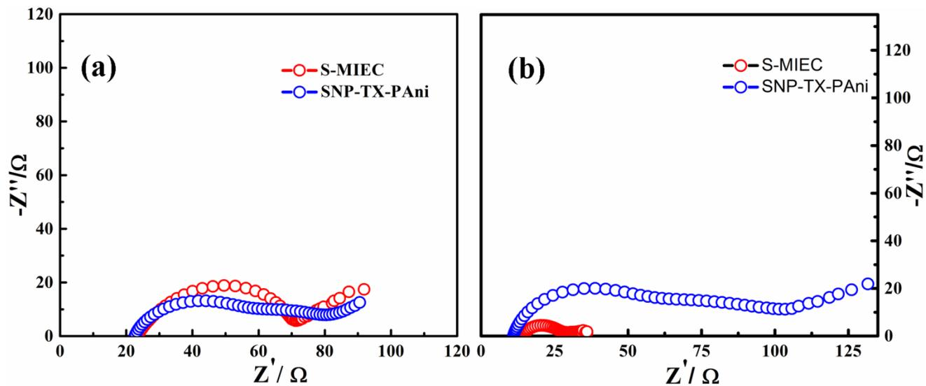
Fig. S9: EIS of Li-S-MIEC cell (a) before and (b) after  $10^{\text{th}}$  galvanostatic cycles.
