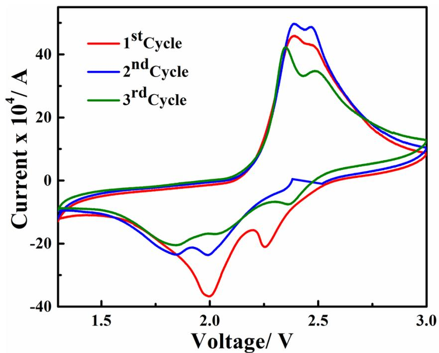
Fig. S8: Cyclic voltammogram of SNP-TX-PANI (at  $0.25 \text{ mV s}^{-1}$ ).
