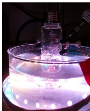
Figure S9. Photograph of the experimental set-up used to measure the generation of \text{MV}^{+\bullet} over time with LED illumination. The reaction vessel fitted with a septum cap was de-aerated with \text{N}_2 and placed in a water bath surrounded by white LED lights to help dissipate heat and act as a UV filter.
