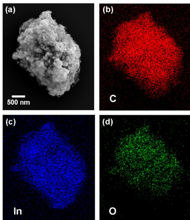
**Fig. S4** (a) SEM image of a piece of  $\text{In}_2\text{O}_3$ /carbon black, and elemental energy-dispersive X-ray (EDX) maps of (b) carbon, (c) indium and (d) oxygen, respectively.
