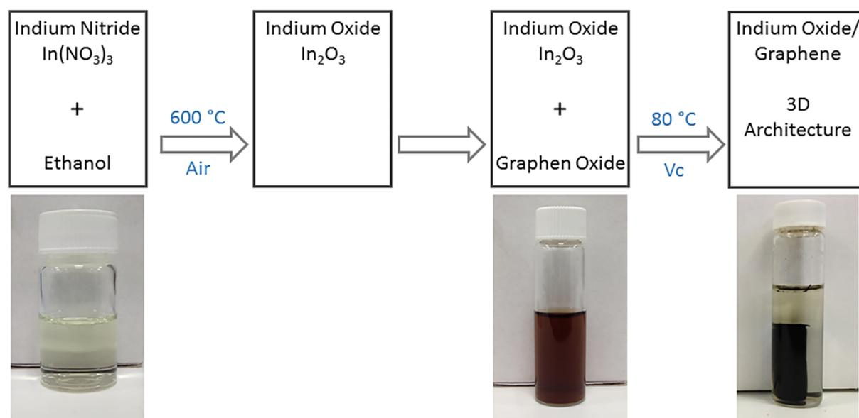
**Fig. S1** Schematic of the fabrication procedure and photos of products at different step including  $\text{In}(\text{NO}_3)_3$  in ethanol,  $\text{In}_2\text{O}_3$  NPs/graphene oxide solution and  $\text{In}_2\text{O}_3$ /graphene 3D architecture after reduction and self-assembly.
