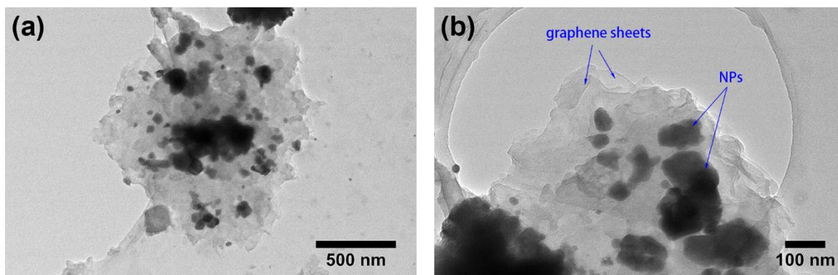
**Fig. S6** TEM images showing In<sub>2</sub>O<sub>3</sub>/graphene 3D architecture after 30 cycles.
