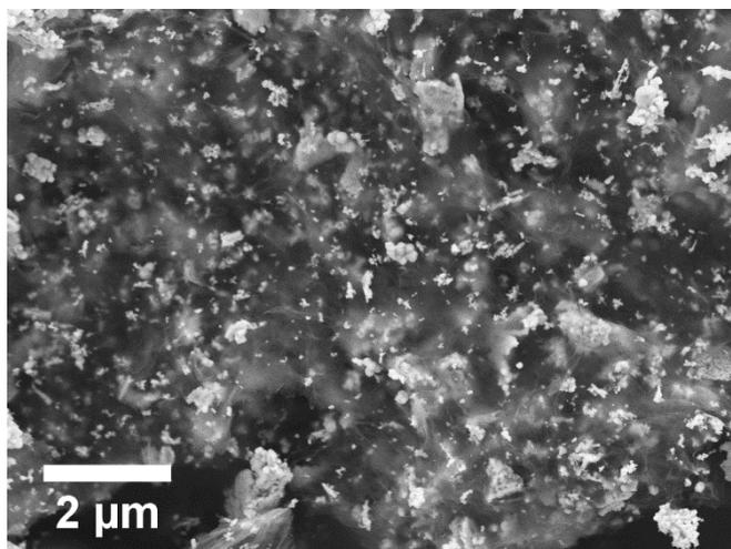
**Fig. S3** SEM image of the In<sub>2</sub>O<sub>3</sub>/graphene 3D architecture showing the dispersion of In<sub>2</sub>O<sub>3</sub> nanoparticles.
