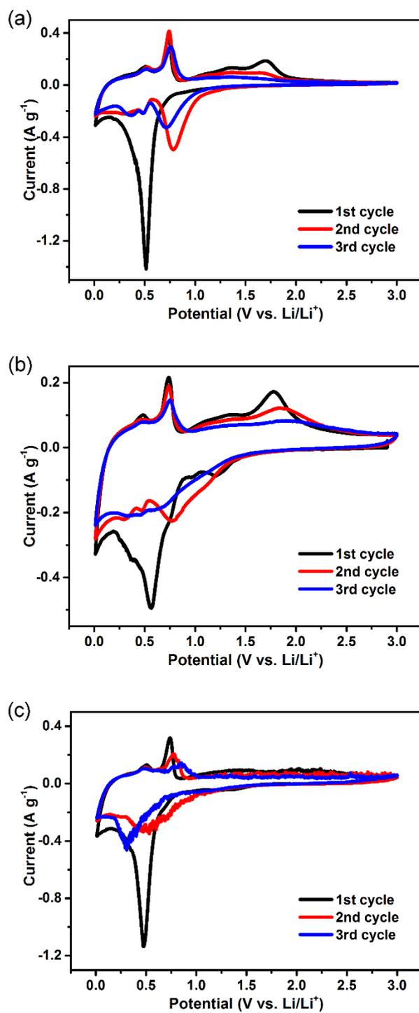
**Fig. S5** CV curves of the first three cycles of (a) pure  $\text{In}_2\text{O}_3$  NPs, (b)  $\text{In}_2\text{O}_3$ /carbon black composite, and (c)  $\text{In}_2\text{O}_3$ /graphene at a voltage range of 0.01 to 3.0 V and scan rate of  $0.1 \text{ mV s}^{-1}$ .
