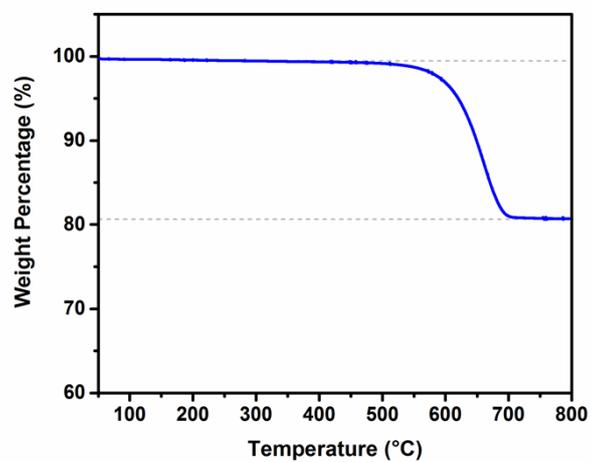
**Fig. S2** Thermogravimetric analysis results showing weight loss of the In<sub>2</sub>O<sub>3</sub>/graphene 3D architecture when heated in air flow from room temperature to 800 °C.
