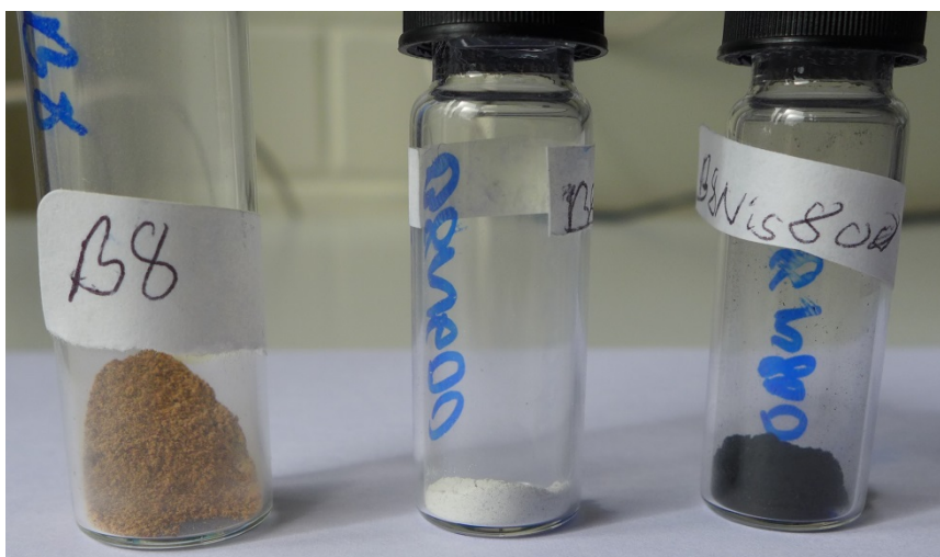
S.I.4. Photos of samples Left: as prepared T225 dried at 150°C. Middle: The T225 sample heated to 600°C in air. Right: the T225 sample with added NaOH heated to 800 °C in oxygen-deficient atmosphere during in situ diffraction.
