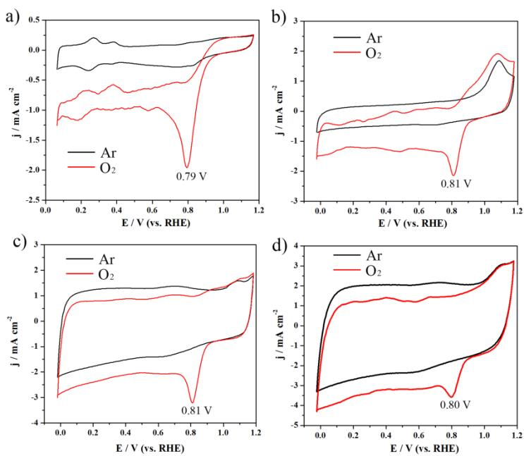
**Figure S4** Cyclic voltammogram (CV) curves of a) Pt/C, b) ZIF/rGO-700, c) ZIF/rGO-700-AL, d) ZIF-700-AL in Ar ( $\text{O}_2$ )-saturated 0.1 M KOH solution with a scan speed of 50 mV/s.
