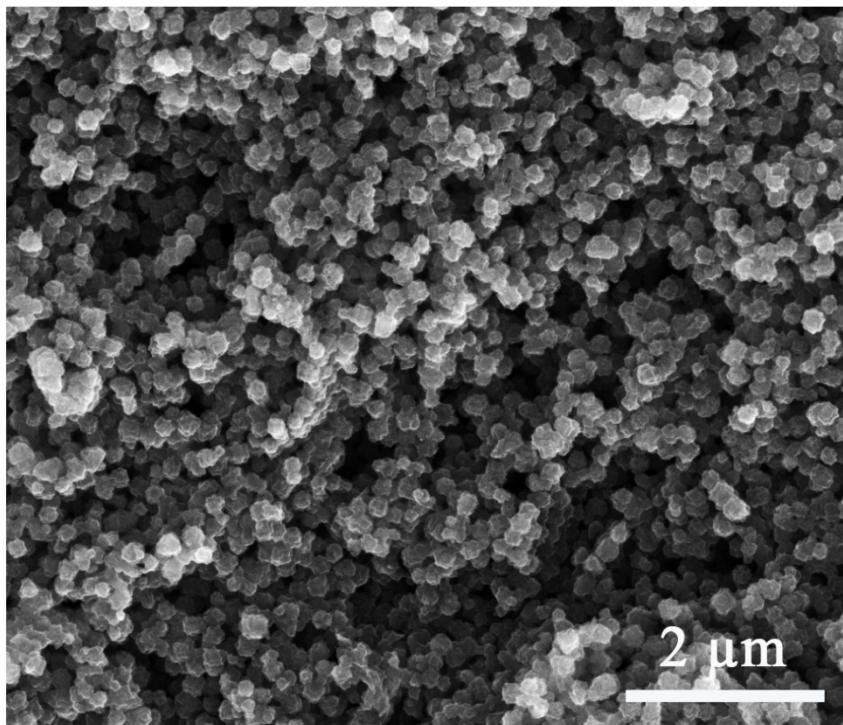
**Figure S2** SEM image of ZIF-700-AL prepared via carbonization of ZIF-67 at 700 °C in Ar followed by acid leaching. The SEM results show loosely packed nanoparticles.
