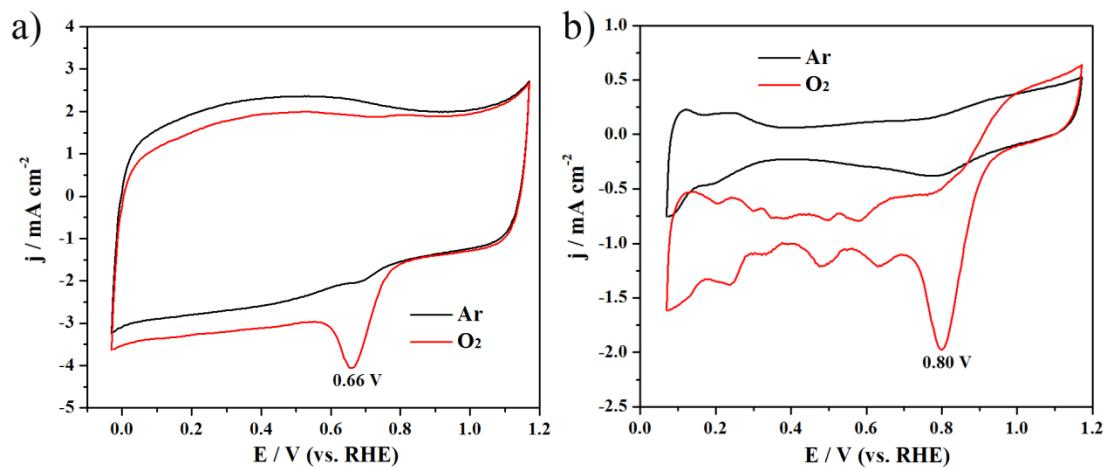
**Figure S5** CV curves of a) ZIF/rGO-700-AL and b) Pt/C in Ar ( $\text{O}_2$ )-saturated 0.1 M  $\text{HClO}_4$  solution with a scan speed of 50 mV/s.
