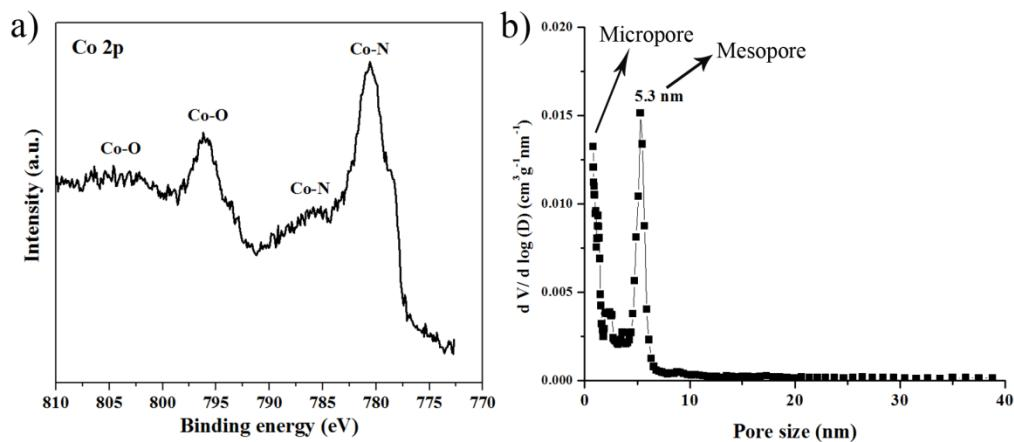
**Figure S3** a) High-resolution Co 2p spectra, b) DFT pore size distributions of ZIF/rGO-700-AL. The XPS data shows Co species exist with Co-N and Co-O bands, which is beneficial to ORR performance. DFT pore size distributions reveal the materials possess microporous and mesoporous structure.
