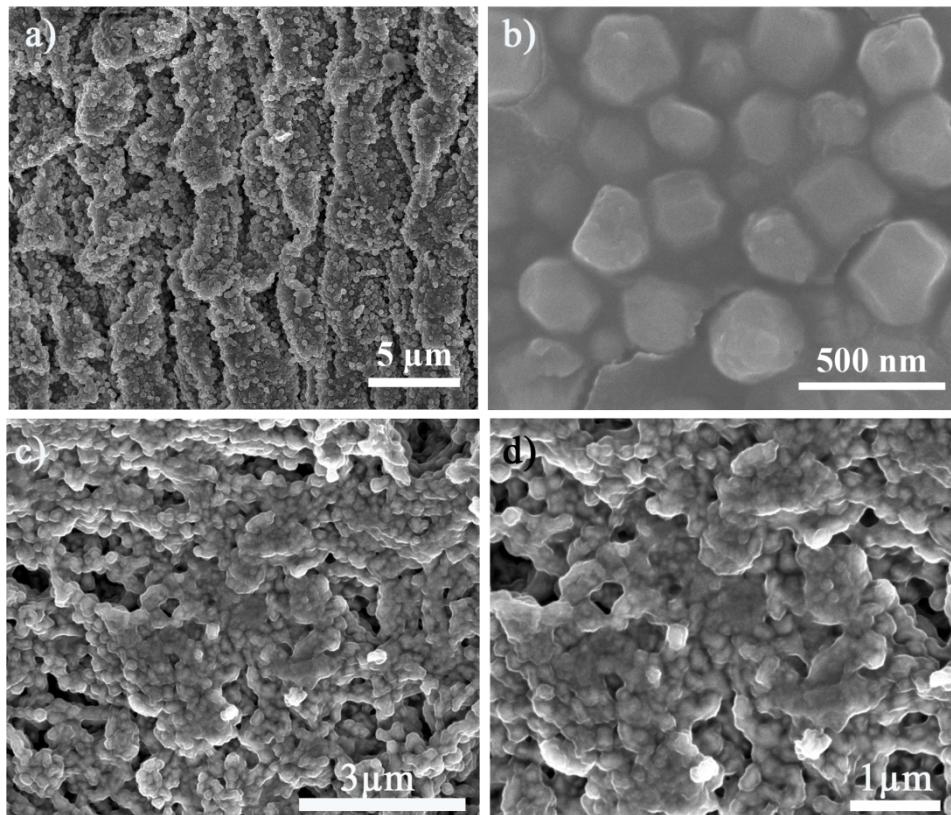
**Figure S1** SEM image of a, b) ZIF/GO-90 prepared by growing ZIF-67 nanocrystals on graphene oxide (GO) and drying at 90 °C in air; c, d) ZIF/rGO-500 prepared by carbonizing ZIF/GO materials at 500 °C for 3 h in Ar. The SEM images show the macroporous structure is produced as the shrinkage of ZIF and GO during carbonization process.
