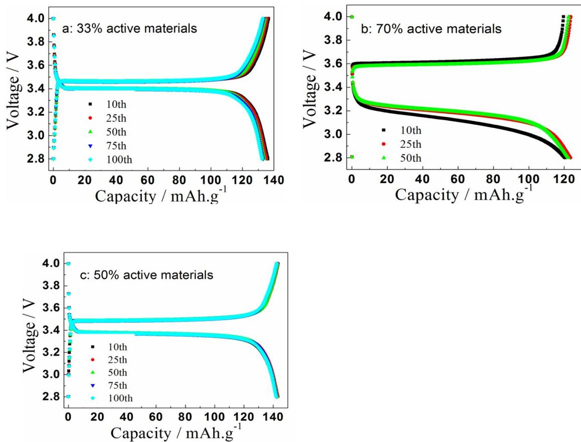
**Fig. S3. Additional Voltage profile with different binder contents:** Charge-discharge profiles of MME with different magnetic binder amount. The mass ratio of  $\text{LiFePO}_4\text{:Fe}_3\text{O}_4\text{:conductive agent}$  is 1:1:1 (a), 70:15:15(b), and 50:35:15(c).
