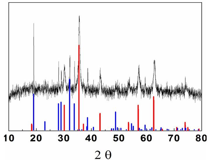
**Fig. S1. Phase purity characterization:** XRD patterns of the as-synthesized  $\text{Fe}_3\text{O}_4$ . (Red line: JCPDS card of 19-0629 as compound  $\text{Fe}_3\text{O}_4$ , Blue line: JCPDS card of 37-1465 as compound  $\text{Na}_2\text{SO}_4$ ).
