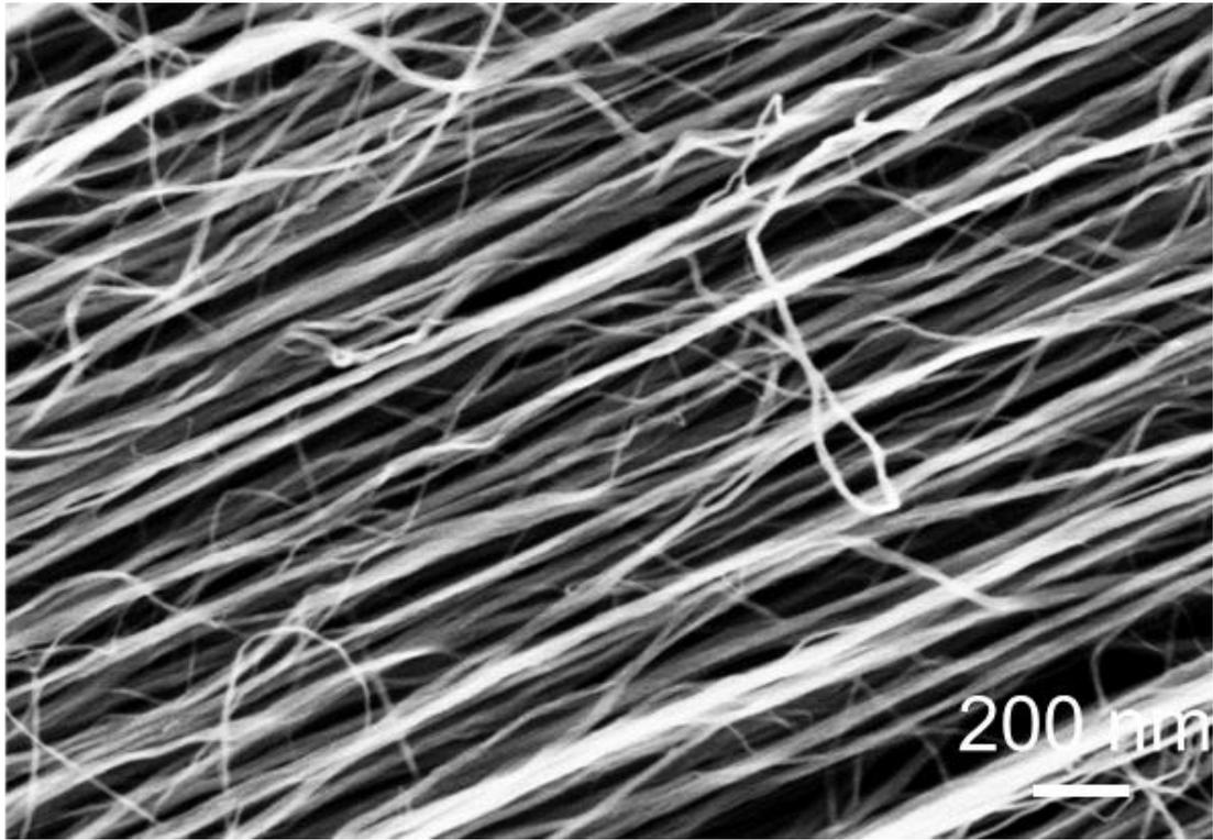
**Fig. S1** Scanning electron microscopy (SEM) image of the aligned CNT sheet.
