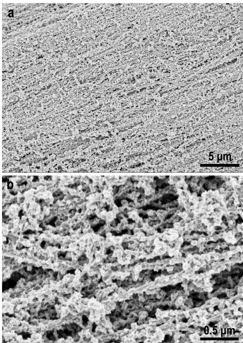
**Fig. S7** SEM images of the aligned CNT/MoS<sub>2</sub> hybrid fiber after bending for 1000 cycles. The top and bottom images show low and high magnifications, respectively.
