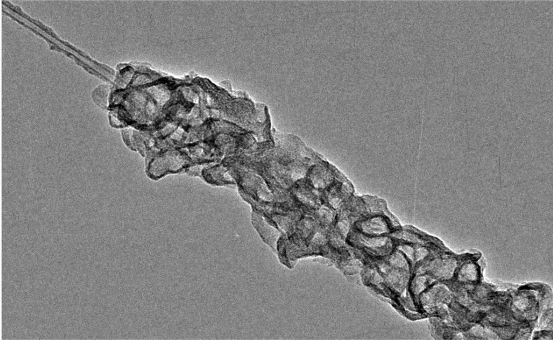
**Fig. S2** Transmission electron microscopy (TEM) image of a CNT wrapped by interwoven MoS<sub>2</sub> nanosheets.
