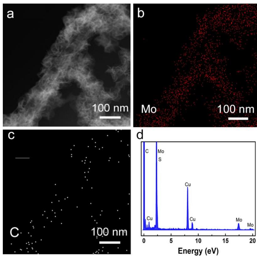
**Fig. S4** (a) Scanning transmission electron microscopy image of a CNT wrapped by interwoven MoS<sub>2</sub> nanosheets. (b-c) Energy dispersive X-Ray mapping of Mo and C. Mo and C are marked with red and white, respectively. L-alpha peak was used for Mo. (d) Energy dispersive X-Ray spectroscopy images of CNT/MoS<sub>2</sub> hybrid.
