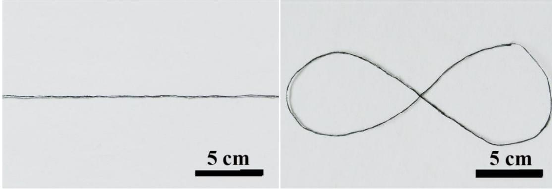
**Fig. S9** Photographs of flexible fibrous supercapacitors in different formats.
