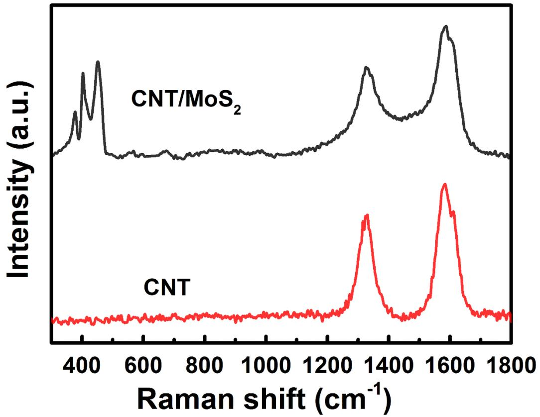
**Fig. S6** Raman spectra of the aligned CNT/MoS<sub>2</sub> hybrid fiber and bare CNT fiber.
