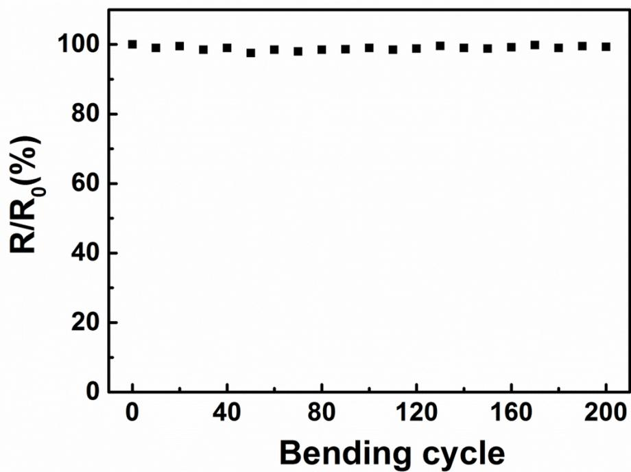
**Fig. S8** Resistance variation of the aligned CNT/MoS<sub>2</sub> hybrid fiber after bending with increasing cycles. R<sub>0</sub> and R represent the resistances before and after bending for different cycles, respectively.
