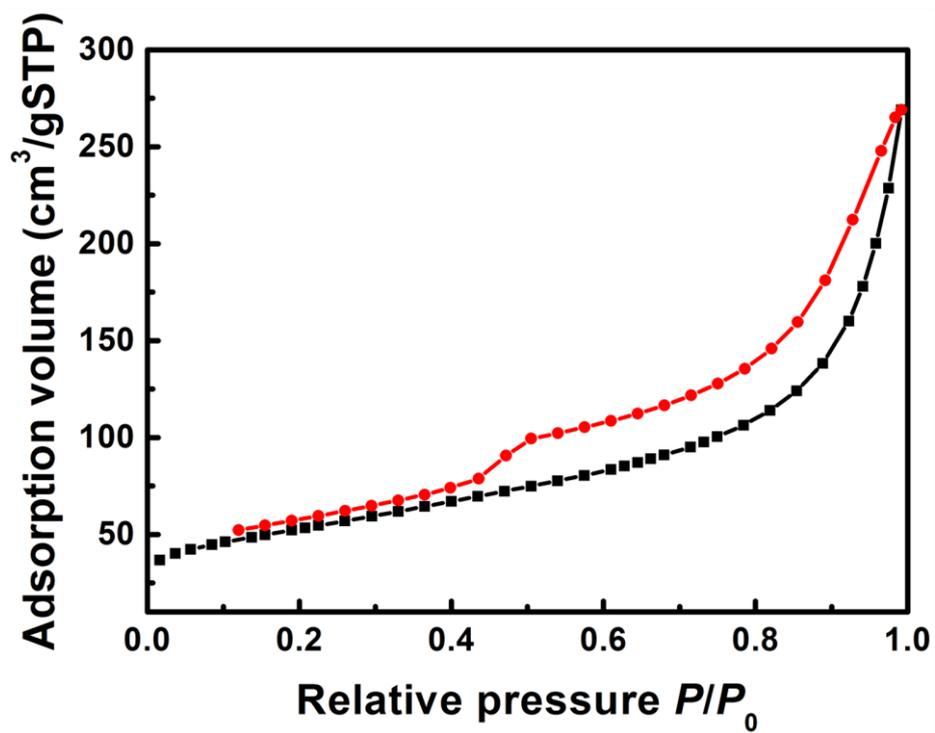
**Fig. S5** Nitrogen adsorption-desorption isotherms.  $P$  is the measured pressure within the adsorption bulb and  $P_0$  is the liquefaction pressure of the adsorbate.
