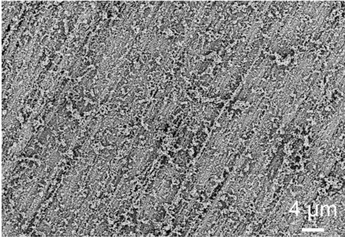
**Fig. S3** SEM image of the aligned CNT/MoS<sub>2</sub> hybrid sheet.
