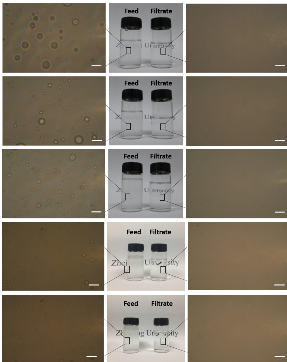
Figure S4. Separation results for various oil-in-water emulsions: hexane/water, octane/water, isopar G/water, SDS-assisted octane/water and SDS-assisted isopar G/water. All the filtrates become transparent and no droplet is observed in the corresponding optical image; scale bar=10 \mu\text{m} .
