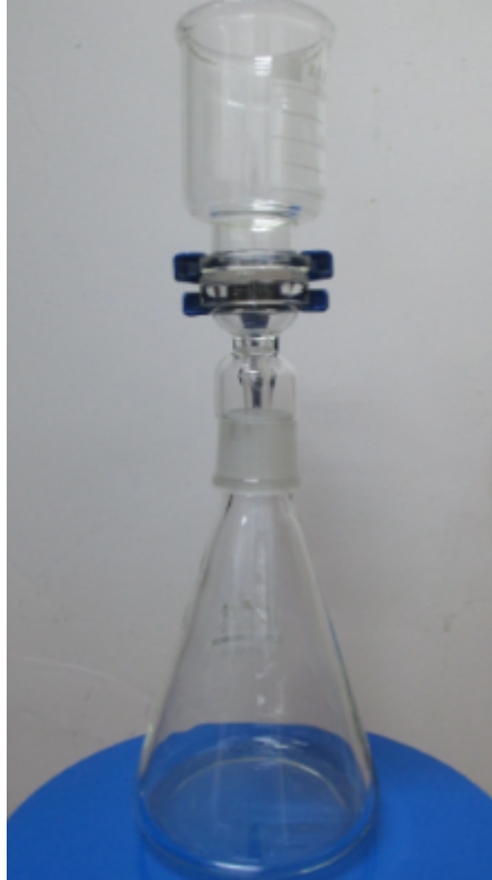
Figure S1. The gravity driven filtration apparatus used in this work.
