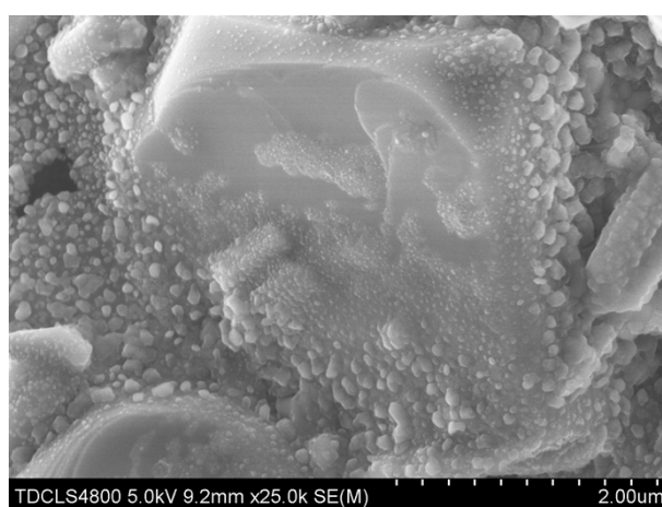
Fig. S1. SEM image of the calcined sample before washing, indicating the salt crystals with three kinds of length scales.
