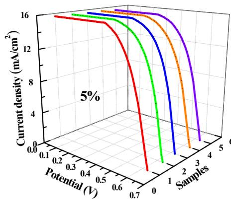
**Fig. S5.**  $J$ - $V$  curves of cell devices based on polysulfide electrolyte containing 5% (wt%) concentrations of PEG additive under the irradiation of AM 1.5G full one sun with 5 devices in parallel.
