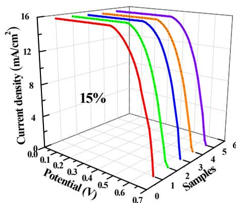
**Fig. S7.**  $J$ - $V$  curves of cell devices based on polysulfide electrolyte containing 15% (wt%) concentrations of PEG additive under the irradiation of AM 1.5G full one sun with 5 devices in parallel.
