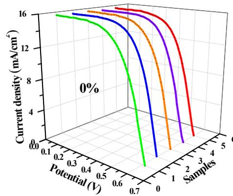
**Fig. S3.**  $J$ - $V$  curves of polysulfide electrolyte based cell devices under the irradiation of AM 1.5G full one sun with 5 devices in parallel.
