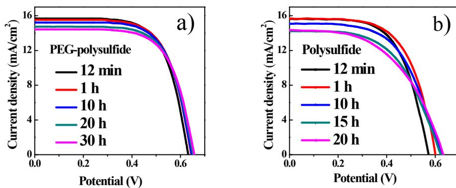
**Fig. S9.** Temporal evolution of  $J-V$  curves for cell devices based on PEG-polysulfide electrolyte (a), and polysulfide electrolyte (b) under the continuous irradiation by an AM 1.5 G solar simulator with intensity of  $100 \text{ mW}/\text{cm}^2$  at room temperature.
