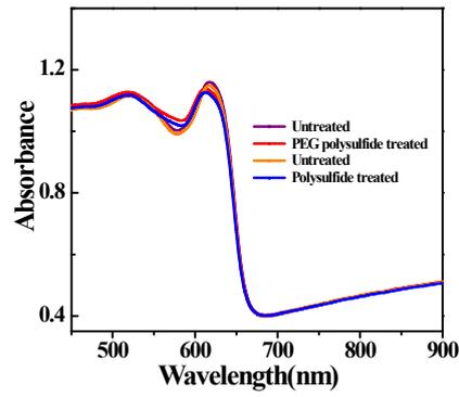
**Fig. S2.** Absorption spectra of the CdSe QDs films before and after with polysulfide electrolyte with (red) and without (blue) 15 wt% PEG additives treatment.
