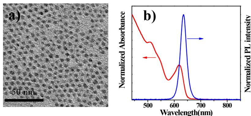
**Fig. S1.** TEM image (a) and UV-vis absorption (red line) and PL emission (blue line,  $\lambda_{\text{ex}} = 410$  nm) spectra of pre-synthesized oil-soluble CdSe QDs.
