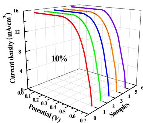
**Fig. S6.**  $J$ - $V$  curves of cell devices based on polysulfide electrolyte containing 10% (wt%) concentrations of PEG additive under the irradiation of AM 1.5G full one sun with 5 devices in parallel.
