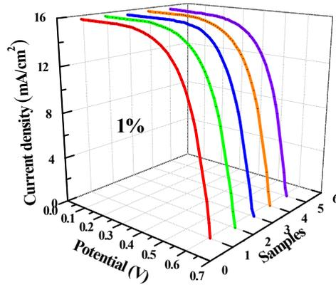
**Fig. S4.**  $J$ - $V$  curves of cell devices based on polysulfide electrolyte containing 1% (wt%) concentrations of PEG additive under the irradiation of AM 1.5G full one sun with 5 devices in parallel.
