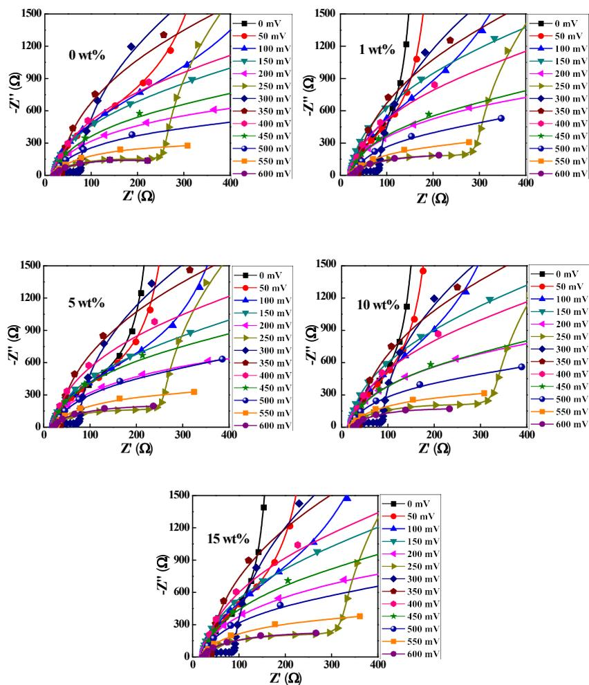
**Fig. S8.** Nyquist plots for polysulfide electrolyte containing different concentrations of PEG additives based cell devices under different forward bias voltages.
