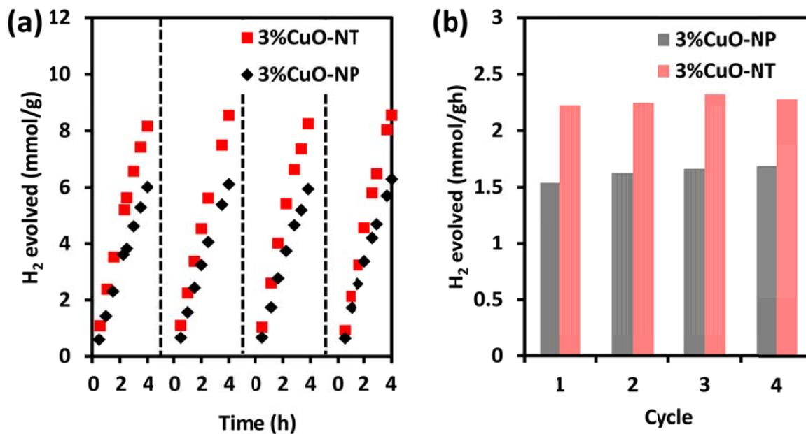
Figure S5 (a) Amount of H<sub>2</sub> evolved for cyclic stability test under Xe irradiation, measured for 4 cycles. (b) Initial rates of H<sub>2</sub> evolution for cyclic stability test of 3%CuO-NP and 3%CuO-NT
