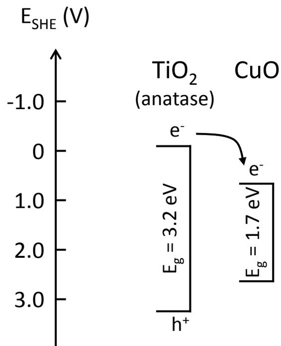
Figure S1 Schematic diagram showing the energy band positions of TiO<sub>2</sub>, CuO with respect to standard hydrogen electrode (SHE) at pH 1, and transfer of electron from the conduction band of TiO<sub>2</sub> to CuO. The  $E_{\text{CB}}$  of TiO<sub>2</sub> (anatase) is -0.25 V vs SHE<sup>1</sup>, and the  $E_{\text{CB}}$  of CuO is 0.96 V vs SHE<sup>2</sup>.
