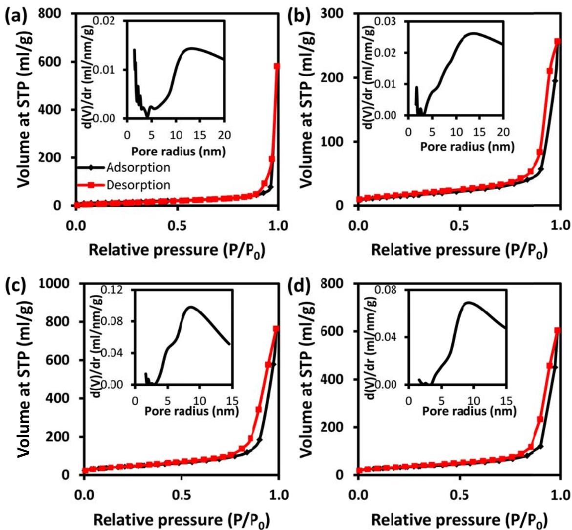
Figure S2 Nitrogen adsorption/desorption isotherms of (a) NP, (b) 3% CuO-NP, (c) NT and (d) 3% CuO-NT with (insets) corresponding BJH pore size distribution.
