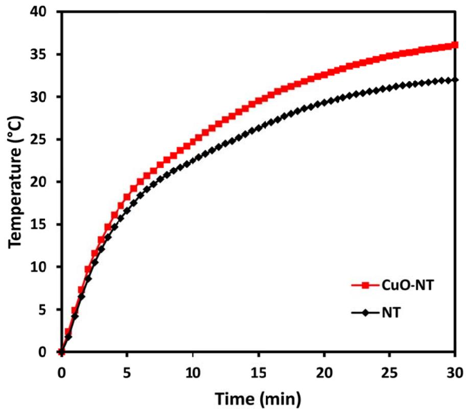
Figure S3 Temperature measurement of NT and CuO-NT in 20% vol glycerol solution under Xe Lamp illumination at  $1000\text{W}/\text{m}^2$ .
