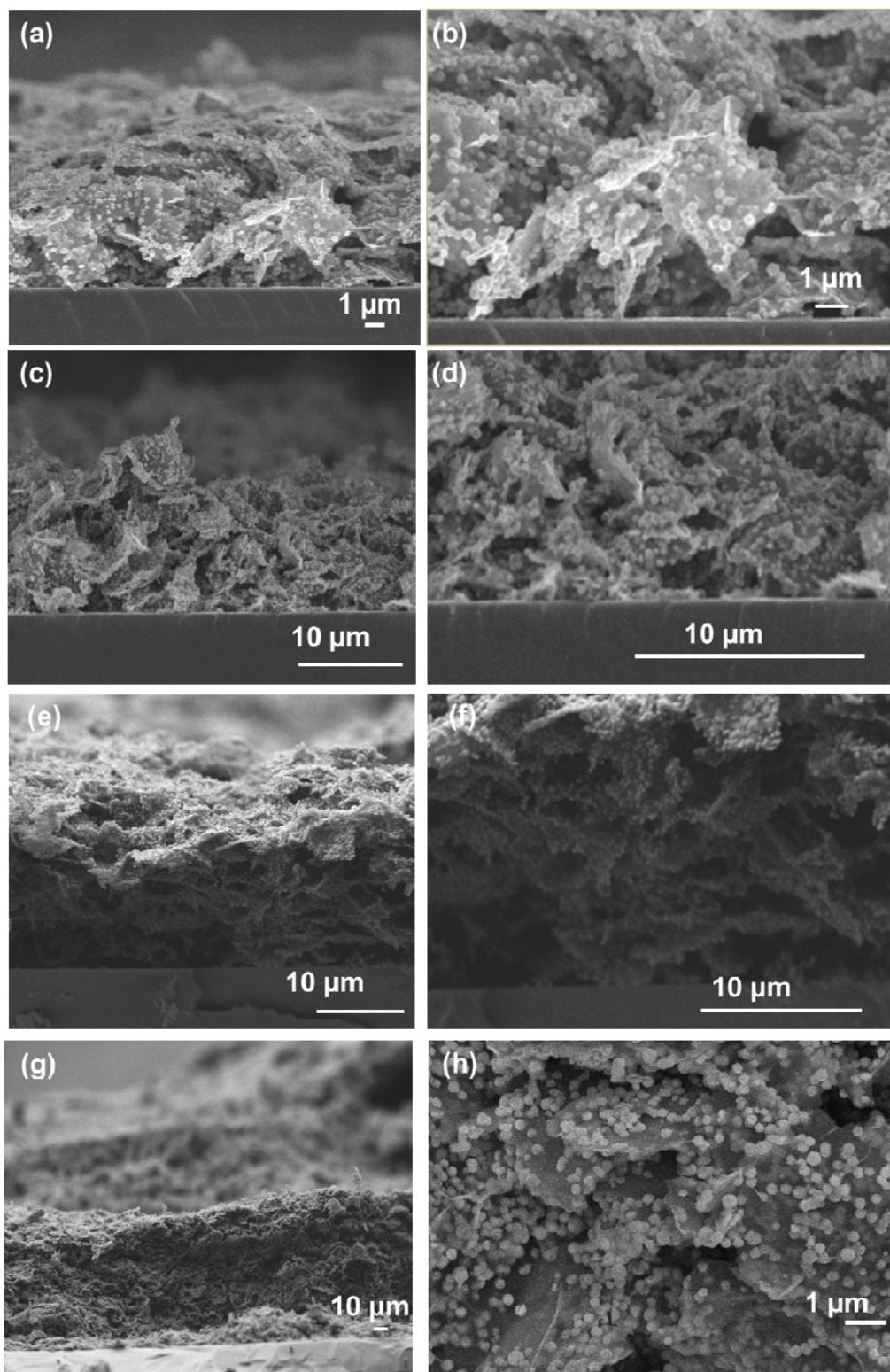
**Fig. S5.** Typical SEM images of the cross-sectional view of  $(\text{Fe}_3\text{O}_4@\text{FLG}/\text{PEDOT:PSS}_2)_n$  hybrid architectures for (a, b)  $n = 15$  bilayers (thickness estimated at  $9 \mu\text{m}$ ), (c, d)  $n = 20$  bilayers (thickness estimated at  $12 \mu\text{m}$ ), (e, f)  $n = 30$  bilayers (thickness estimated at  $17 \mu\text{m}$ ) and (g, h)  $n = 120$  bilayers (thickness estimated at  $72 \mu\text{m}$ ).
