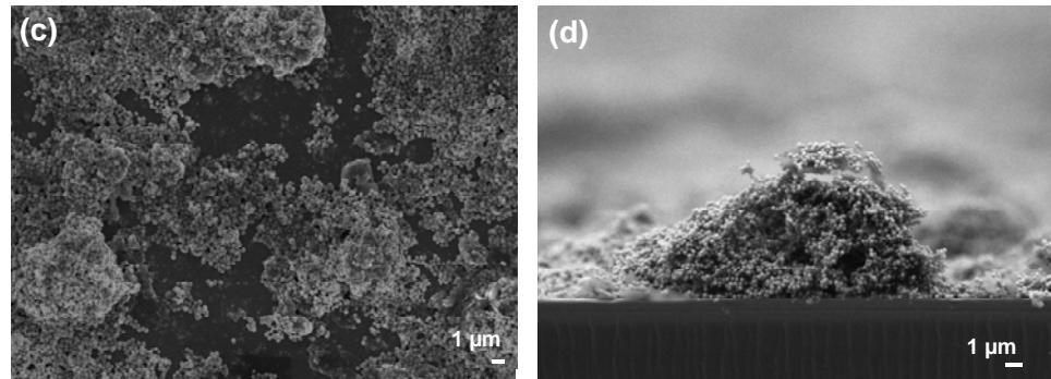
**Fig. S7.** Typical SEM images of the top and the cross-sectional view of the (a, b) grafted  $(\text{Fe}_3\text{O}_4@\text{FLG} / \text{PEDOT:PSS})_{15}$  and (c, d) ungrafted  $(\text{FLG}/\text{Fe}_3\text{O}_4/\text{PEDOT:PSS})_{15}$  hybrid architectures.
