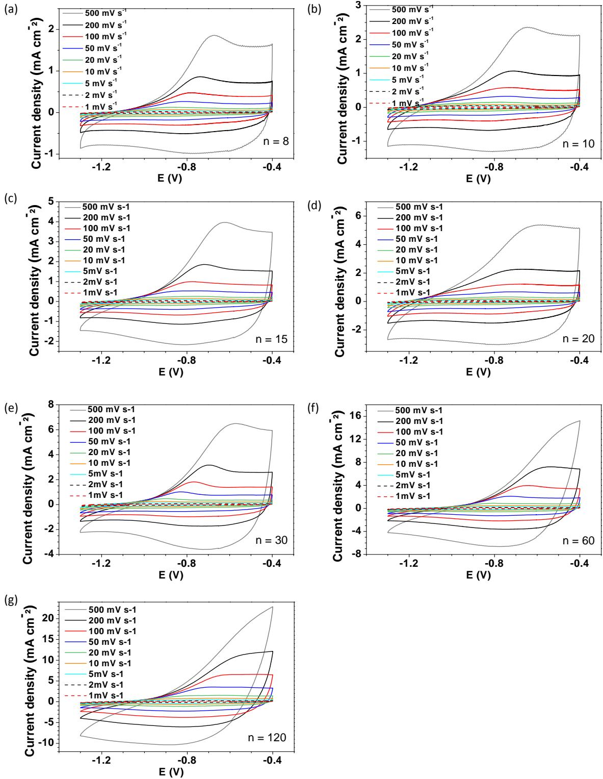
**Fig. S8.** Voltamograms of  $(\text{Fe}_3\text{O}_4@\text{FLG}/\text{PEDOT:PSS})_n$  hybrid architecture recorded at different scan rates from 1 to  $500 \text{ mV s}^{-1}$  for (a)  $n = 8$  bilayers, (b)  $n = 10$  bilayers, (c)  $n = 15$  bilayers, (d)  $n = 20$  bilayers, (e)  $n = 30$  bilayers, (f)  $n = 60$  bilayers and (g)  $n = 120$  bilayers.
