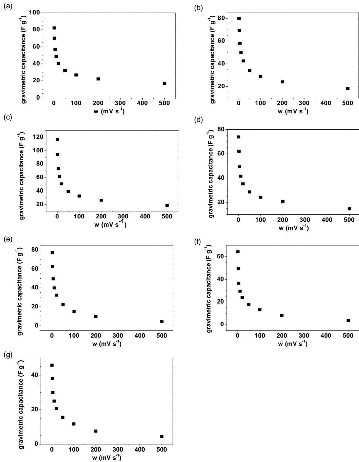
**Fig. S10.** Gravimetric capacitance of  $(\text{Fe}_3\text{O}_4@\text{FLG /PEDOT:PSS})_n$  hybrid architecture as a function of scan rate recorded with a potential range between -1.3 and -0.4 V for (a)  $n = 8$  bilayers, (b)  $n = 10$  bilayers, (c)  $n = 15$  bilayers, (d)  $n = 20$  bilayers, (e)  $n = 30$  bilayers, (f)  $n = 60$  bilayers and (g)  $n = 120$  bilayers.
