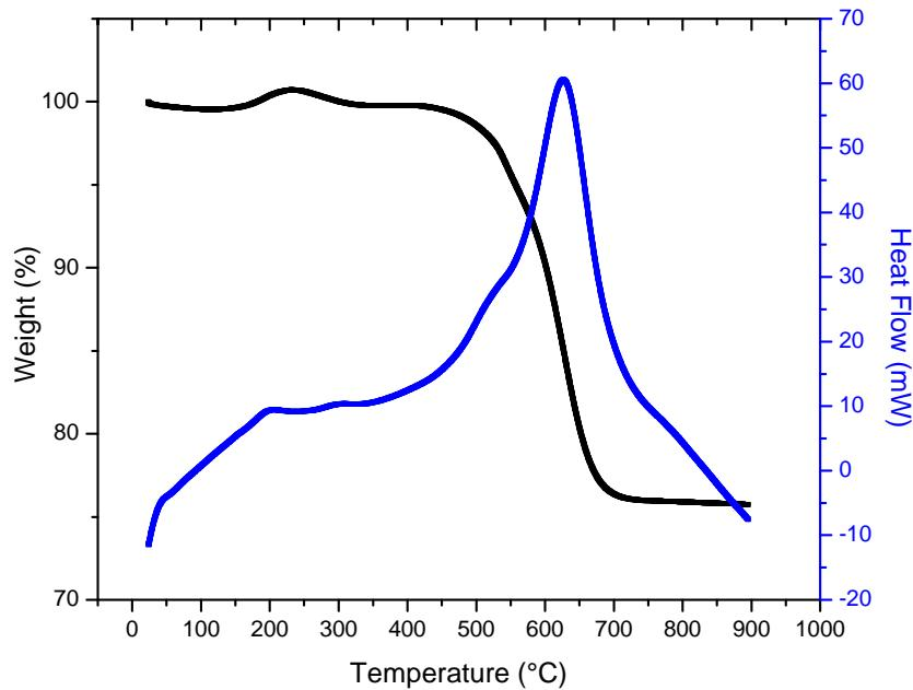
**Fig. S2.** Thermogram of iron oxide nanostructures on graphene (Fe<sub>3</sub>O<sub>4</sub>@FLG) carried out in air atmosphere.
