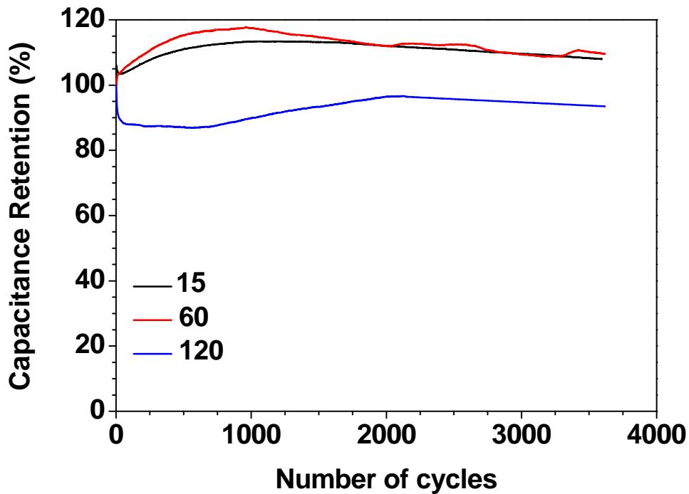
**Fig. S11.** Capacitance retention (%) as a function of number of cycles of  $(\text{Fe}_3\text{O}_4@\text{FLG}/\text{PEDOT:PSS})_n$  hybrid architecture for different number of bilayers ( $n$ ).
