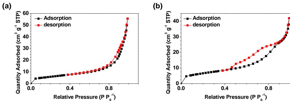
**Fig. S1.** N<sub>2</sub> adsorption-desorption isotherms of (a) Fe<sub>3</sub>O<sub>4</sub> nanostructures and (b) Fe<sub>3</sub>O<sub>4</sub>@FLG composites.
