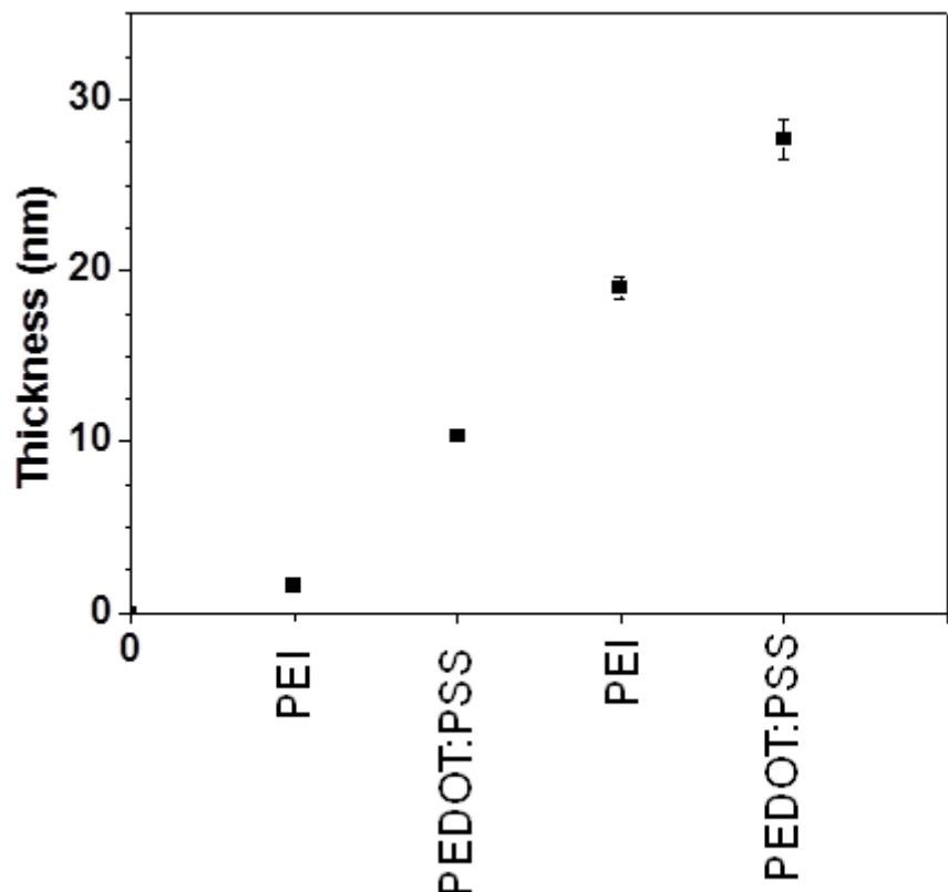
**Fig. S3.** Evolution of the thickness of  $(\text{PEI}/\text{PEDOT:PSS})_2$ , measured by ellipsometry, as a function of the last deposited layer.
