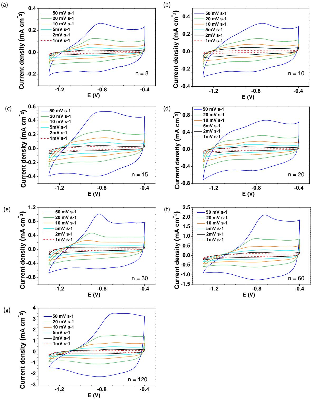
**Fig. S9.** Voltamogramms of  $(\text{Fe}_3\text{O}_4@\text{FLG}/\text{PEDOT:PSS})_n$  hybrid architecture recorded at different scan rates from 1 to  $50 \text{ mV s}^{-1}$  for (a)  $n = 8$  bilayers, (b)  $n = 10$  bilayers, (c)  $n = 15$  bilayers, (d)  $n = 20$  bilayers, (e)  $n = 30$  bilayers, (f)  $n = 60$  bilayers and (g)  $n = 120$  bilayers.
