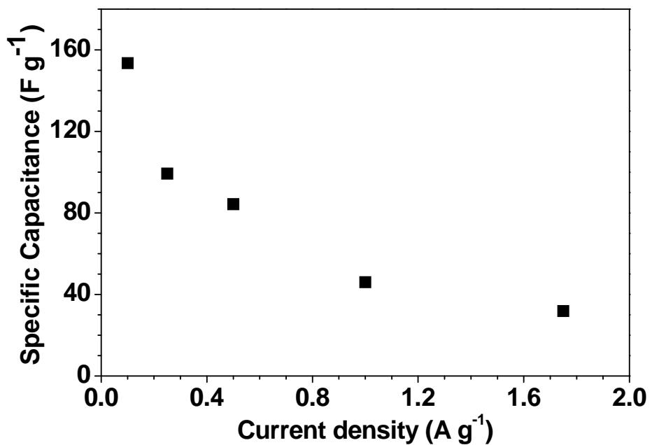
**Fig. S12.** Specific capacitance of  $(\text{Fe}_3\text{O}_4@\text{FLG}/\text{PEDOT:PSS})_{15}$  hybrid architecture at various discharge current densities.
