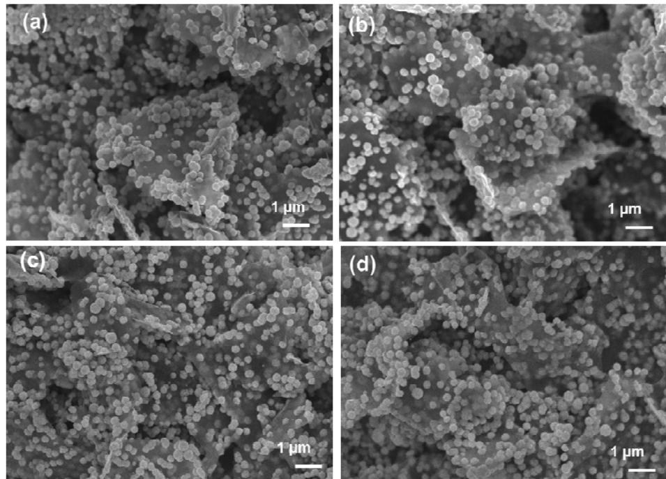
**Fig. S4.** Typical SEM images of the top view of  $(\text{Fe}_3\text{O}_4@\text{FLG}/\text{PEDOT:PSS})_n$  hybrid architecture for (a)  $n = 15$  bilayers, (b)  $n = 20$  bilayers, (c)  $n = 30$  bilayers and (d)  $n = 120$  bilayers.
