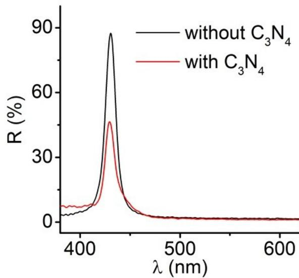
**SI Figure 3.** Reflection spectrum of SiO<sub>2</sub>/ETPTA photonic crystal film with and without the loading of meso-C<sub>3</sub>N<sub>4</sub> nanorods.
