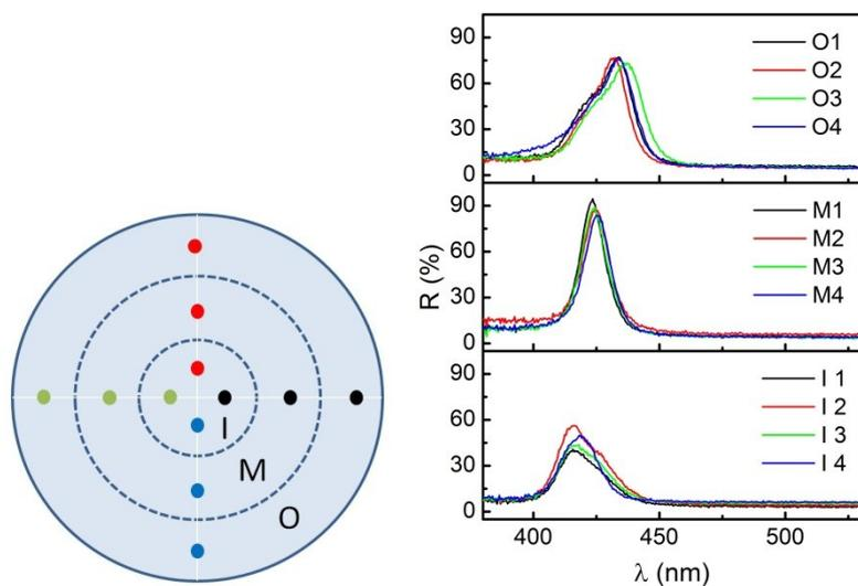
**SI Figure 1.** Reflection spectrum measured in the inner (I), middle (M) and outer (O) region of the SiO<sub>2</sub>/ETPTA photonic crystal film. As shown in the left scheme, 4 points are tested in each group and their reflection spectra are very close.
