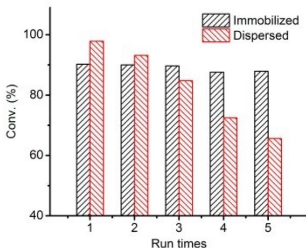
**SI Figure 5.** Comparison of photocatalytic activity for immobilized and dispersed meso-C<sub>3</sub>N<sub>4</sub> in 5 successive 60-min degradation of RhB.
