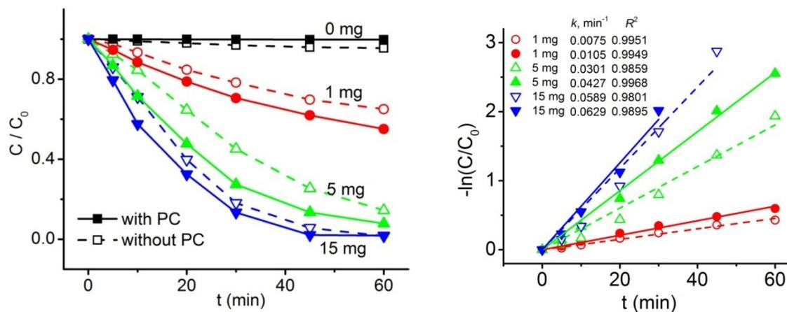
**SI Figure 4.** Comparison of photodegradation efficiency when the catalysts are supported by pure ETPTA film (dash line) and SiO<sub>2</sub>/ETPTA photonic crystal film (solid line). The catalysts dosage is set to be 0, 1, 5 and 15 mg, respectively.
