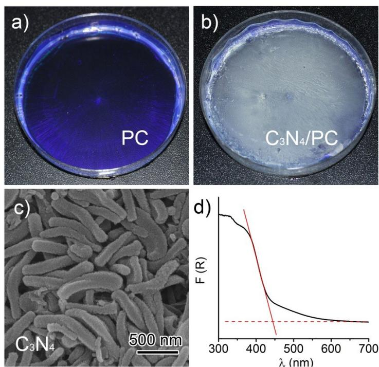
**SI Figure 2.** Digital photos of (a) SiO<sub>2</sub>/ETPTA photonic crystal film and (b) meso-C<sub>3</sub>N<sub>4</sub> loaded PC film. (c) SEM image and (d) UV-Vis diffuse reflectance spectrum of meso-C<sub>3</sub>N<sub>4</sub> nanorods photocatalyst.
