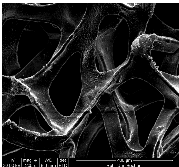
Figure S3. SEM image of nickel oxalate nanosheets decorated 3D nickel foam at low magnification.
