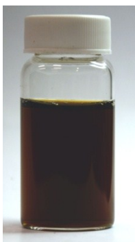
Figure S1. Digital image of the TEA/GO aqueous dispersion (same concentration as the reaction condition).
