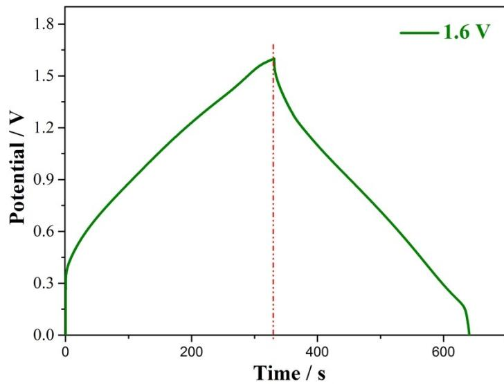
**Figure S13** The galvanostatic charge–discharge curves at a current of 5 mA under a potential of 1.6 V in 2 M KOH solution.
