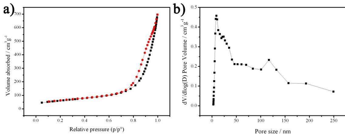
**Figure S4** (a) Nitrogen adsorption and desorption isotherms and (b) the corresponding pore-size distribution calculated by BJH method from the desorption branch of hierarchical NCMNT-3.
