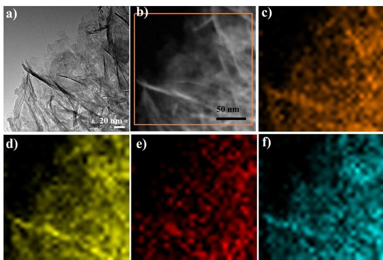
**Figure S3** a) TEM image, b) STEM image, c) Mo mapping, d) Ni mapping, e) Co mapping, and f) O mapping.
