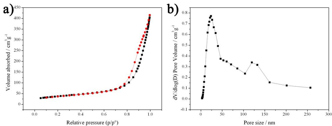
**Figure S8** (a) Nitrogen adsorption and desorption isotherms and (b) the corresponding pore-size distribution calculated by BJH method from the desorption branch of hierarchical NCMNT-2.
