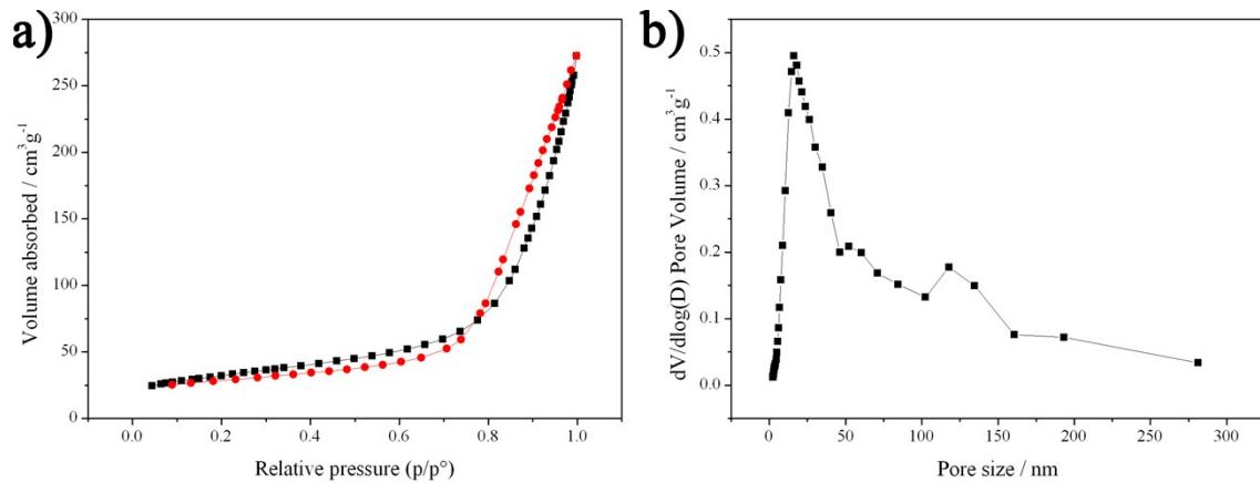
**Figure S7** (a) Nitrogen adsorption and desorption isotherms and (b) the corresponding pore-size distribution calculated by BJH method from the desorption branch of hierarchical NCMNT-1.
