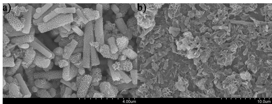
**Figure S9** (a) SEM image of the sample obtained as the added weight of cobalt chloride was 95 mg and (b) SEM image of the sample obtained as the added weight of cobalt chloride was 590 mg.
