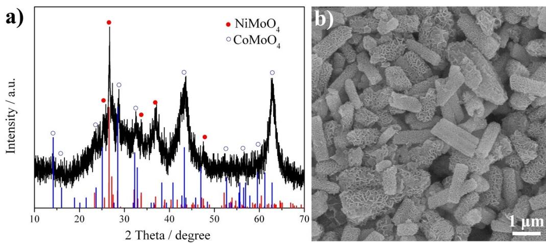
**Figure S11** a) XRD and b) SEM image of the sample obtained as cobalt chloride was replaced with cobalt acetate. The experimental conditions are similar to those of synthesis of NCMNT-3, but cobalt chloride was replaced with cobalt acetate (the molar quantity molar 68 mg).
