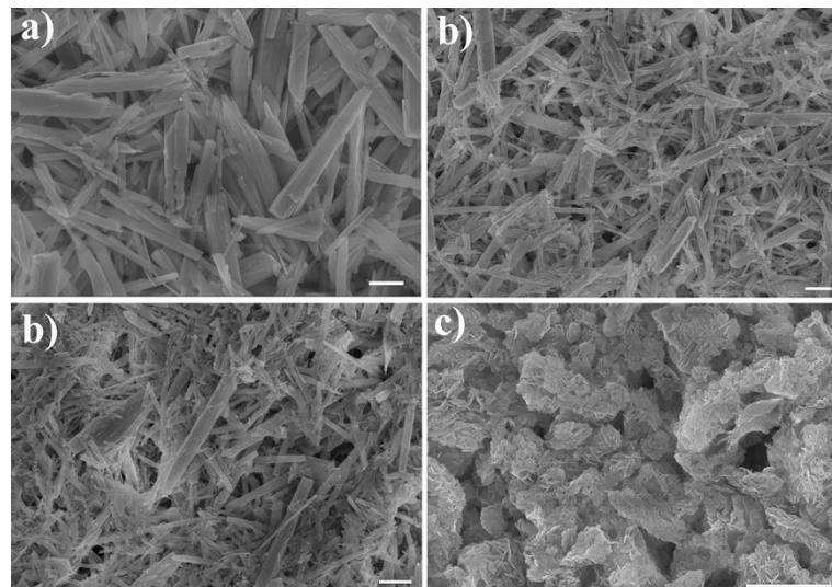
**Figure S12** SEM image of the samples obtained using MoO<sub>3</sub> nanorods and cobalt acetate as precursors in the water–ethanol (volume ratio = 1: 1) system and the hydrothermal treatment proceeded at 90°C for 5 h. a) Weight of cobalt acetate is 68 mg, b) weight of cobalt acetate is 78 mg, c) weight of cobalt acetate is 78 mg, and d) weight of cobalt acetate is 620 mg. The scar bars: 2 μm.
