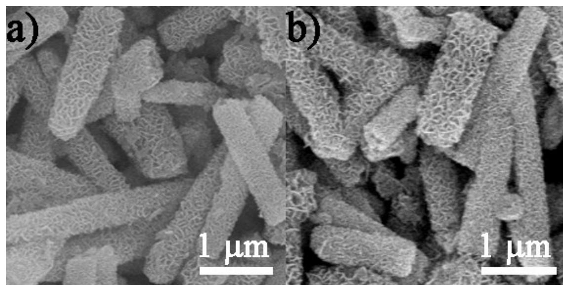
**Figure S6** SEM images of the hierarchical nanosheet-based nanotubes with different added weight of cobalt chloride. (a) NCMNT-1 and (b) NCMNT-2.
