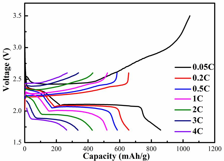
**Figure S6.** Voltage-capacity profiles of the top current collector cell with  $\text{Li}_2\text{S}@\text{C}$  cathode at various discharge/charge current rates.
