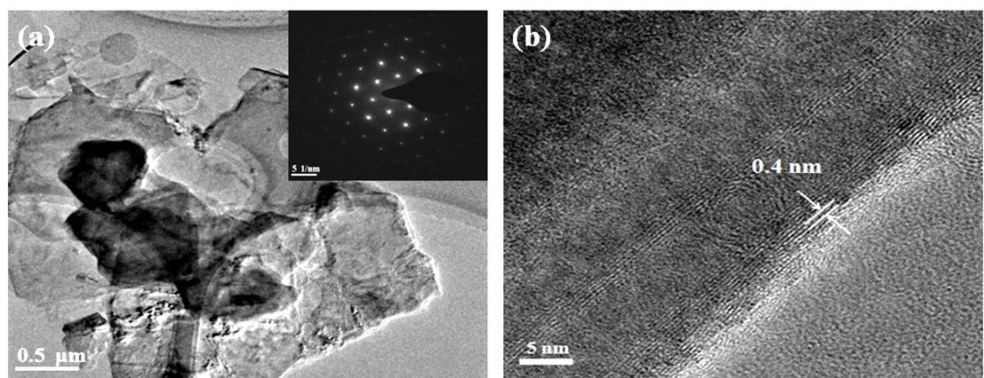
**Figure S3.** (a) A representative FETEM image of  $C_{AG}$  and SAED pattern of  $C_{AG}$ ; (b) HRTEM image of  $C_{AG}$ .
