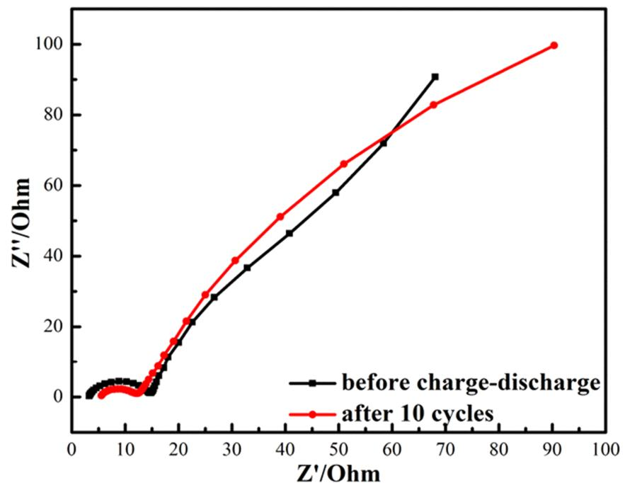
**Figure S5.** Electrochemical impedance spectra of  $\text{Li}_2\text{S}@\text{C}$  composites with N-CNT top current collector.
