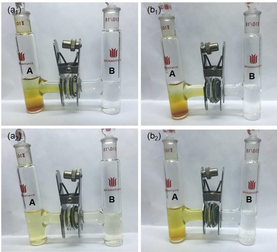
**Figure S4.** Photos of the H-type glass containers with “side A” containing electrolyte with Li<sub>2</sub>S<sub>8</sub> and “side B” containing pure electrolyte: (a<sub>1</sub>) pure separator at 0 min; (a<sub>2</sub>) pure separator after 20h; (b<sub>1</sub>) pure separator with N-CNT film at 0 min; (b<sub>2</sub>) pure separator with N-CNT film after 20 h.
