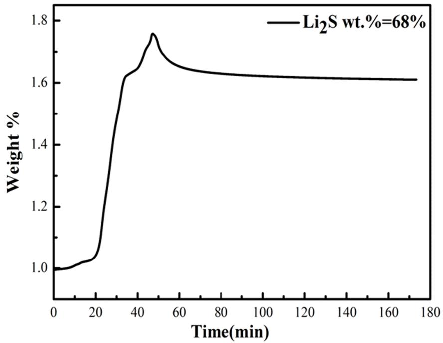
**Figure S1.** TGA curve of Li<sub>2</sub>S@C composites heating in air.
