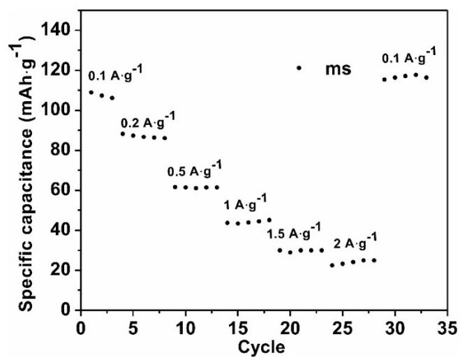
Fig. S3 Rate performance of mesoporous silica.
