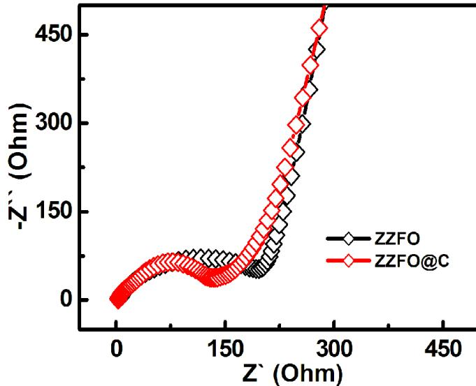
**Fig. S10.** EIS spectra of the ZZFO@C and ZZFO anodes at an open circuit voltage state using fresh cells as indicated
