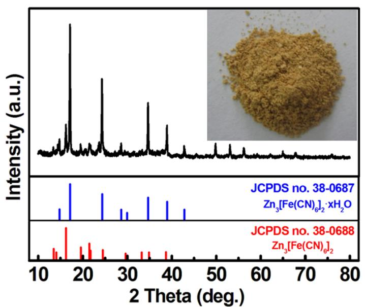
**Fig. S1.** Wide-angle XRD pattern and typical optical image (the inset) of the resulting ZFC
