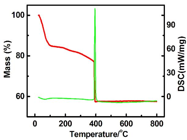
**Fig. S2.** TG data for the precursor of ZFC
