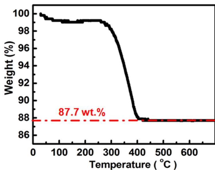
**Fig. S4.** TG analysis of the core-shell ZZFO@C under air flow with a temperature ramp of  $10\text{ }^{\circ}\text{C min}^{-1}$
