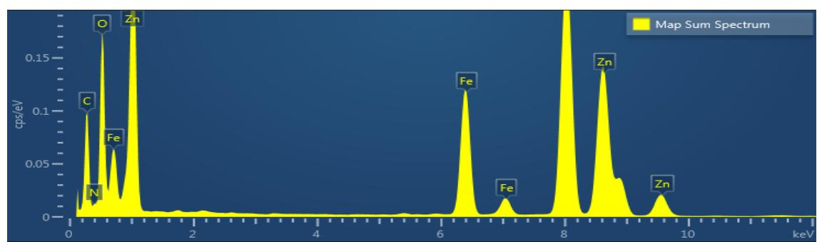
**Fig. S8.** EDXA spectrum of the as-synthesized core-shell ZZFO@C
