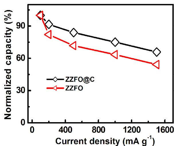
**Fig. S9.** Normalized capacity at each current step (Fig. 6c) by the average capacity under a current rate of 100 mA g<sup>-1</sup> of the initial step
