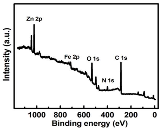
**Fig. S6.** Overview survey XPS spectrum of the as-prepared ZFC precursor
