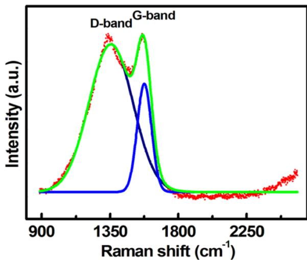
**Fig. S5.** Raman spectrum of the as-prepared core-shell ZZFO@C
