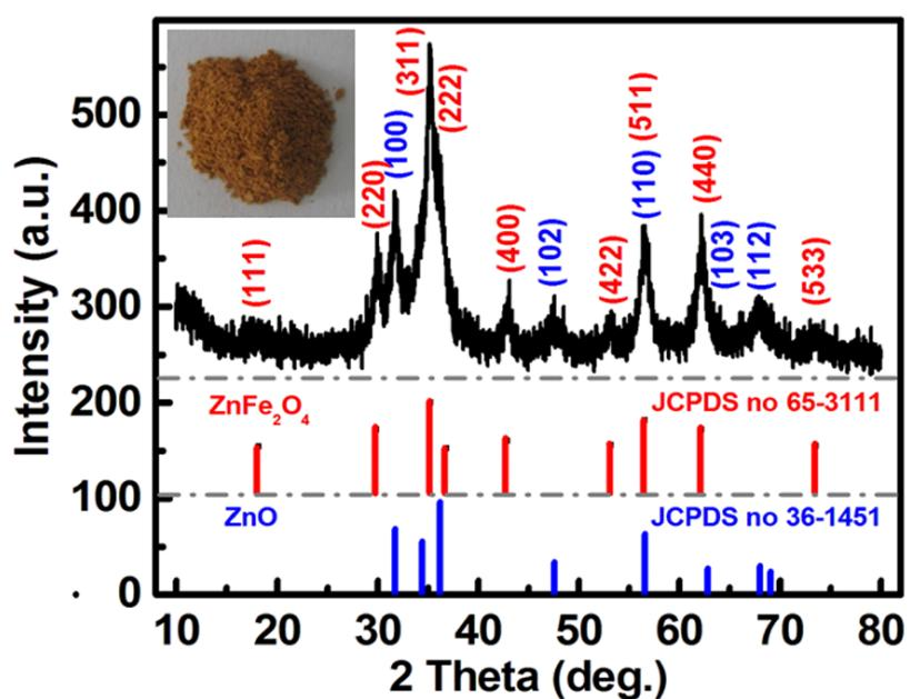
**Fig. S3.** Wide-angle XRD pattern and typical optical image (the inset) of the as-obtained ZZFO
