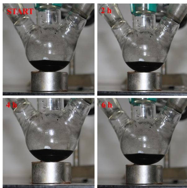
Fig. S13 Pictures of the as prepared RhNi@CeO x /rGO suspensions contact with a ferromagnetic magnet for a period of time.
