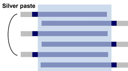
**Fig. S8** Stacked electrochemical capacitors. (a) Single stack, (b) double stack, and (c) triple stack.
