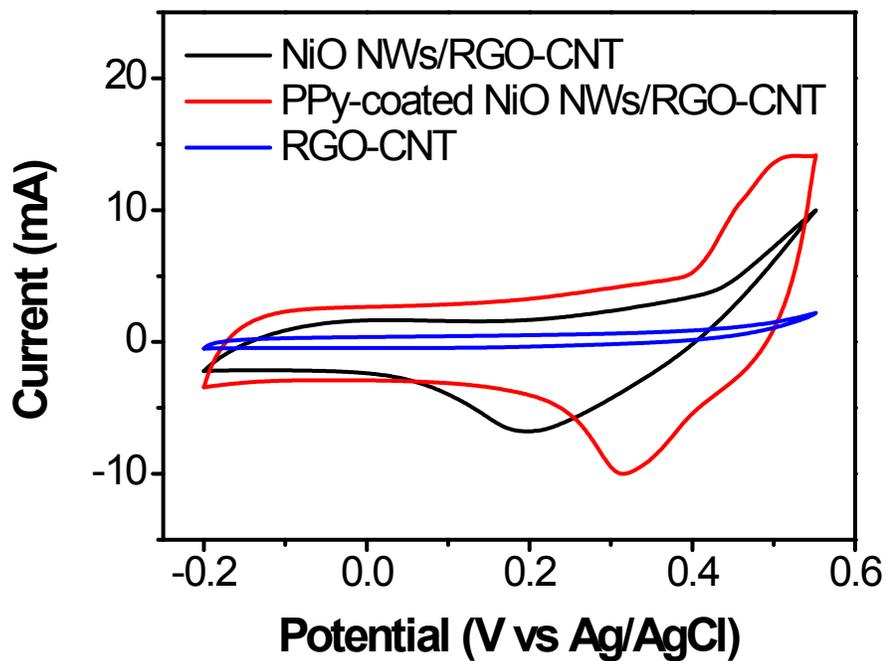
**Fig. S3** CV curves of RGO-CNT, and NiO and PPy-coated NiO nanowalls electrodes obtained at a scan rate of  $20 \text{ mV s}^{-1}$  (CV curves of NiO and PPy-coated NiO nanowalls electrodes are shown in Fig. 4a).
