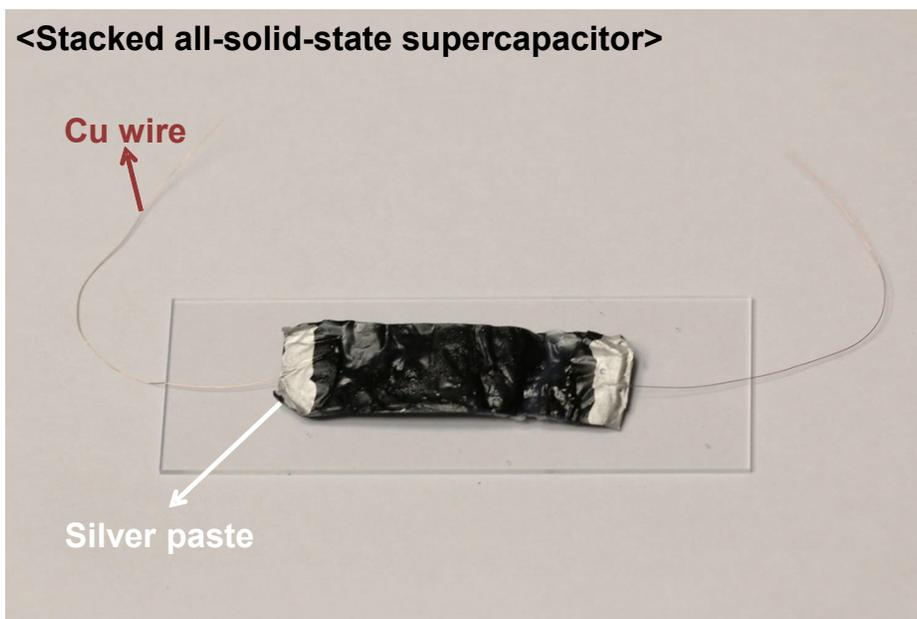
**Fig. S10** Photo images of (a) each electrodes and (b) triple stacked all-solid-state capacitor
