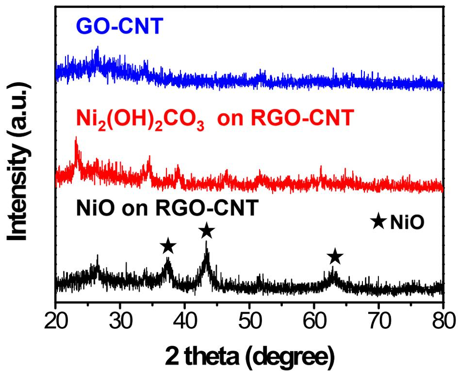
**Fig. S1** XRD patterns of GO-CNT, Ni<sub>2</sub>(OH)<sub>2</sub>CO<sub>3</sub> nullaginite nanowalls on RGO-CNT, and NiO nanowalls on RGO-CNT.
