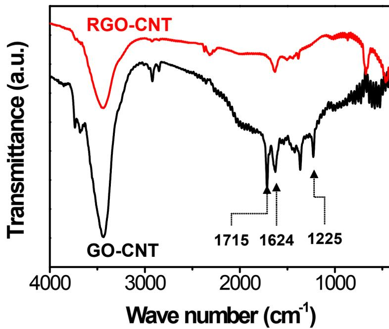
**Fig. S2** FT-IR spectra of GO-CNT and RGO-CNT.
