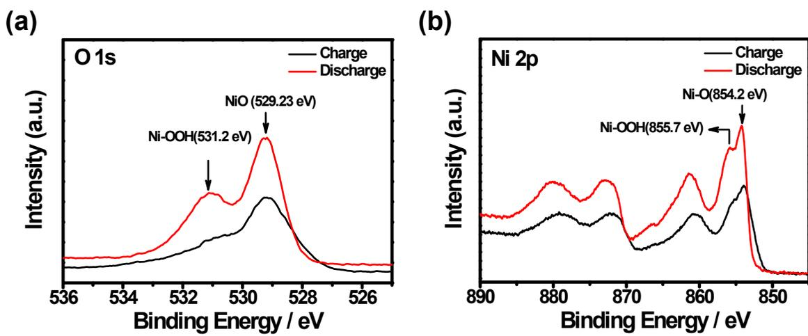
Fig. S6 (a) O 1s XPS spectrum and (b) Ni 2p XPS spectrum of Ppy-coated NiO NWs on RGO-CNT electrode after discharging and charging
