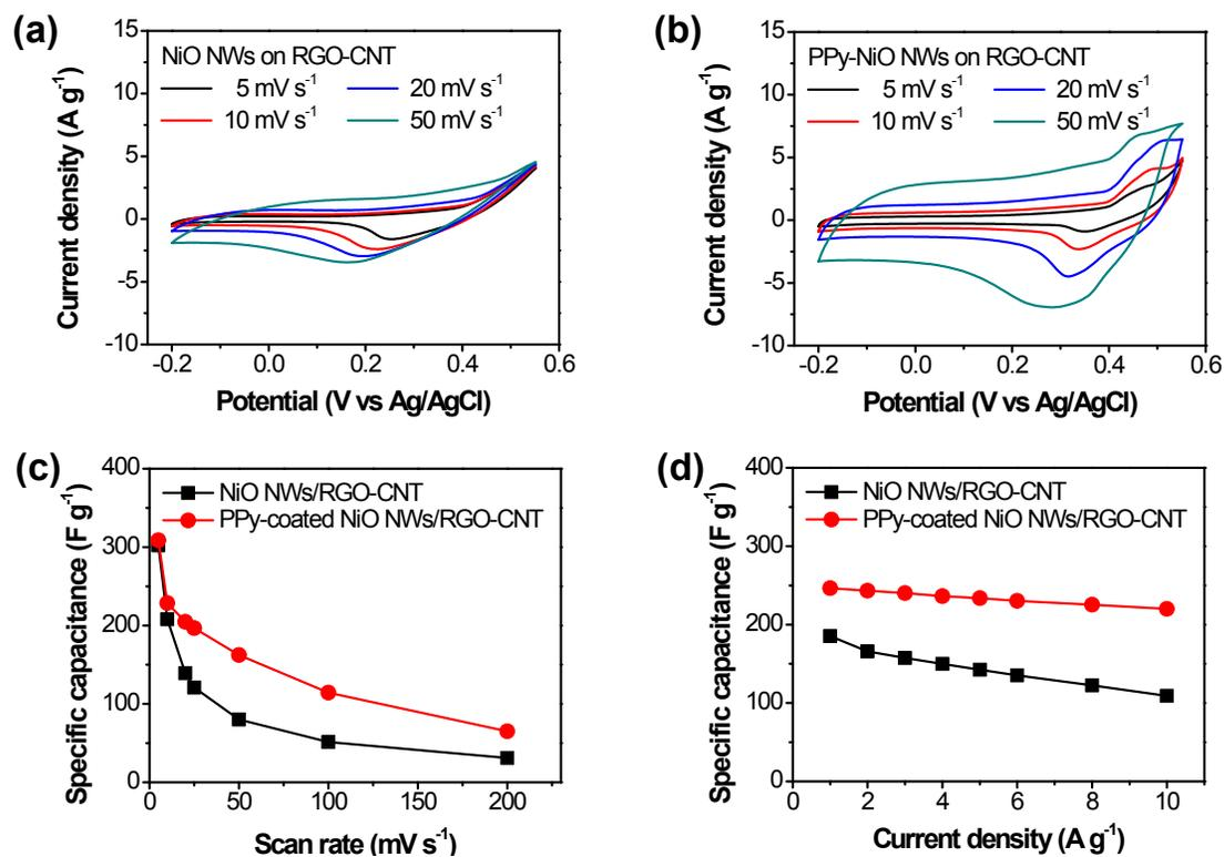
**Fig. S7** CV curves of (a) NiO and (b) PPy-coated NiO nanowalls electrodes obtained at different scan rates. Specific capacitance of NiO and PPy-coated NiO nanowalls electrodes obtained at different (c) scan rates and (d) current densities.
