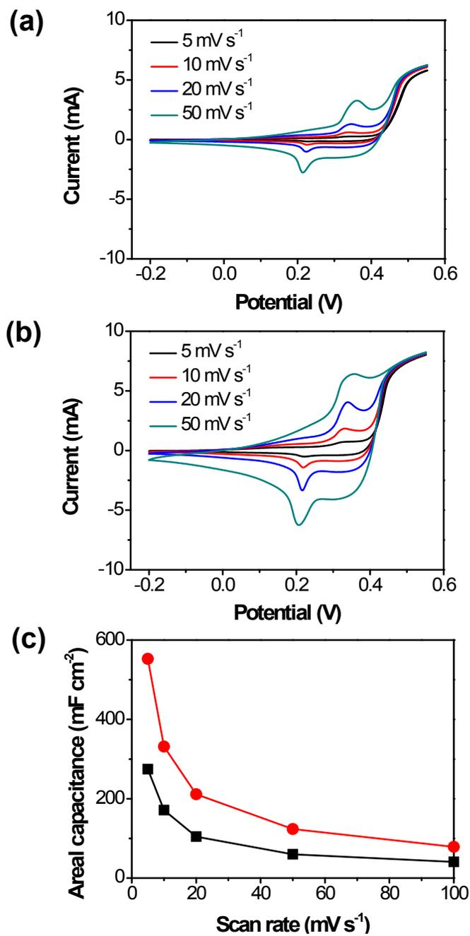
**Fig. S9** (a) CV curves of single-sided and (b) double-sided NiO nanowalls on stainless steel substrate. (c) Areal capacitance of both electrodes with increasing scan rate.
