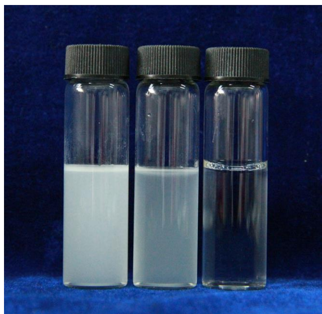
Fig. S5 Tween 20-stabilized diesel-in-water emulsion separation processes of two layers of MCE filter membranes (in the middle) and the MCE-supported RGO membrane (in the right).
