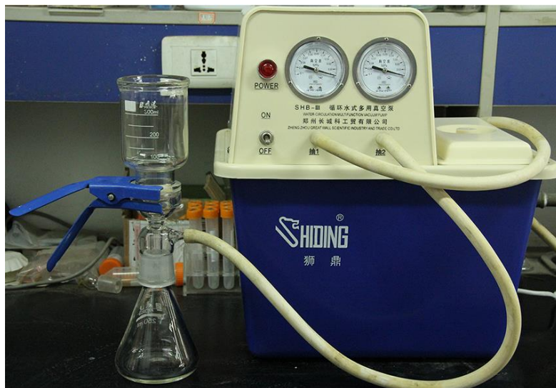
Fig. S3 The vacuum driven filtration system used in this work.
