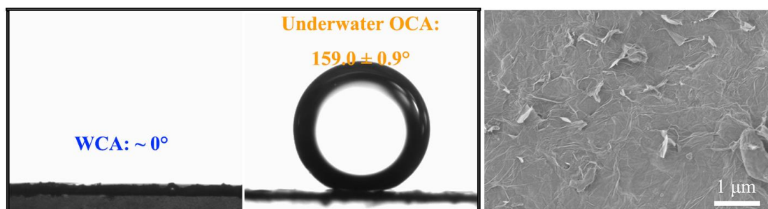
Fig. S9 Wetting behavior toward water in air and 1, 2-dichloroethane under water as well as microstructure of the RGO membrane after cycles of emulsion separation tests.
