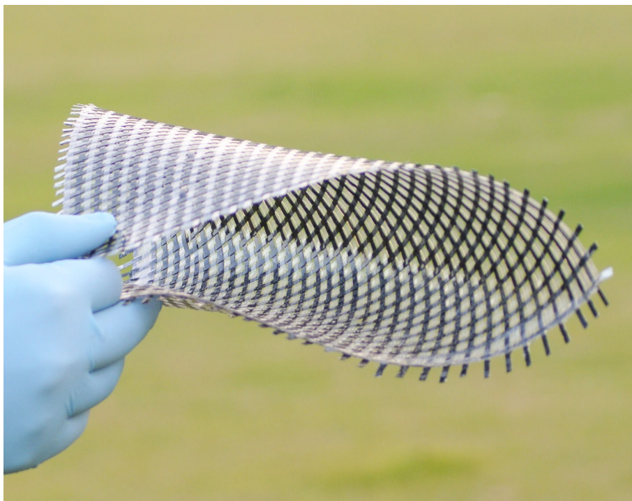
Fig. S17 Photograph of a bent energy storage fabric woven from strip-shaped supercapacitors with a length of 25 cm.
