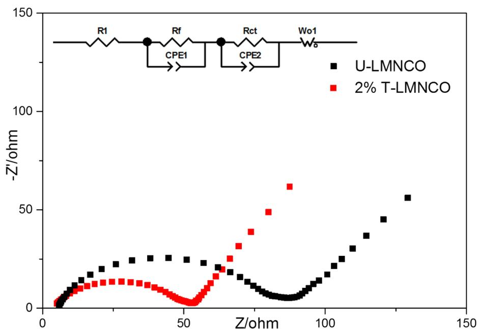
**Fig. S5** EIS spectrum of U-LMNCO and 2% T-LMNCO charged to 4.8 V after first cycle at 0.1 C
