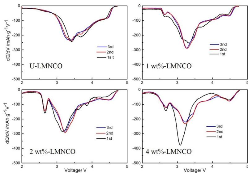
**Fig. S3**  $dQ/dV$  curves of all the samples for three cycles at 0.1 C rate
