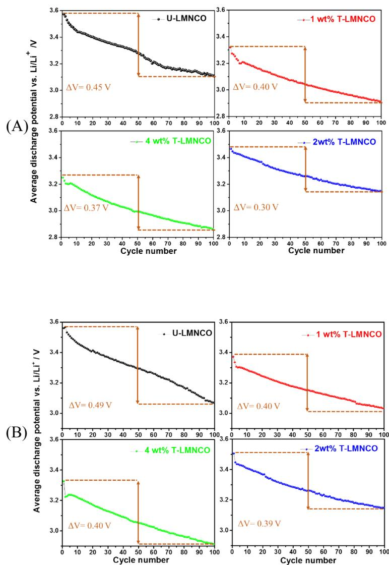
**Fig. S4** Comparison of voltage fading rates of the cells with the synthesized cathode materials during cycling at 0.5 C (A) and 1 C rate (B).
