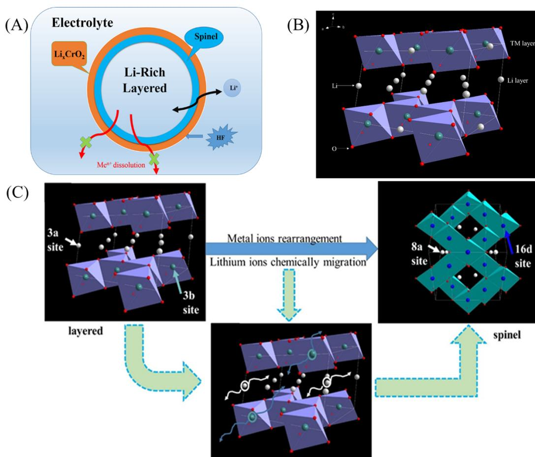
Fig. S2 Schematic view of the Layered@Spinel@Coating layer heterostructure (A); schematic
