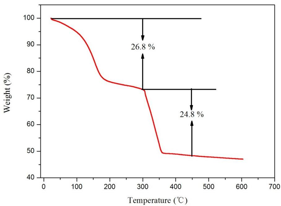
**Figure S6.** TGA curve of  $\text{Fe}_3[\text{Co}(\text{CN})_6]_2 \cdot \text{nH}_2\text{O}$  precursor nanocubes in air flow with a ramp of  $10^{\circ}\text{C min}^{-1}$ .
