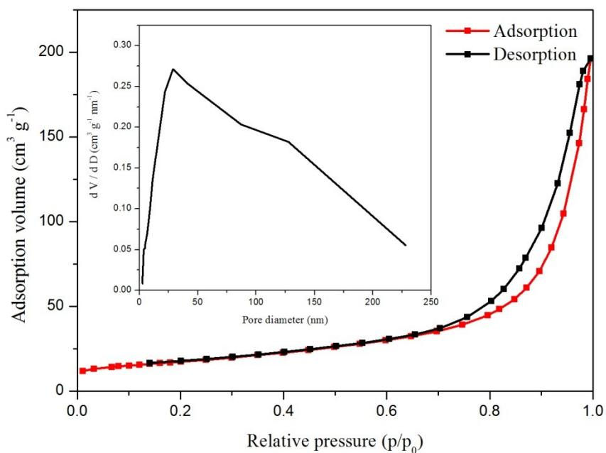
**Figure S10.**  $N_2$  adsorption/desorption isotherm (77 K) curves for the  $\text{Mn}_x\text{Co}_{3-x}\text{O}_4$  nanocages. Inset: The pore-size distribution of the  $\text{Mn}_x\text{Co}_{3-x}\text{O}_4$  nanocages.
