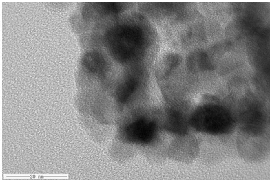
**Figure S20.** HRTEM images of  $\text{Co}_3\text{O}_4$  porous nanocages after photocatalytic water oxidation.
