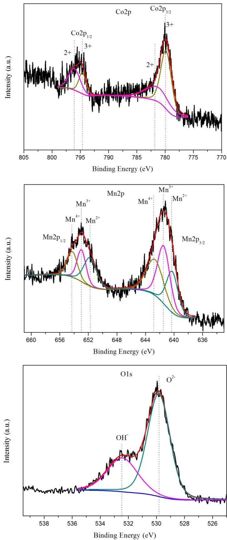
**Figure S13.** Co 2p (top), Mn 2p (middle) and O 1s (bottom) XPS spectra of  $\text{Mn}_x\text{Co}_{3-x}\text{O}_4$  nanocages.
