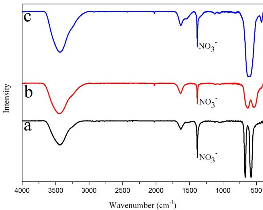
**Figure S7.** FTIR spectra of  $\text{Co}_3\text{O}_4$  (a),  $\text{Mn}_x\text{Co}_{3-x}\text{O}_4$  (b) and  $\text{Fe}_x\text{Co}_{3-x}\text{O}_4$  (c) nanocubes.
