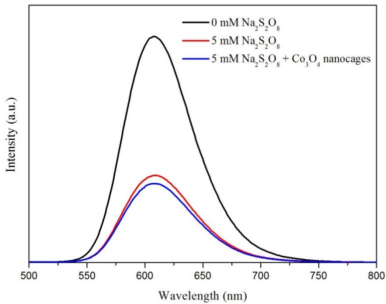
**Figure S15.** Steady-state luminescence spectra ( $\lambda_{\text{ex}} = 450 \text{ nm}$ ) of 1 mM  $[\text{Ru}(\text{bpy})_3]\text{Cl}_2$  in 100 mM phosphate buffer (pH 7.0) containing 5.0 mM persulfate or 0.2 g L<sup>-1</sup> catalyst.
