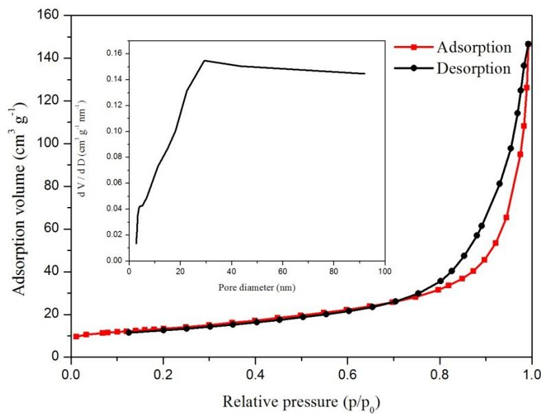
**Figure S9.**  $N_2$  adsorption/desorption isotherm (77 K) curves for  $\text{Co}_3\text{O}_4$  porous nanocages. Inset: The pore-size distribution of the  $\text{Co}_3\text{O}_4$  nanocages.
