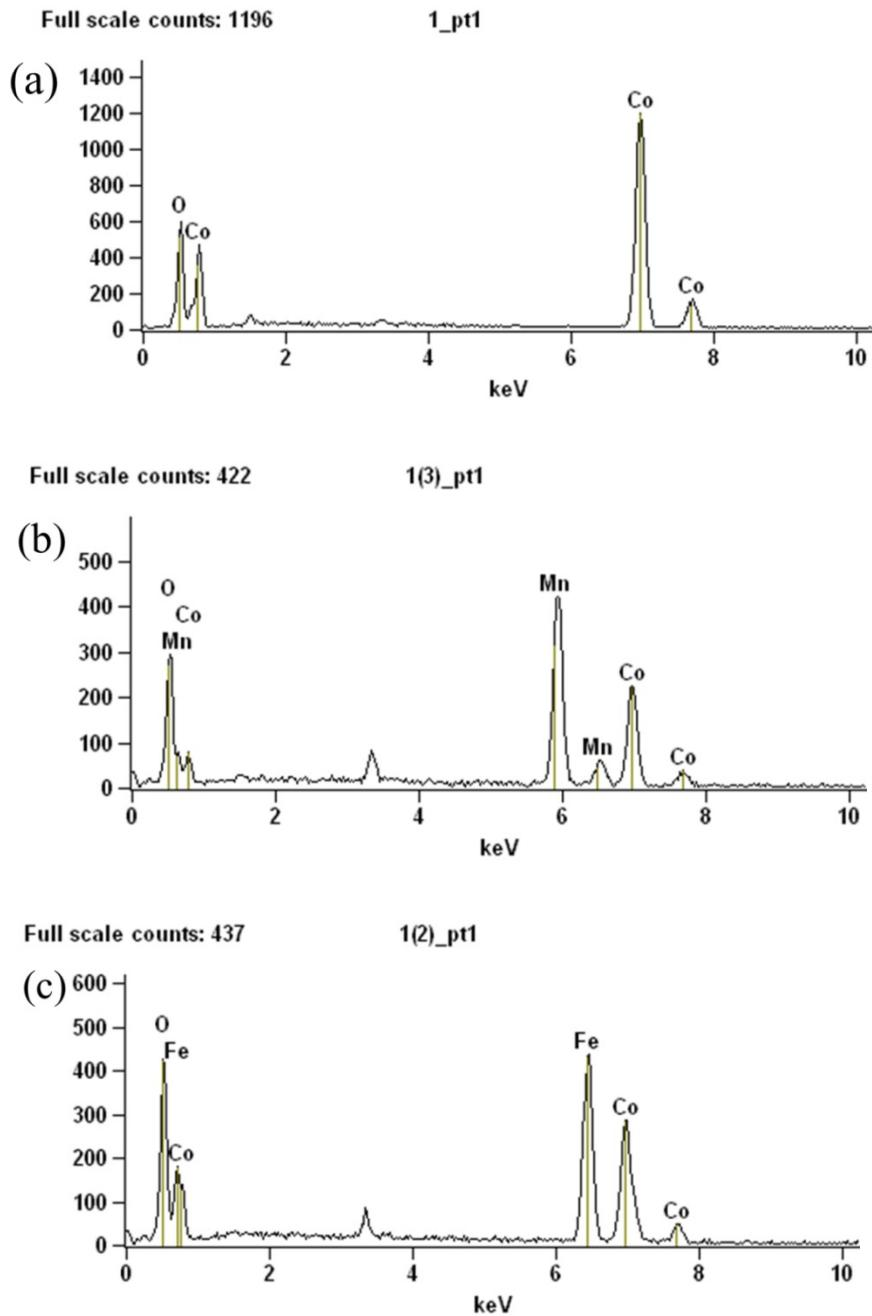
**Figure S12.** EDX measurements of Co, Mn and Fe in (a)  $\text{Co}_3\text{O}_4$ , (b)  $\text{Mn}_x\text{Co}_{3-x}\text{O}_4$  and (c)  $\text{Fe}_x\text{Co}_{3-x}\text{O}_4$ .
