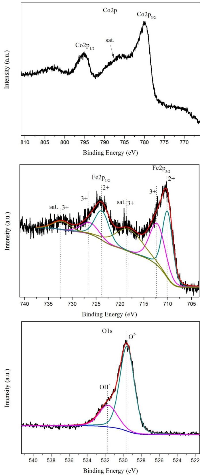
**Figure S14.** Co 2p (top), Fe 2p (middle) and O 1s (bottom) XPS spectra of  $\text{Fe}_x\text{Co}_{3-x}\text{O}_4$  nanocages.
