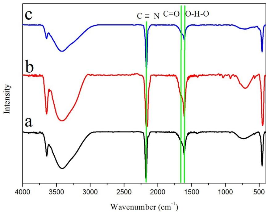
**Figure S3.** FTIR spectra of  $\text{Co}_3[\text{Co}(\text{CN})_6]_2$ ,  $\text{Mn}_3[\text{Co}(\text{CN})_6]_2$  and  $\text{Fe}_3[\text{Co}(\text{CN})_6]_2$  precursor nanocubes.
