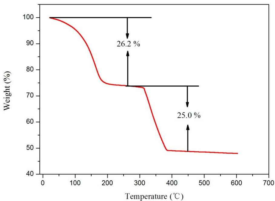
**Figure S5.** TGA curve of  $\text{Mn}_3[\text{Co}(\text{CN})_6]_2 \cdot n\text{H}_2\text{O}$  precursor nanocubes in air flow with a ramp of  $10^{\circ}\text{C min}^{-1}$ .
