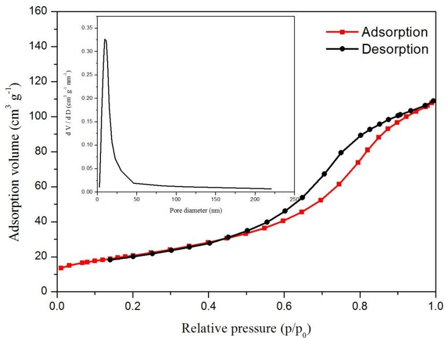
**Figure S11.**  $N_2$  adsorption/desorption isotherm (77 K) curves for the  $Fe_xCo_{3-x}O_4$  nanocages. Inset: The pore-size distribution of the  $Fe_xCo_{3-x}O_4$  nanocages.
