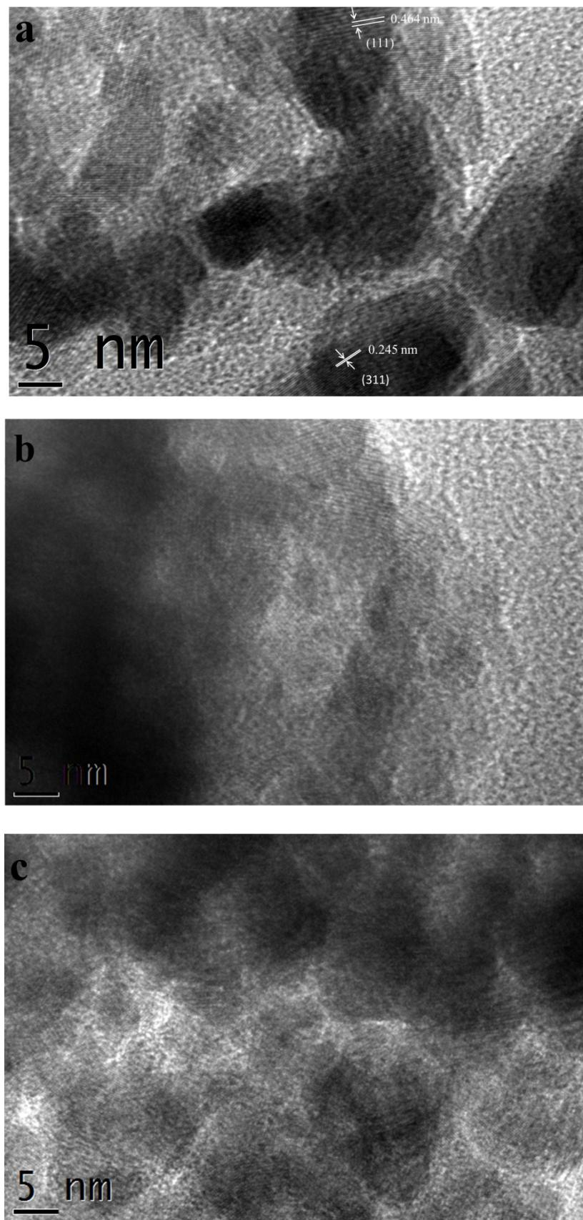
**Figure S8.** HRTEM images for as-prepared (a)  $\text{Co}_3\text{O}_4$  nanocages, (b)  $\text{Mn}_x\text{Co}_{3-x}\text{O}_4$  nanocages and (c)  $\text{Fe}_x\text{Co}_{3-x}\text{O}_4$  nanocages.
