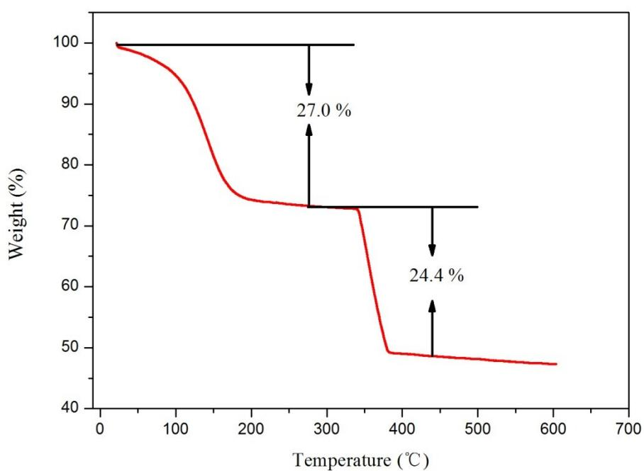
**Figure S4.** TGA curve of  $\text{Co}_3[\text{Co}(\text{CN})_6]_2 \cdot n\text{H}_2\text{O}$  precursor nanocubes in air flow with a ramp of  $10^{\circ}\text{C min}^{-1}$ .
