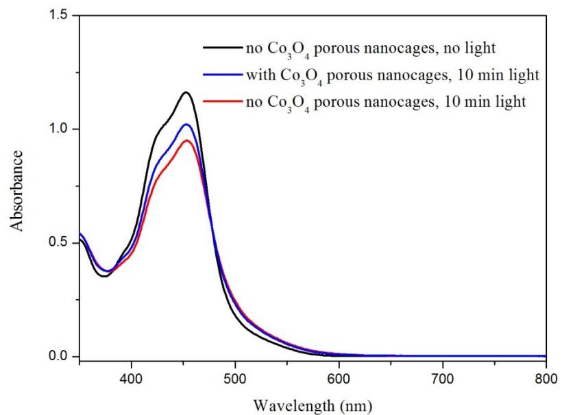
**Figure S16.** UV-vis spectral changes during the photocatalytic  $\text{O}_2$  evolution with or without catalyst. (absorption of  $[\text{Ru}(\text{bpy})_3]\text{Cl}_2$  at 450 nm).
