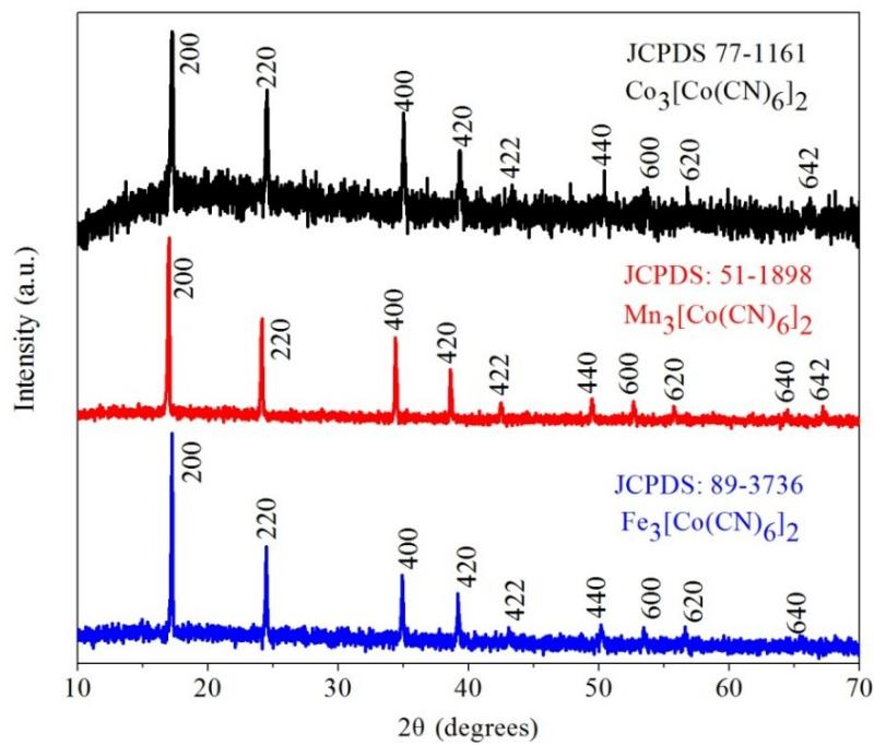
**Figure S2.** PXRD patterns of  $\text{Co}_3[\text{Co}(\text{CN})_6]_2$ ,  $\text{Mn}_3[\text{Co}(\text{CN})_6]_2$  and  $\text{Fe}_3[\text{Co}(\text{CN})_6]_2$  precursor nanocubes.
