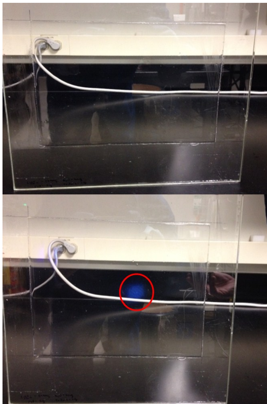
Figure S17. (top) PVA film with \text{Li}_2\text{B}_{12}\text{H}_{12} , (bottom) PVA with \text{Li}_2\text{B}_{12}\text{H}_{12} exposed to the UV-LED projection source in normal room light. Red circle highlights the projected image.
