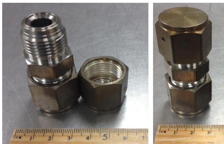
Figure S1. Reactor used for the thermochemical synthesis of \text{Li}_2\text{B}_{12}\text{H}_{12} .
