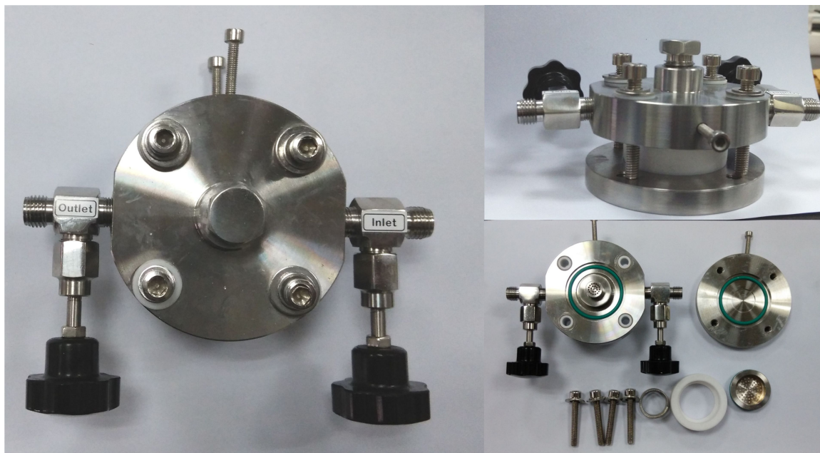
Fig. S10 Picture of a cell for the DEMS analysis. The DEMS system was built in-house and guided by the requirement to detect the gases evolved during the charge. A quadrupole mass spectrometer (NETZSCH QMS 403 C) with leak inlet is connected to a customized Swagelok cell assembly ( Fig. S10 ). The cathode current collector is integrated with two tubes as purge gas inlet and outlet ( Fig. S10 ). Each tested cell was discharged with a fixed capacitance of 500 \text{ mAh g}^{-1} in the sealed assembly, and then online gas analysis was performed during the recharge process with a purge Ar stream at a current density of 0.25 \text{ mA cm}^{-2} . Before the charge test and online gas analysis, the system was purged with pure Ar stream for 12 hours, and the background for \text{O}_2 and \text{CO}_2 was calibrated. Purge gas flows were typically 10 \text{ mL/min} .
